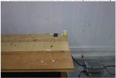
1.2 Radiated Emissions (9kHz-30MHz) Test Setup
