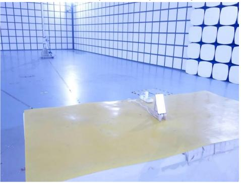
1.4 Emission Mask Test Setup
