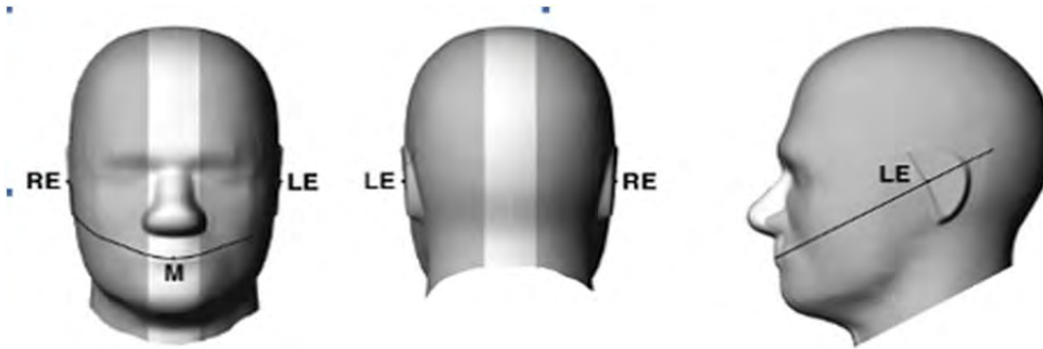
F-3. Front, back, and side views of SAM (model for the phantom shell). Full-head model is for illustration purposes only-procedures in this recommended practice are intended primarily for the phantom setup.
