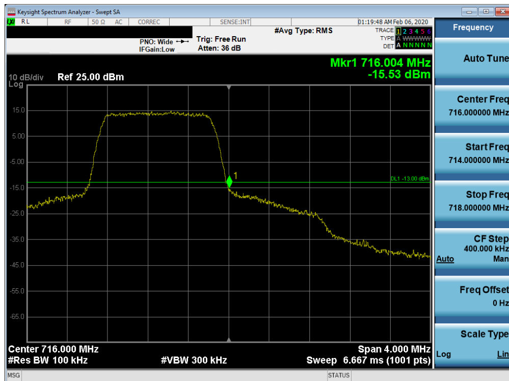
Plot 7-109. Upper Band Edge Plot (Band 12 - 1.4MHz QPSK - Full RB Configuration)
