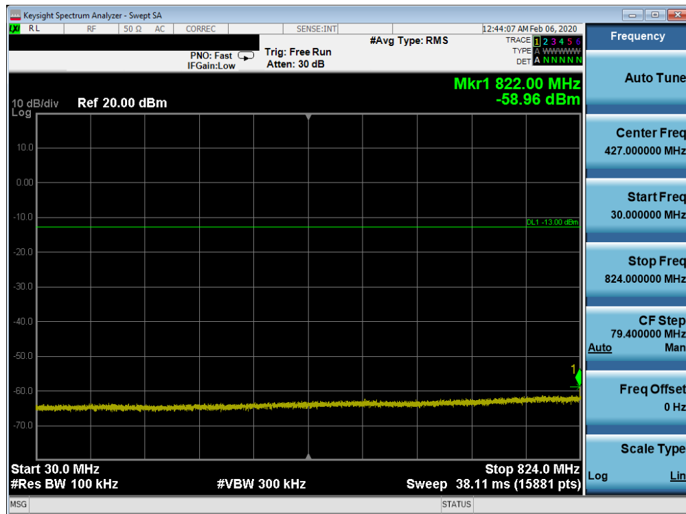
Plot 7-75. Conducted Spurious Plot (Band 5 - 10.0MHz QPSK - RB Size 1, RB Offset 0 - High Channel)
