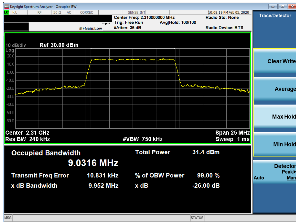
Plot 7-47. Occupied Bandwidth Plot (Band 30 - 10.0MHz QPSK - Full RB Configuration)
