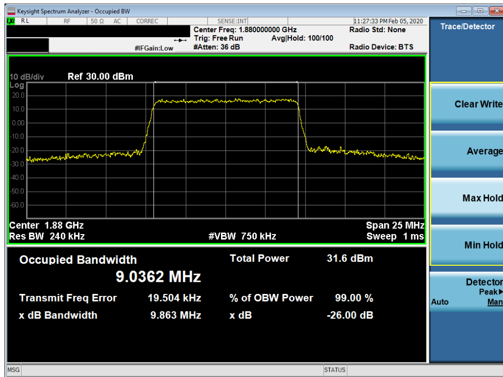
Plot 7-39. Occupied Bandwidth Plot (Band 2 - 10.0MHz QPSK - Full RB Configuration)
