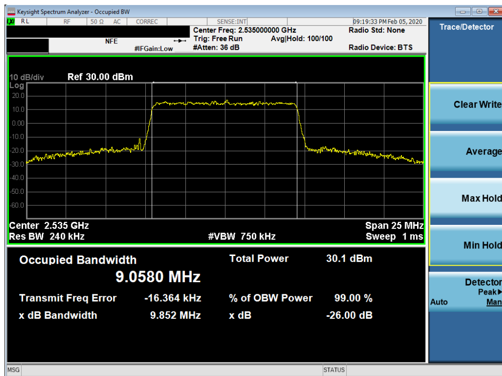
Plot 7-52. Occupied Bandwidth Plot (Band 7 - 10.0MHz 16-QAM - Full RB Configuration)
