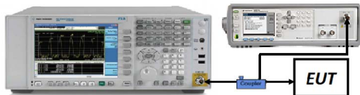
Figure 7-3. Test Instrument & Measurement Setup
