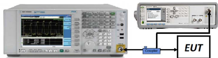
Figure 7-4. Test Instrument & Measurement Setup
