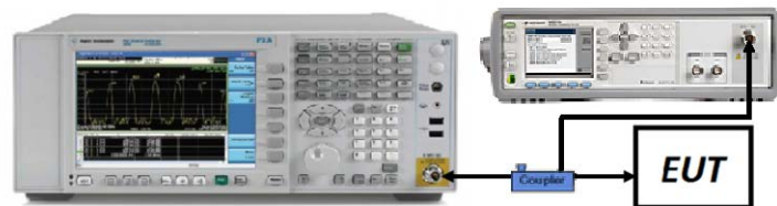
Figure 7-1. Test Instrument & Measurement Setup
