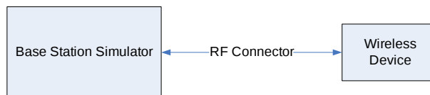
Figure 9-2 Power Measurement Setup
