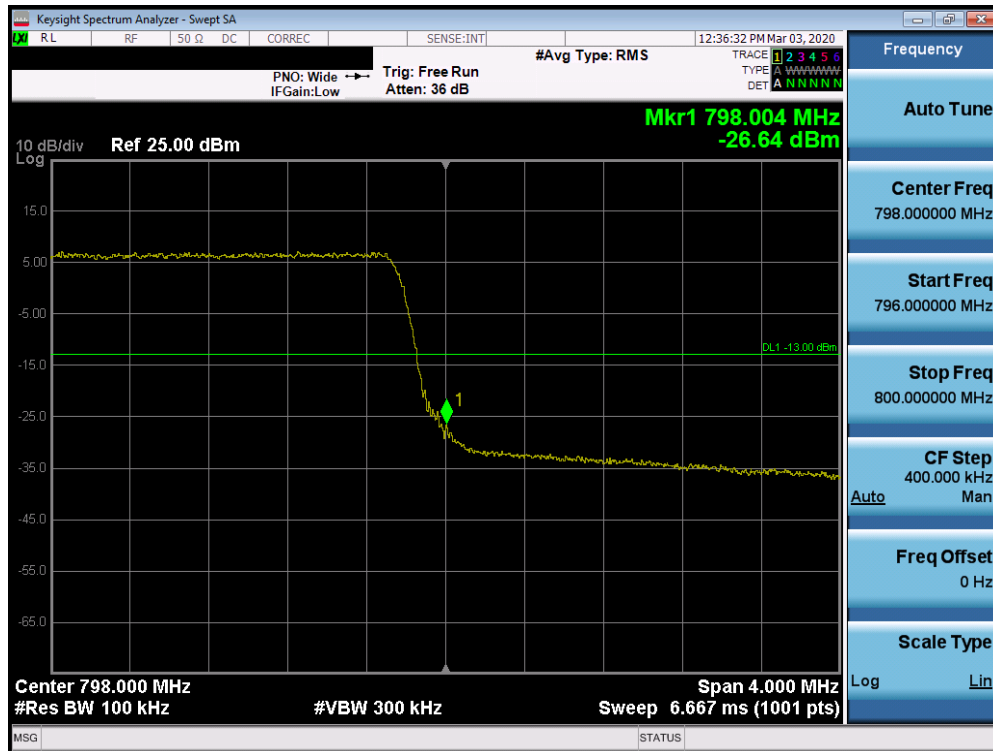
Plot 7-10. Upper Band Edge Plot (Band 14 - 5MHz QPSK – Full RB Configuration)
