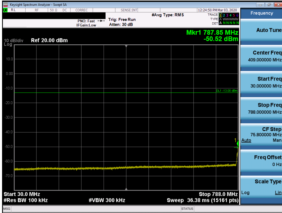
Plot 7-5. Conducted Spurious Plot (LTE Band 14 – 10 MHz QPSK - RB Size 1, RB Offset 0 - Mid Channel)
