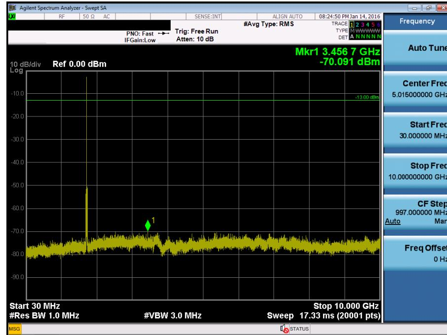
BAND 4. Conducted Spurious Plot\_2 (20175ch\_10MHz\_QPSK\_RB 1\_0)
