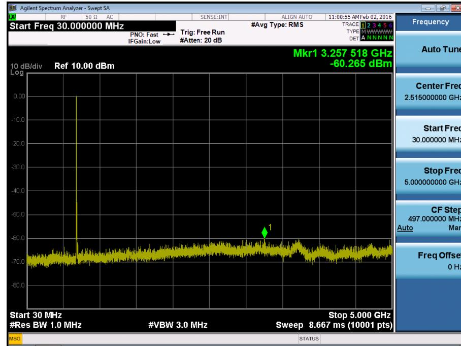
BAND 17. Conducted Spurious Plot\_2 (23790ch\_10MHz\_QPSK\_RB 1\_0)
