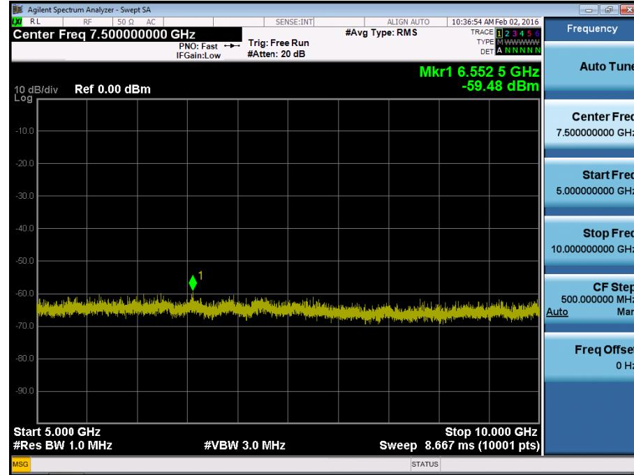
BAND 17. Conducted Spurious Plot\_1 (23790ch\_10MHz\_QPSK\_RB 1\_0)
