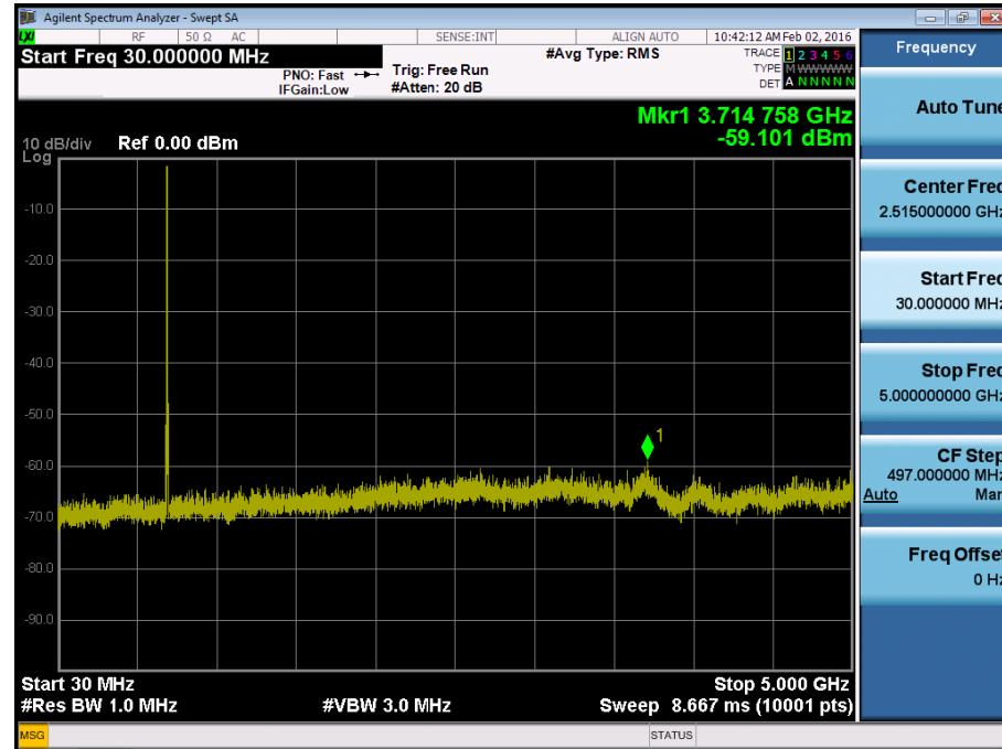
BAND 17. Conducted Spurious Plot\_2 (23825ch\_5MHz\_QPSK\_RB 1\_0)
