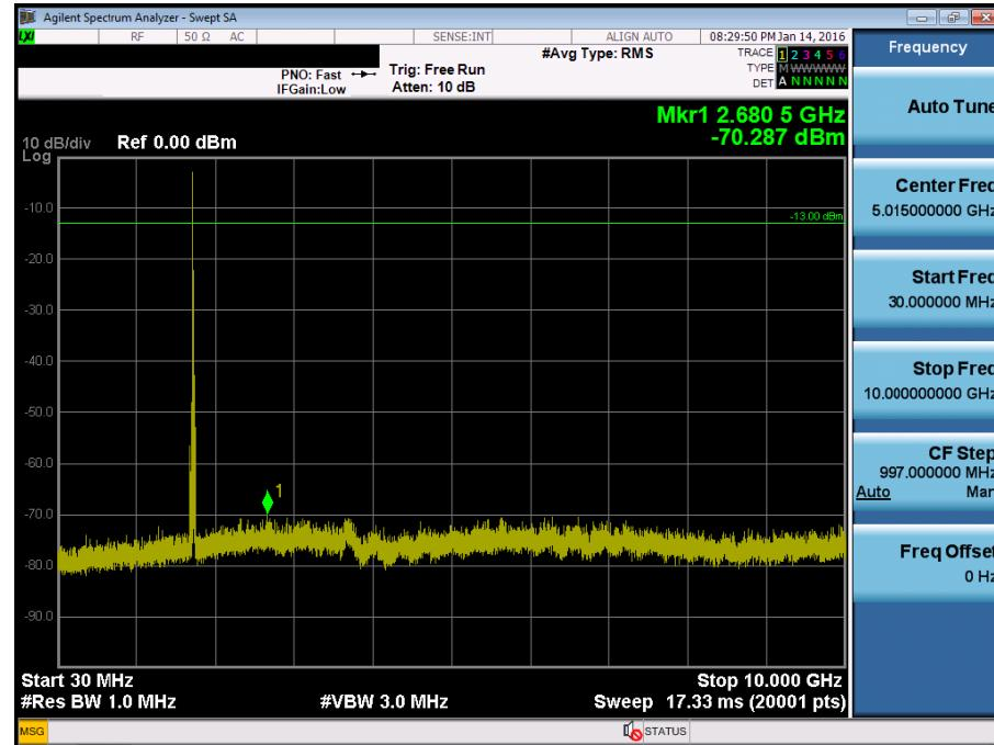
BAND 4. Conducted Spurious Plot\_2 (20300ch\_20MHz\_QPSK\_RB 1\_0)
