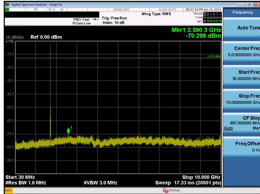
BAND 4. Conducted Spurious Plot\_2 (20175ch\_5MHz\_QPSK\_RB 1\_0)
