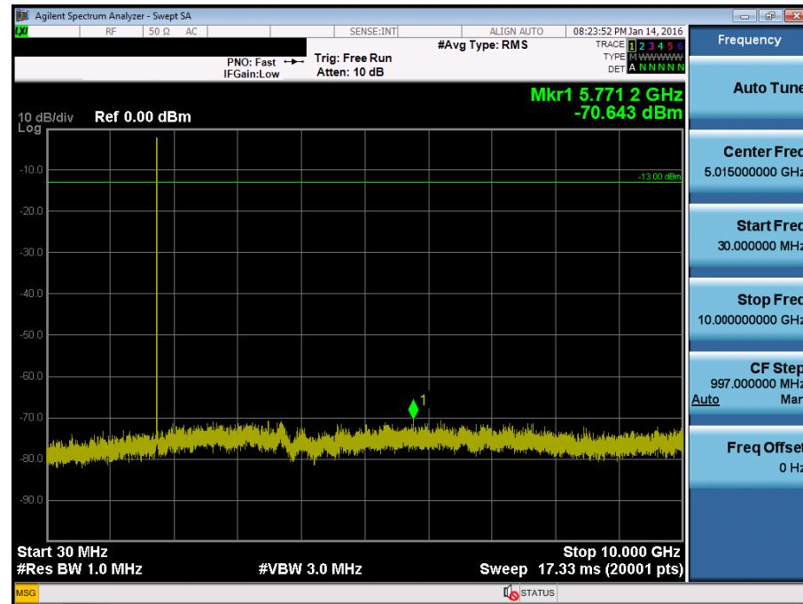
BAND 4. Conducted Spurious Plot\_2 (20375ch\_5MHz\_QPSK\_RB 1\_0)
