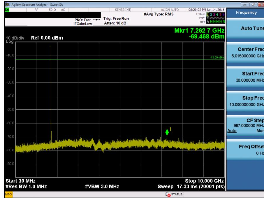
BAND 4. Conducted Spurious Plot\_2 (20175ch\_3MHz\_QPSK\_RB 1\_0)
