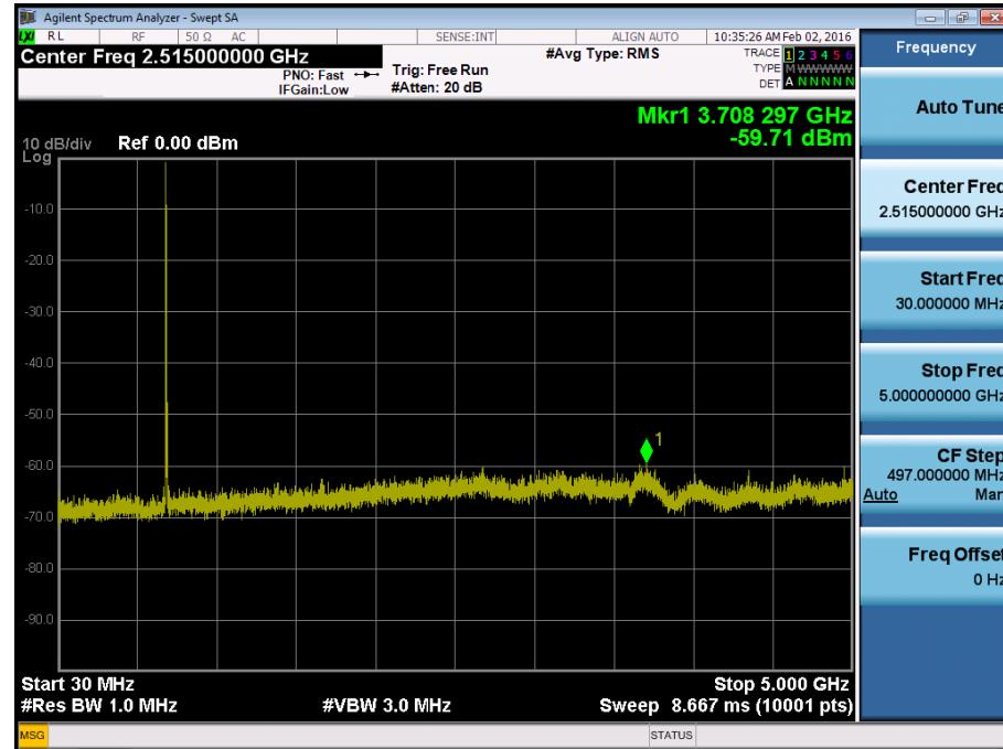
BAND 17. Conducted Spurious Plot\_2 (23755ch\_5MHz\_QPSK\_RB 1\_0)
