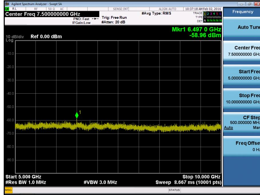
BAND 17. Conducted Spurious Plot\_1 (23800ch\_10MHz\_QPSK\_RB 1\_0)
