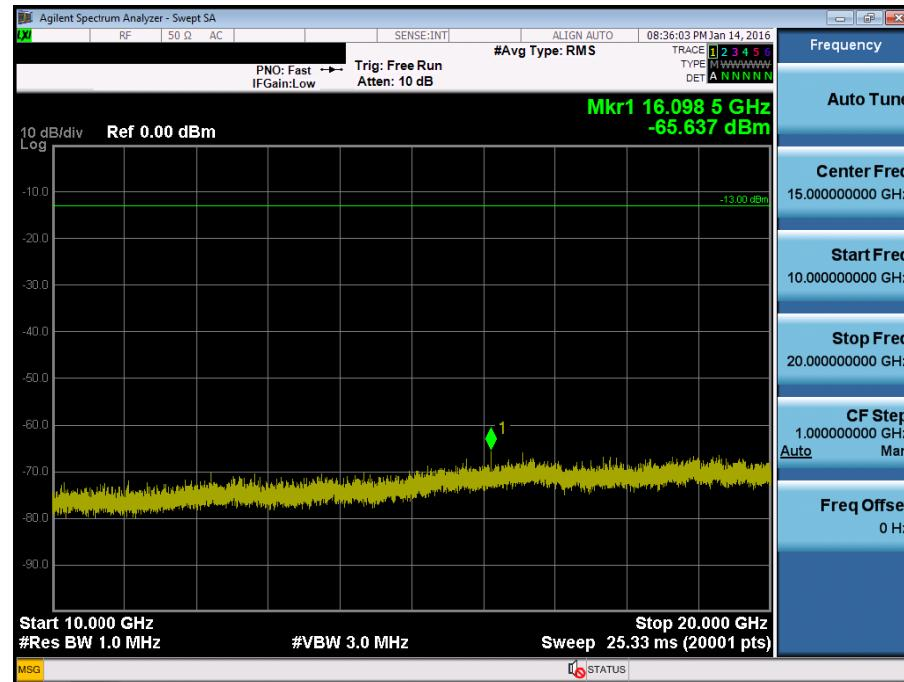
BAND 4. Conducted Spurious Plot\_1 (19965ch\_3MHz\_QPSK\_RB 1\_0)
