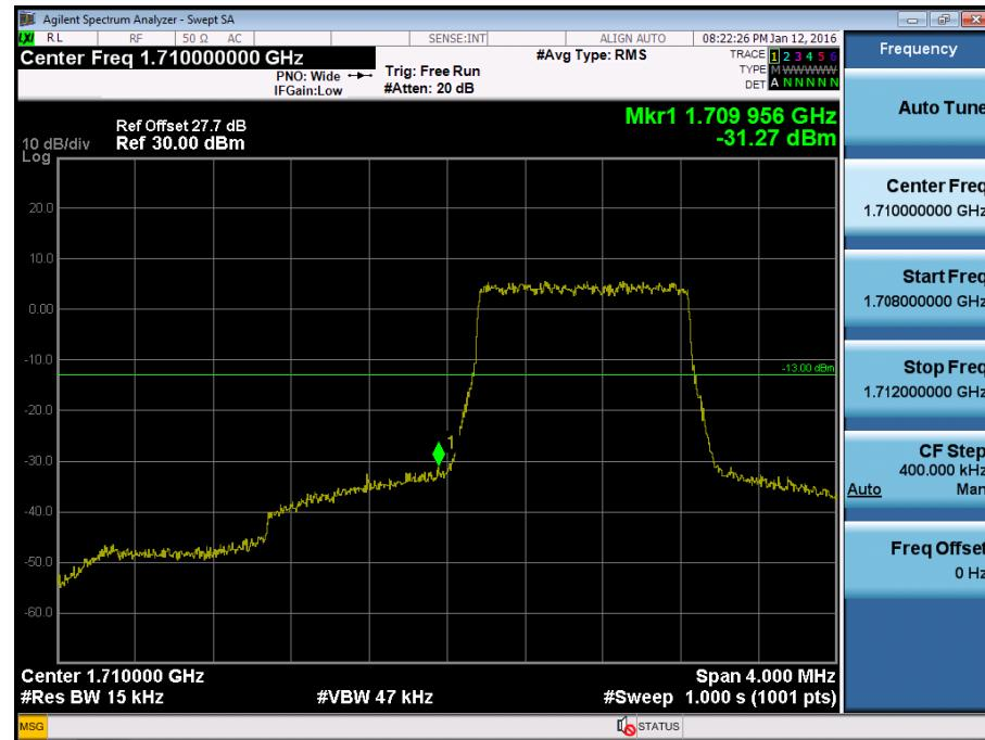
BAND 4. Lower Extended Band Edge Plot (1.4M BW Ch.19957 QPSK\_RB6\_0) -3
