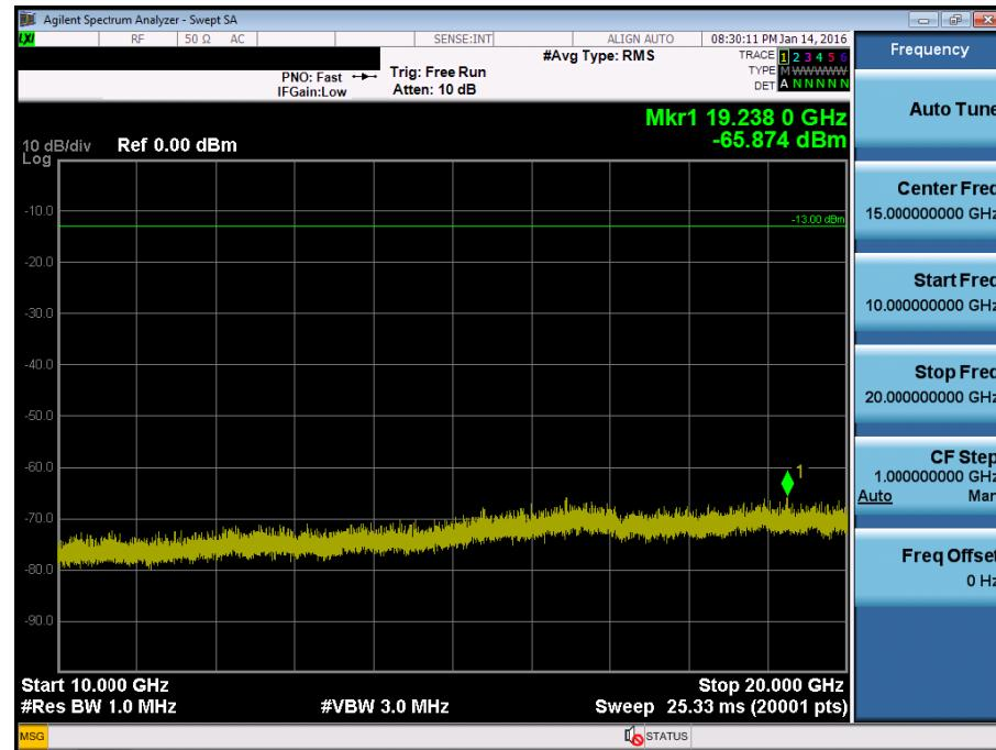
BAND 17. Conducted Spurious Plot\_1 (23755ch\_5MHz\_QPSK\_RB 1\_0)
