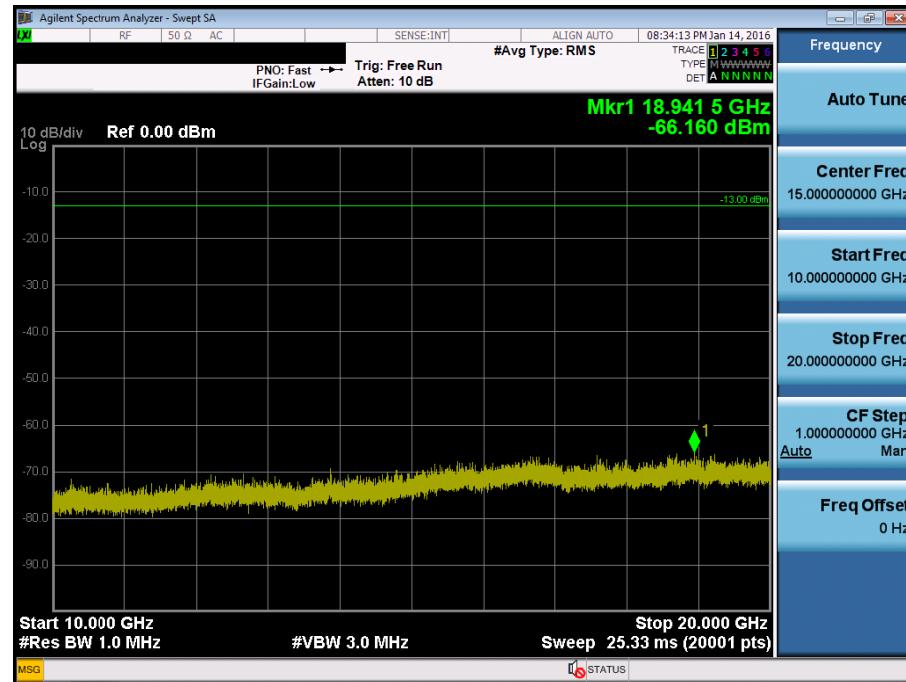
BAND 4. Conducted Spurious Plot\_1 (20175ch\_5MHz\_QPSK\_RB 1\_0)
