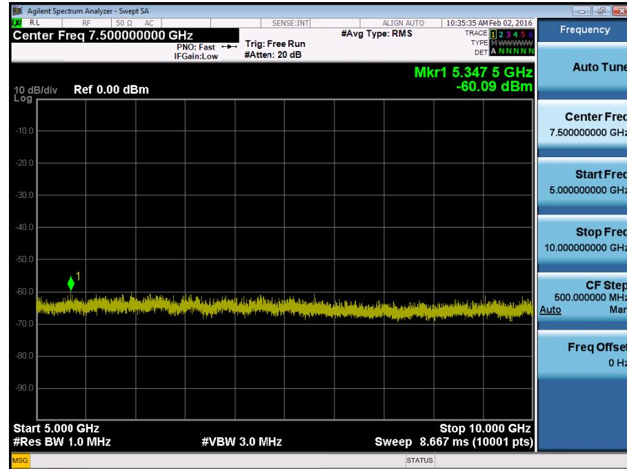
BAND 17. Conducted Spurious Plot\_1 (23790ch\_5MHz\_QPSK\_RB 1\_0)
