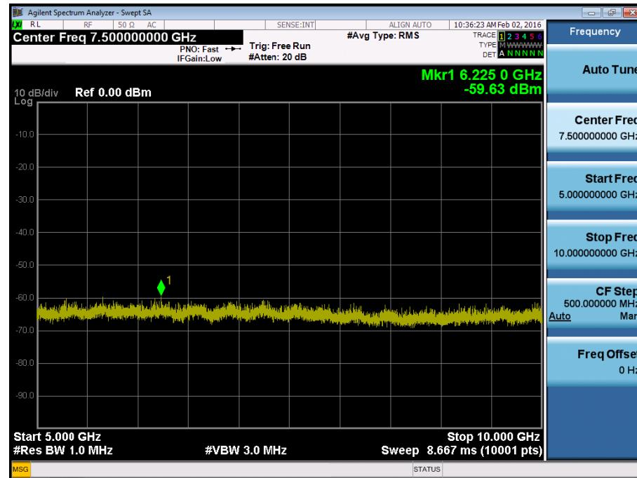
BAND 17. Conducted Spurious Plot\_1 (23780ch\_10MHz\_QPSK\_RB 1\_0)
