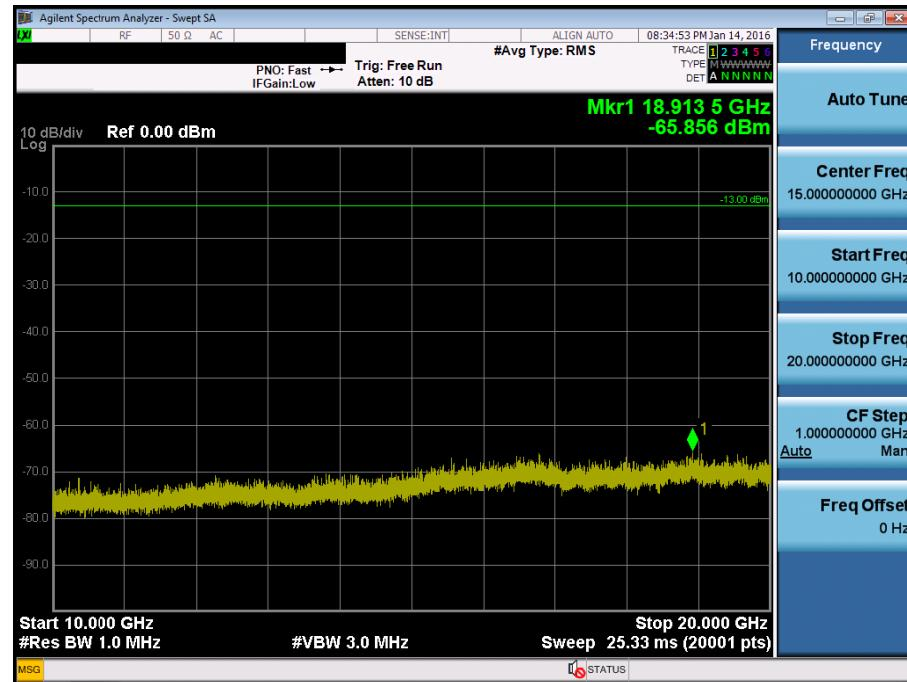
BAND 4. Conducted Spurious Plot\_1 (19975ch\_5MHz\_QPSK\_RB 1\_0)
