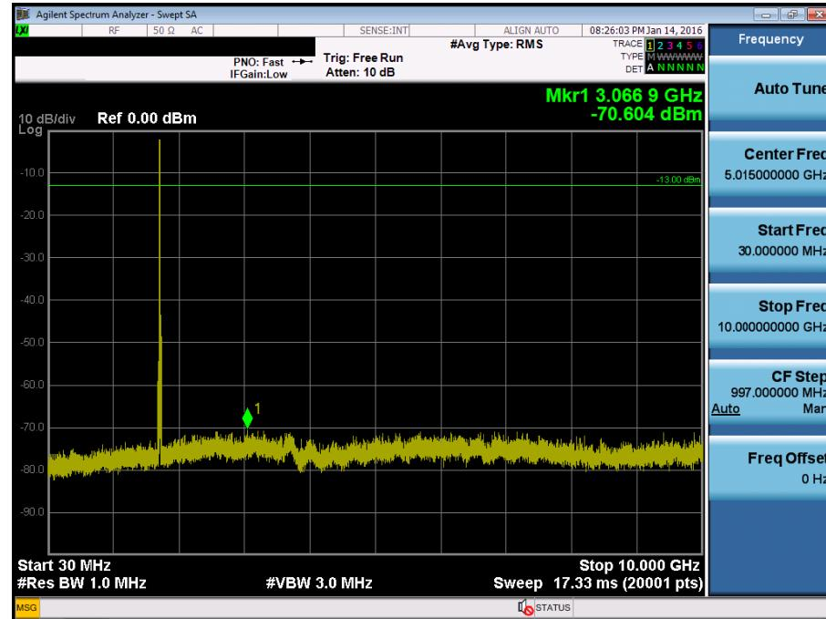
BAND 4. Conducted Spurious Plot\_2 (20175ch\_15MHz\_QPSK\_RB 1\_0)
