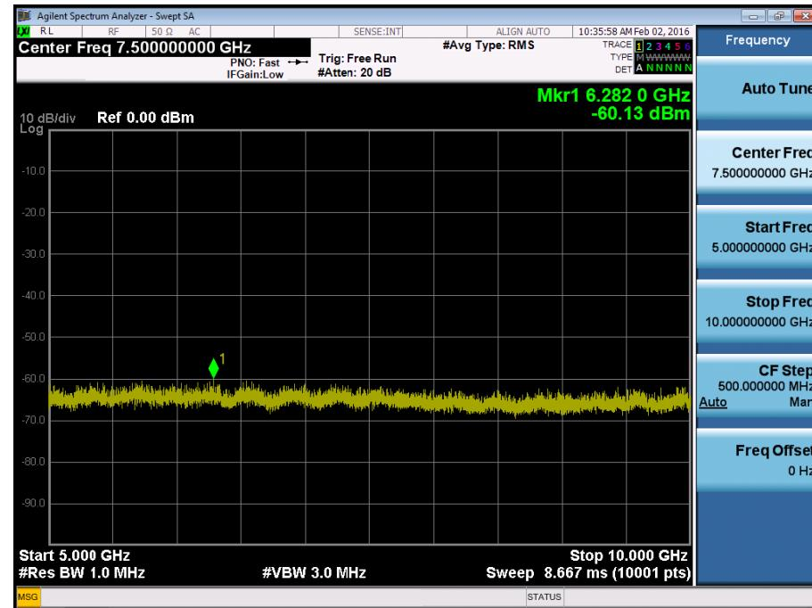
BAND 17. Conducted Spurious Plot\_1 (23825ch\_5MHz\_QPSK\_RB 1\_0)
