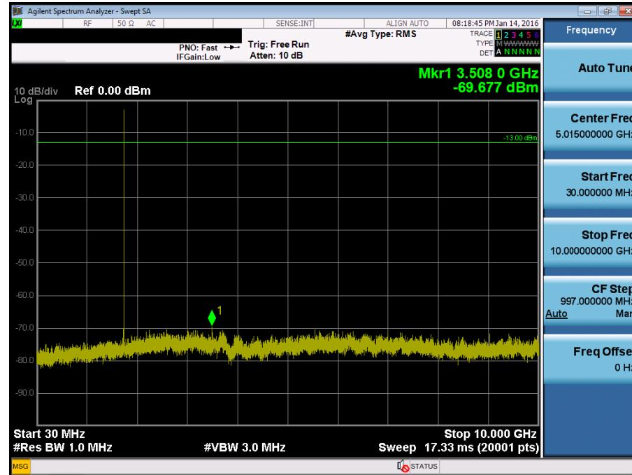
BAND 4. Conducted Spurious Plot\_2 (20393ch\_1.4MHz\_QPSK\_RB 1\_0)
