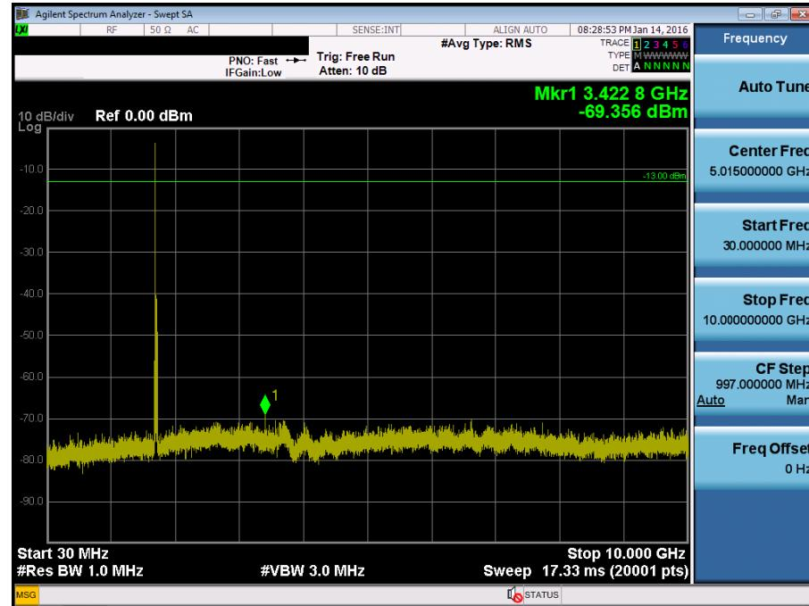
BAND 4. Conducted Spurious Plot\_2 (20050ch\_20MHz\_QPSK\_RB 1\_0)
