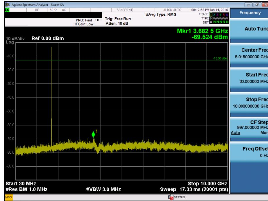
BAND 4. Conducted Spurious Plot\_2 (19957ch\_1.4MHz\_QPSK\_RB 1\_0)
