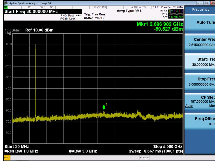
BAND 17. Conducted Spurious Plot\_2 (23780ch\_10MHz\_QPSK\_RB 1\_0)
