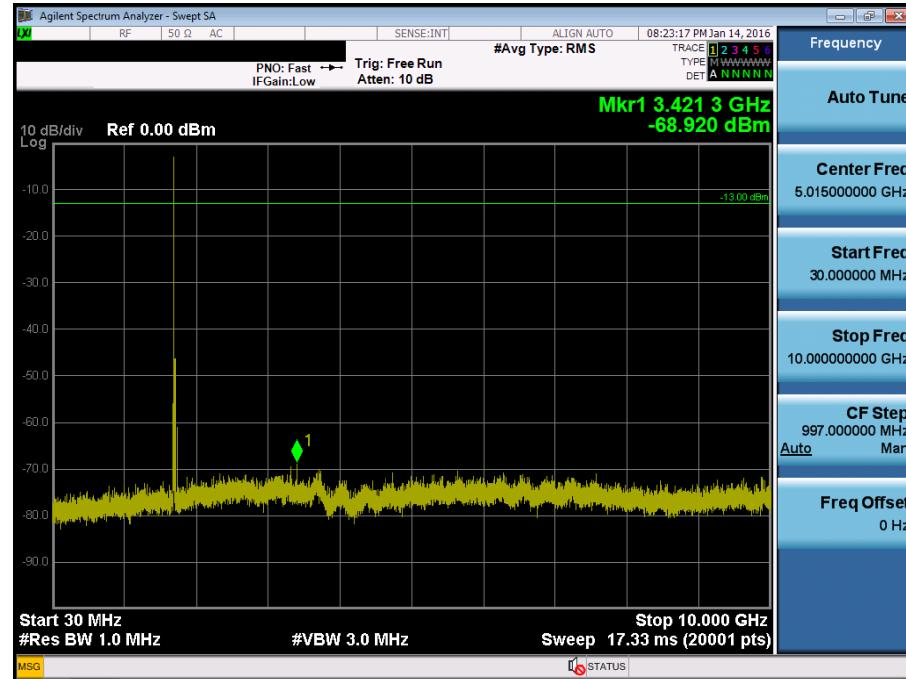
BAND 4. Conducted Spurious Plot\_2 (19975ch\_5MHz\_QPSK\_RB 1\_0)
