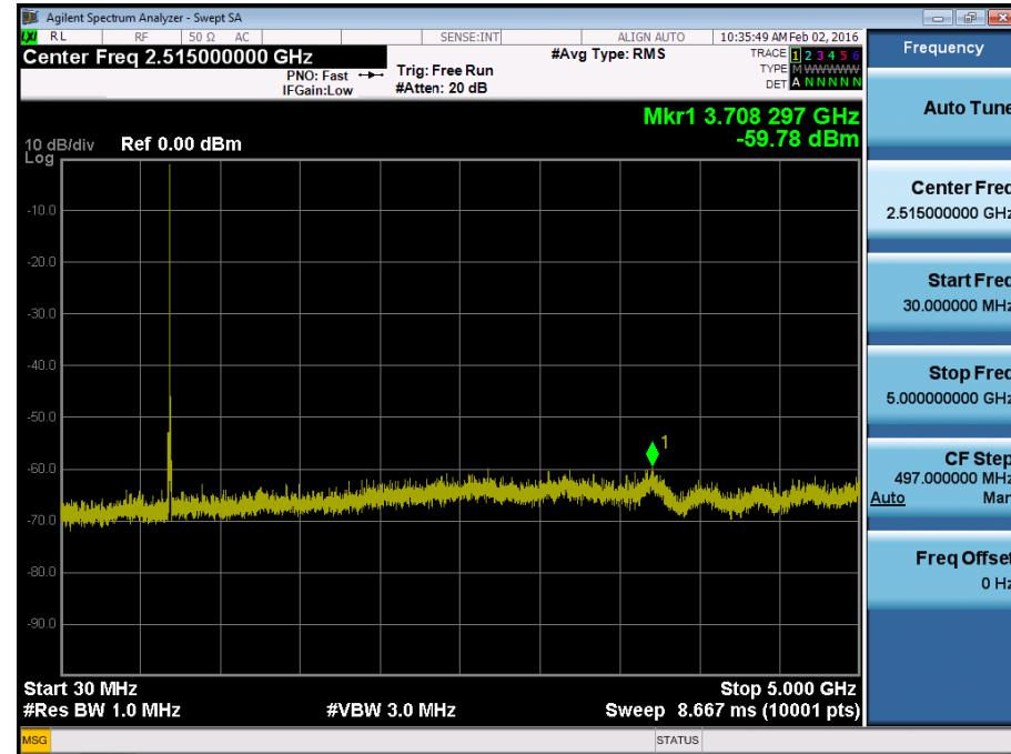
BAND 17. Conducted Spurious Plot\_2 (23790ch\_5MHz\_QPSK\_RB 1\_0)
