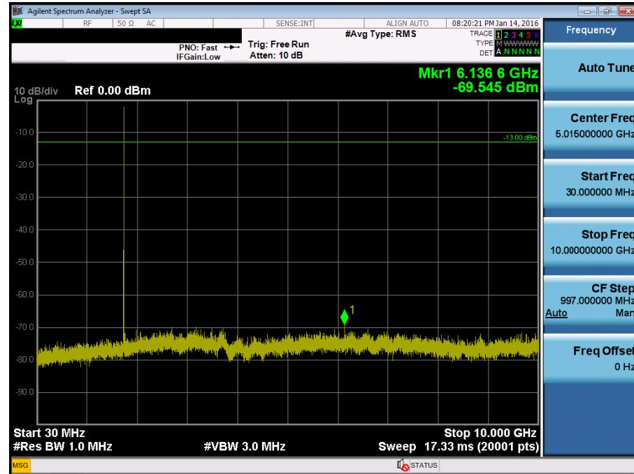
BAND 4. Conducted Spurious Plot\_2 (20385ch\_3MHz\_QPSK\_RB 1\_0)
