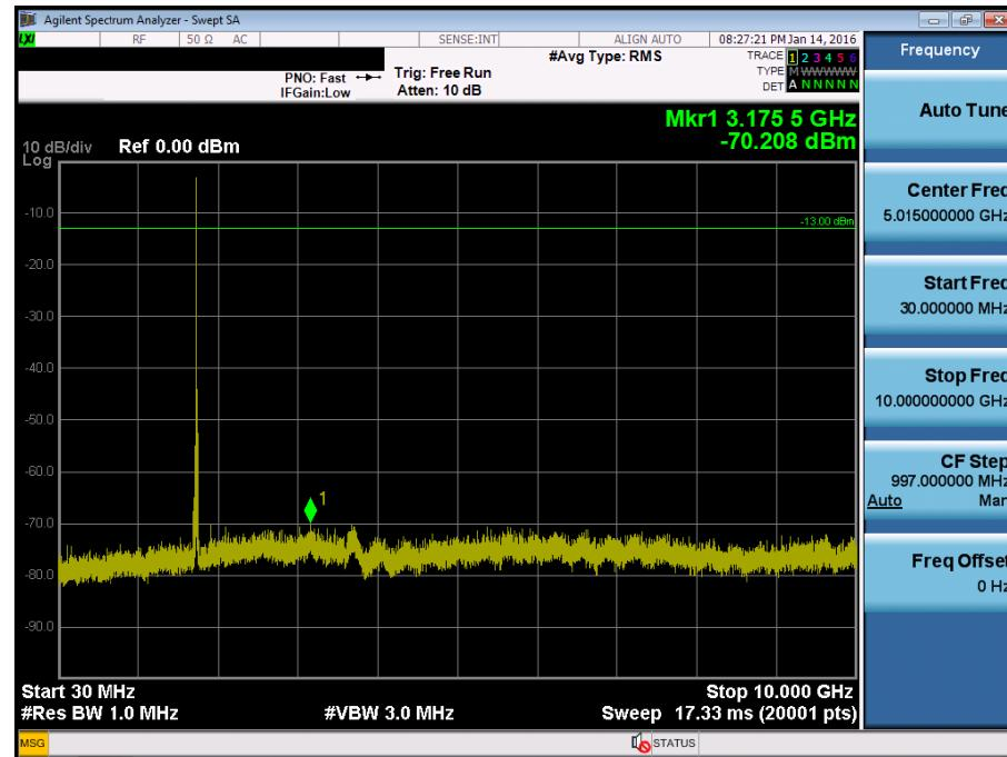
BAND 4. Conducted Spurious Plot\_2 (20325ch\_15MHz\_QPSK\_RB 1\_0)
