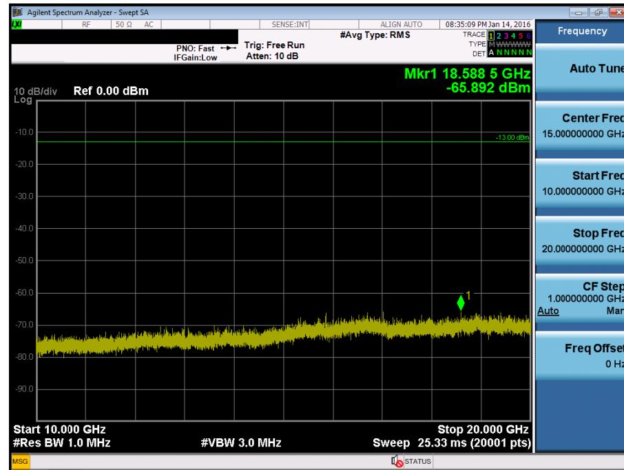
BAND 4. Conducted Spurious Plot\_1 (20385ch\_3MHz\_QPSK\_RB 1\_0)
