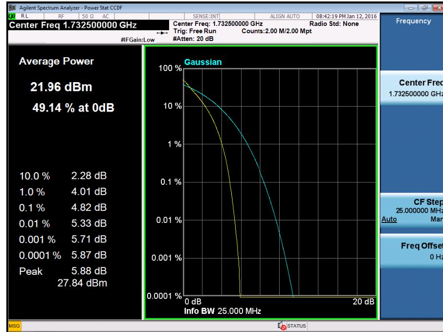
BAND 4. PAR Plot (20M BW\_Ch.20175\_16QAM\_RB100\_0)
