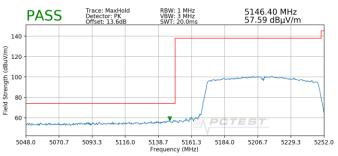
Plot 7-22. Radiated Lower Band Edge Plot SISO ANT1 (Peak – UNII Band 1)
