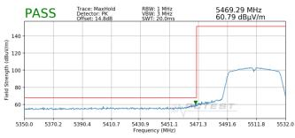
Plot 7-19. Radiated Lower Band Edge Plot SISO ANT1 (Peak – UNII Band 2C)
