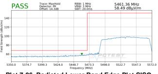
Plot 7-26. Radiated Lower Band Edge Plot SISO ANT1 (Peak – UNII Band 2C)
