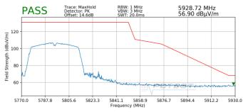
Plot 7-20. Radiated Upper Band Edge Plot SISO ANT1 (Peak – UNII Band 3)
