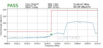
Plot 7-15. Radiated Lower Band Edge Plot SISO ANT1 (Peak – UNII Band 1)
