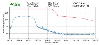
Plot 7-13. Radiated Upper Band Edge Plot SISO ANT1 (Peak – UNII Band 3)
