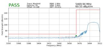
Plot 7-12. Radiated Lower Band Edge Plot SISO ANT1 (Peak – UNII Band 2C)
