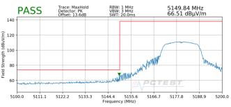
Plot 7-8. Radiated Lower Band Edge Plot SISO ANT1 (Peak – UNII Band 1)
