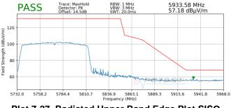
Plot 7-27. Radiated Upper Band Edge Plot SISO ANT1 (Peak – UNII Band 3)
