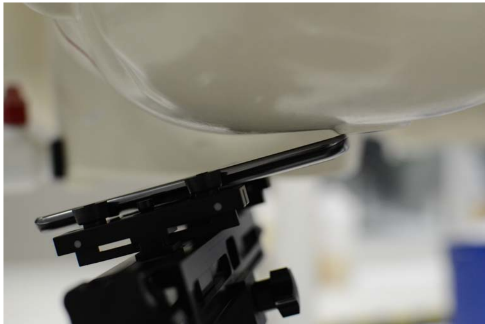
SAR Test Setup Photo 4: Left Tilt
