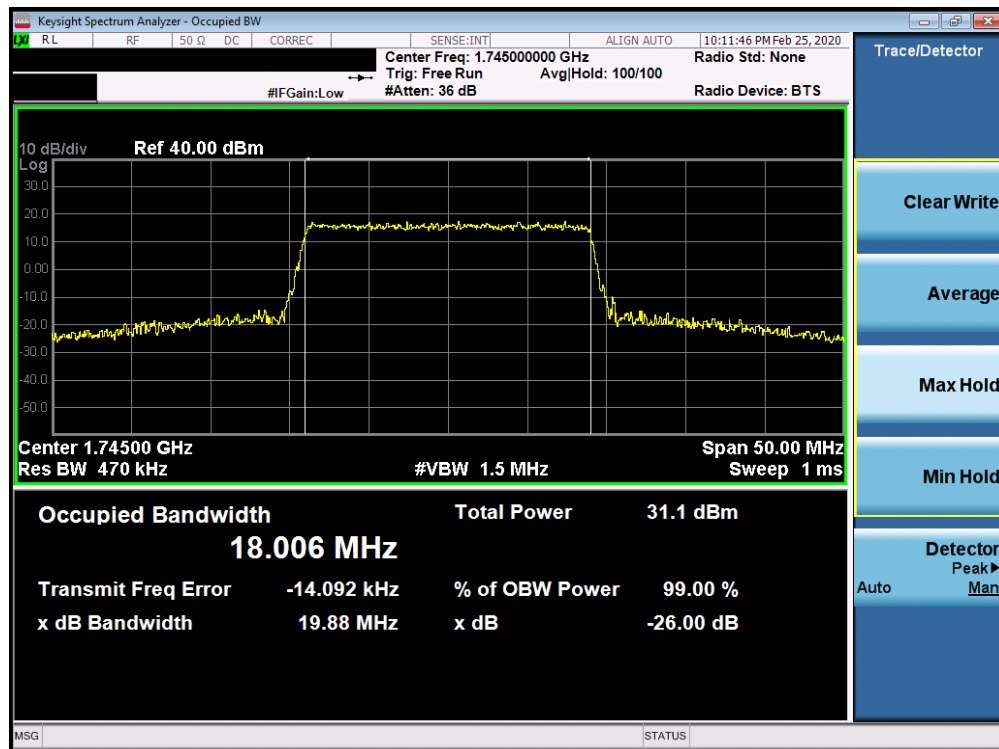
Plot 7-62. Occupied Bandwidth Plot (Band 66/4 - 20.0MHz 16-QAM - Full RB Configuration)
