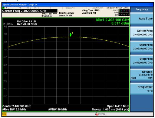
Test Plots (π/4DQPSK) Peak Power (CH.39)
