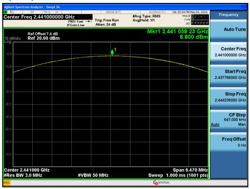
Test Plots (8DPSK) Peak Power (CH.78)
