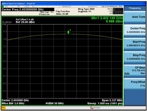
Test Plots (GFSK) Peak Power (CH.39)
