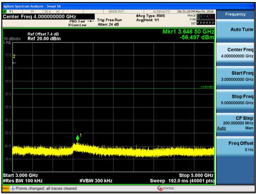
Test Plots (8DPSK)- 5 GHz - 7 GHz Spurious Emission (CH.39)
