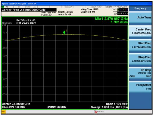
Test Plots (8DPSK) Peak Power (CH.0)
