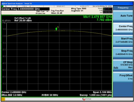
Test Plots (8DPSK) Peak Power (CH.0)
