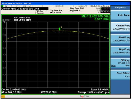
Test Plots (π/4DQPSK) Peak Power (CH.39)
