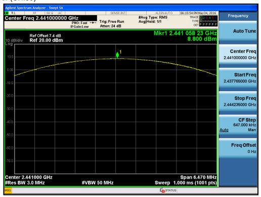
Test Plots (8DPSK) Peak Power (CH.78)
