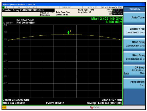
Test Plots (GFSK) Peak Power (CH.39)
