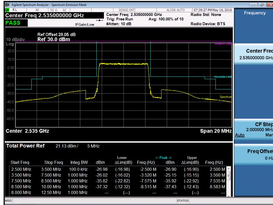
BAND7. High Channel Edge Plot (5MHz Ch.21425 QPSK RB 25)
