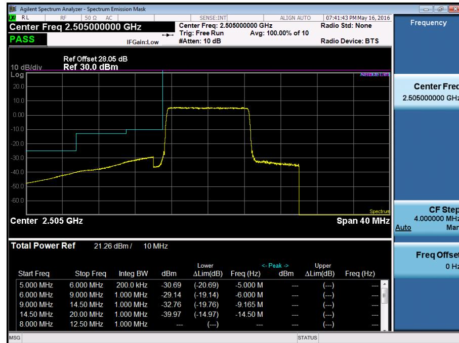
BAND7. Low Channel Edge Plot (10MHz Ch.20800 QPSK RB 50)-2
