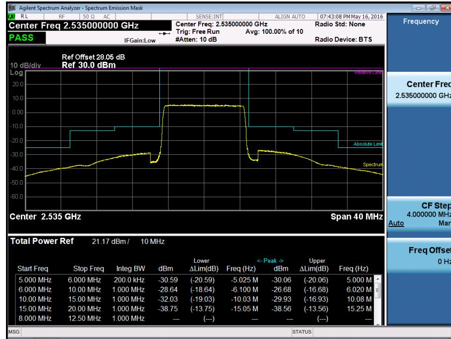
BAND7. High Channel Edge Plot (10MHz Ch.21400 QPSK RB 50)
