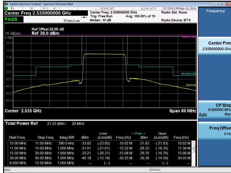
BAND7. High Channel Edge Plot (20MHz Ch.21350 QPSK RB 100)
