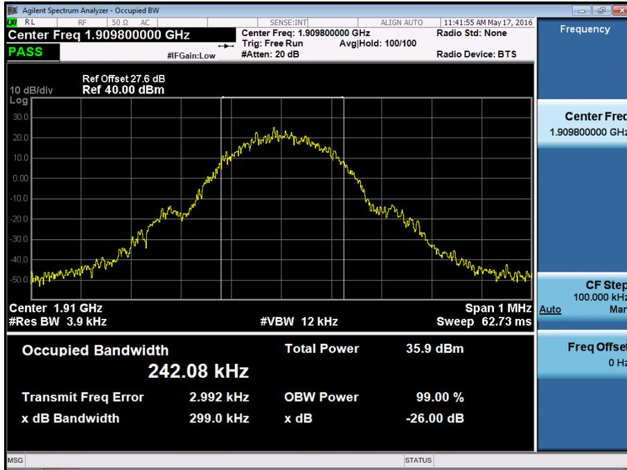
■ GSM1900 EDGE (661 CH.) Occupied Bandwidth
