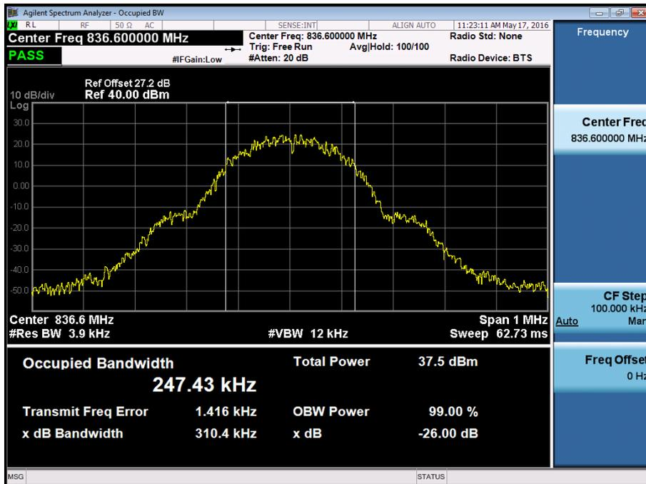
■ GSM850 MODE (251 CH.) Occupied Bandwidth
