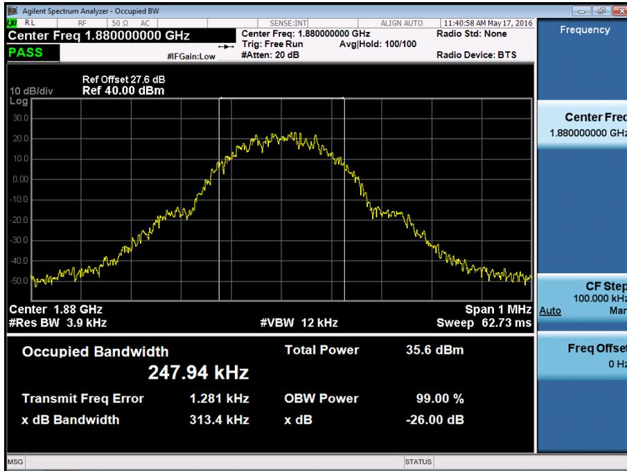
■ GSM1900 MODE (810 CH.) Occupied Bandwidth
