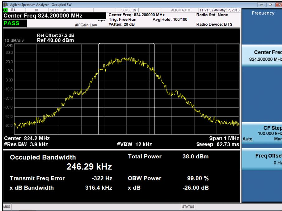
■ GSM850 MODE (190 CH.) Occupied Bandwidth
