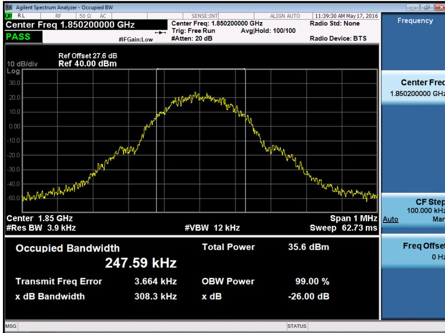
■ GSM1900 MODE (661 CH.) Occupied Bandwidth
