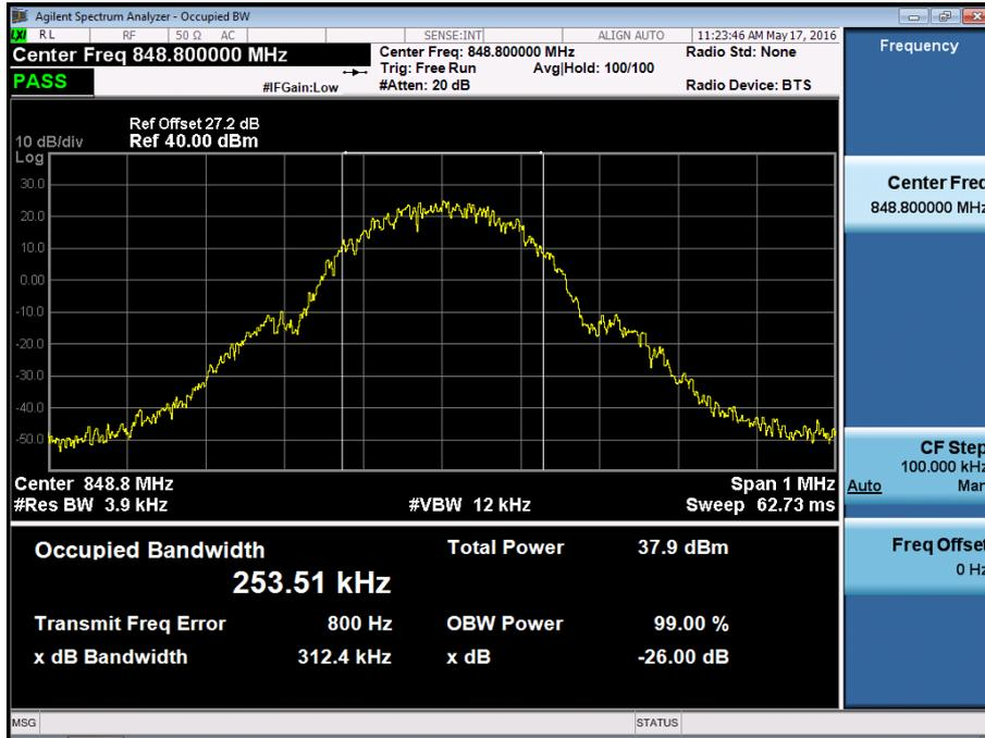
■ GSM850 EDGE (251 CH.) Occupied Bandwidth
