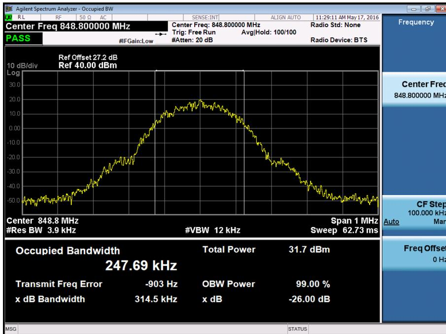
■ GSM1900 MODE (512 CH.) Occupied Bandwidth
