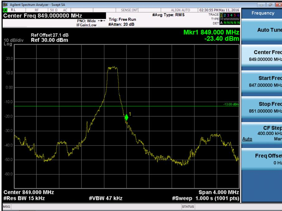
BAND 5. Upper Band Edge Plot (1.4M BW Ch.20643 QPSK\_RB6\_Offset 0)
