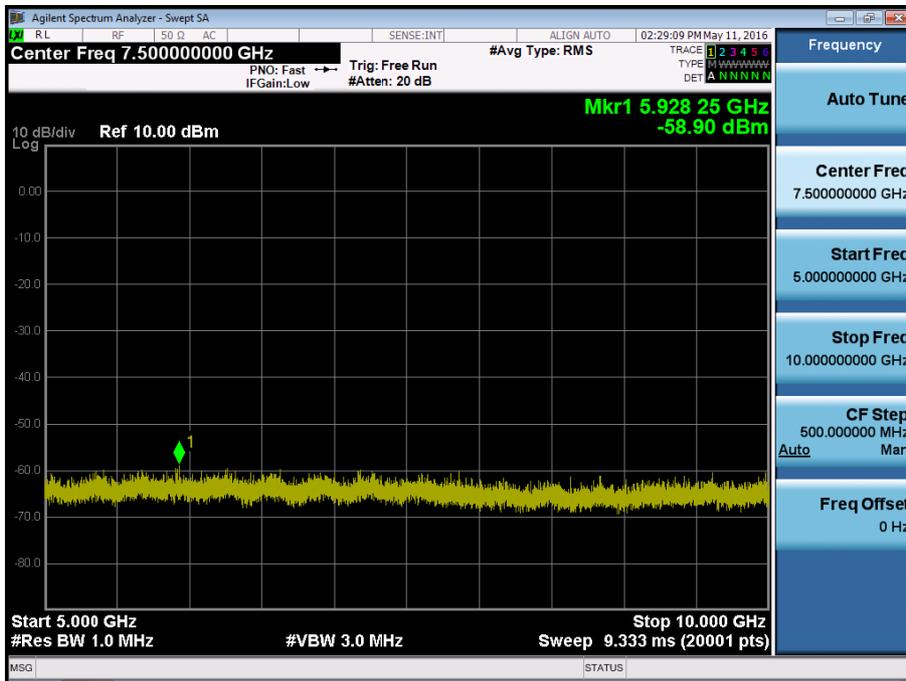
BAND 5. Conducted Spurious Plot \_1 (20525ch\_1.4MHz\_QPSK\_RB 1\_0)
