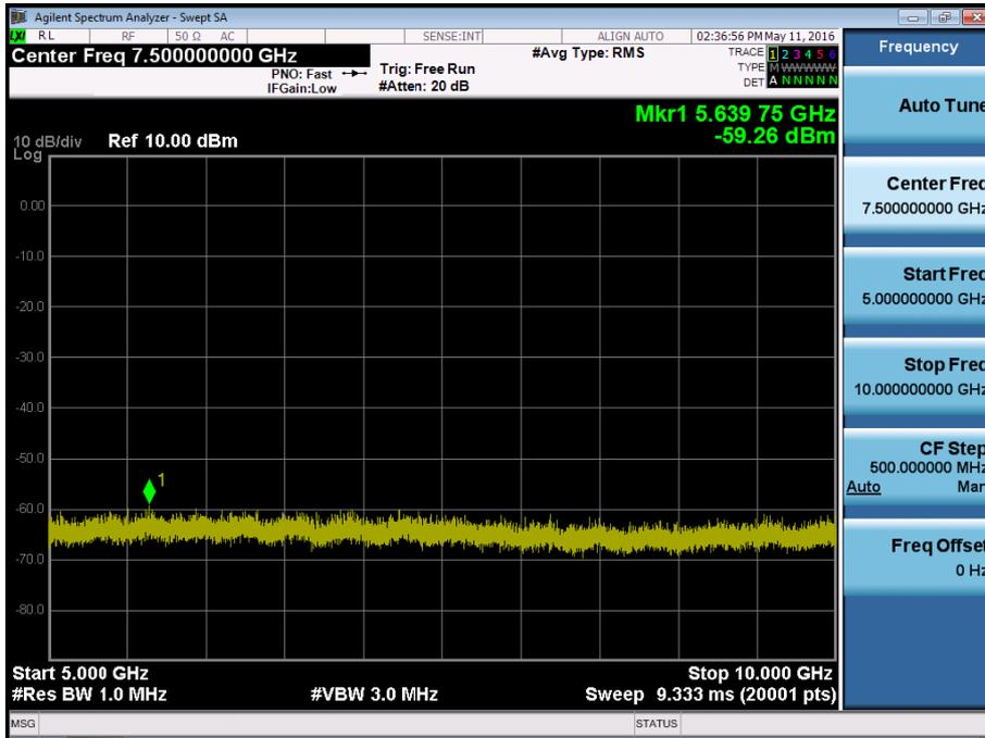
BAND 5. Conducted Spurious Plot \_1 (20625ch\_5MHz\_QPSK\_RB 1\_0)
