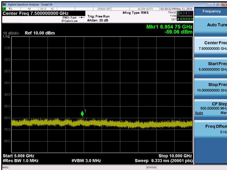
BAND 5. Conducted Spurious Plot \_1 (20643ch\_1.4MHz\_QPSK\_RB 1\_0)
