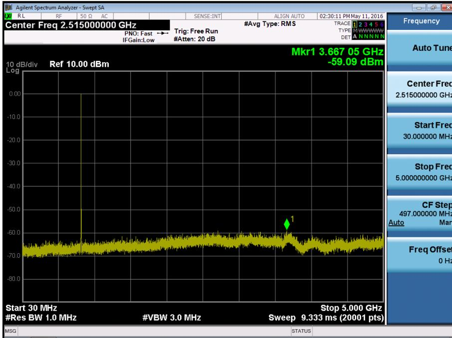
BAND 5. Conducted Spurious Plot \_2 (20525ch\_1.4MHz\_QPSK\_RB 1\_0)
