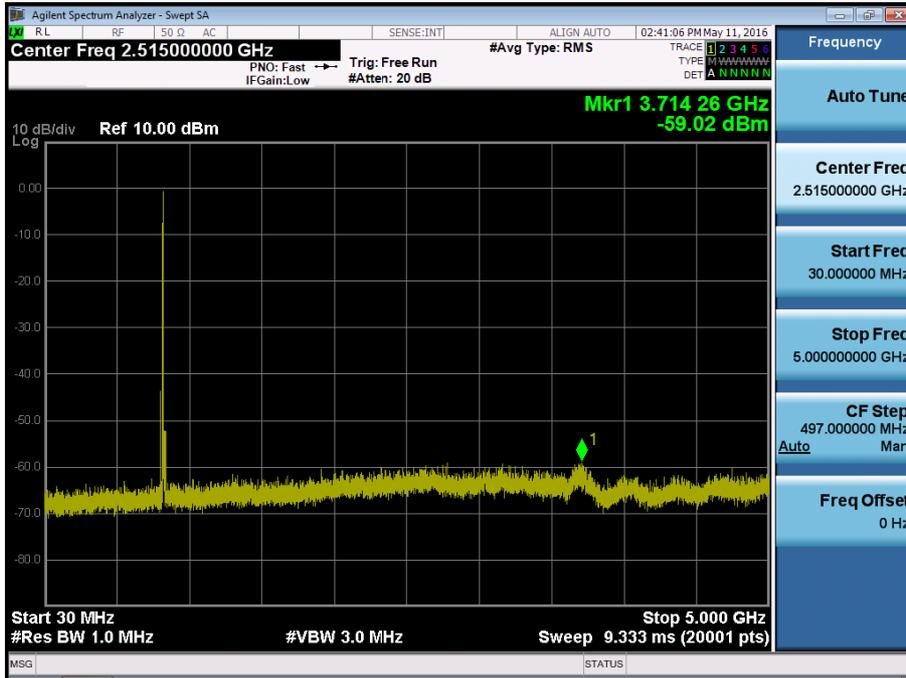
BAND 5. Conducted Spurious Plot \_2 (20600ch\_10MHz\_QPSK\_RB 1\_0)
