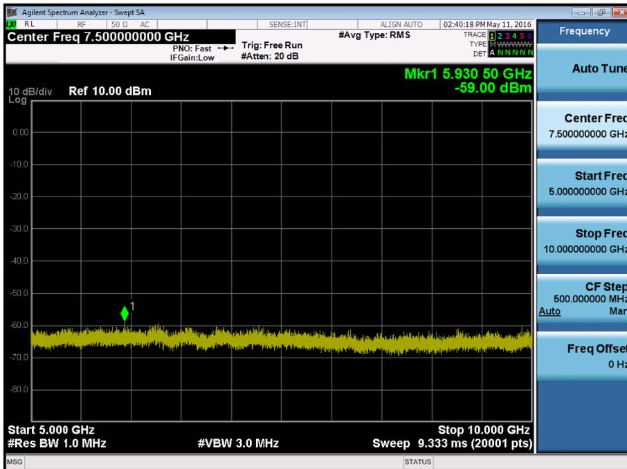
BAND 5. Conducted Spurious Plot \_1 (20600ch\_10MHz\_QPSK\_RB 1\_0)
