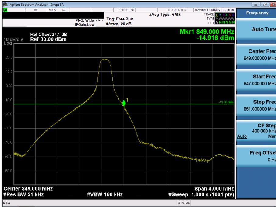
BAND 5. Upper Band Edge Plot (5M BW Ch.20625 QPSK\_RB25\_Offset 0)
