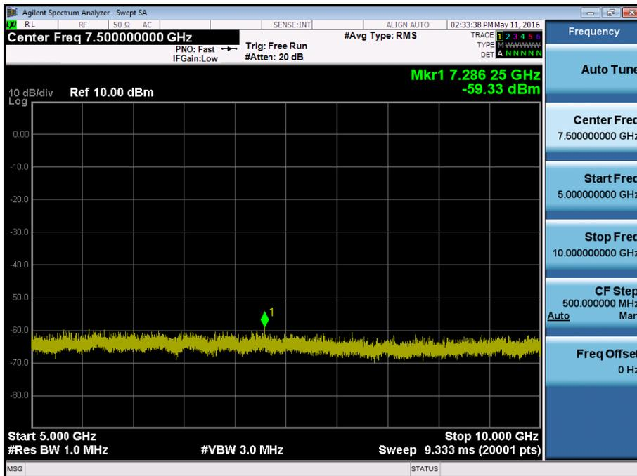
BAND 5. Conducted Spurious Plot \_1 (20635ch\_3MHz\_QPSK\_RB 1\_0)
