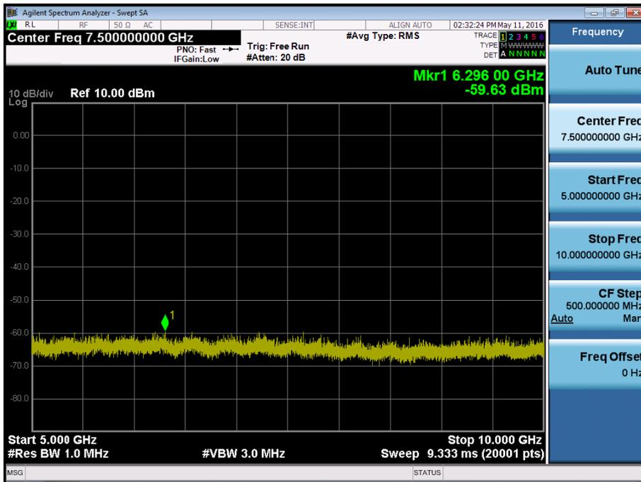
BAND 5. Conducted Spurious Plot \_1 (20525ch\_3MHz\_QPSK\_RB 1\_0)
