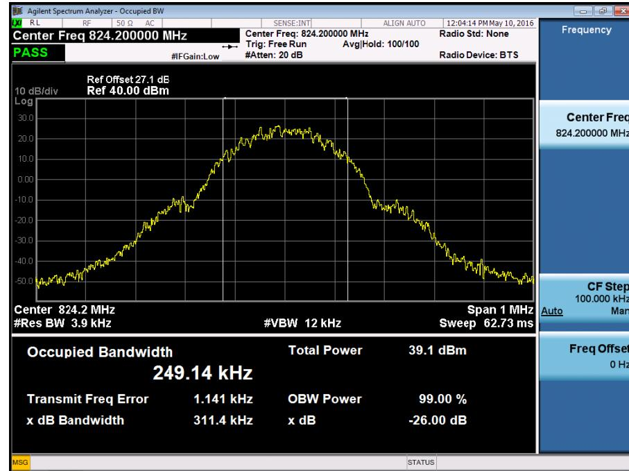
■ GSM850 MODE (190 CH.) Occupied Bandwidth
