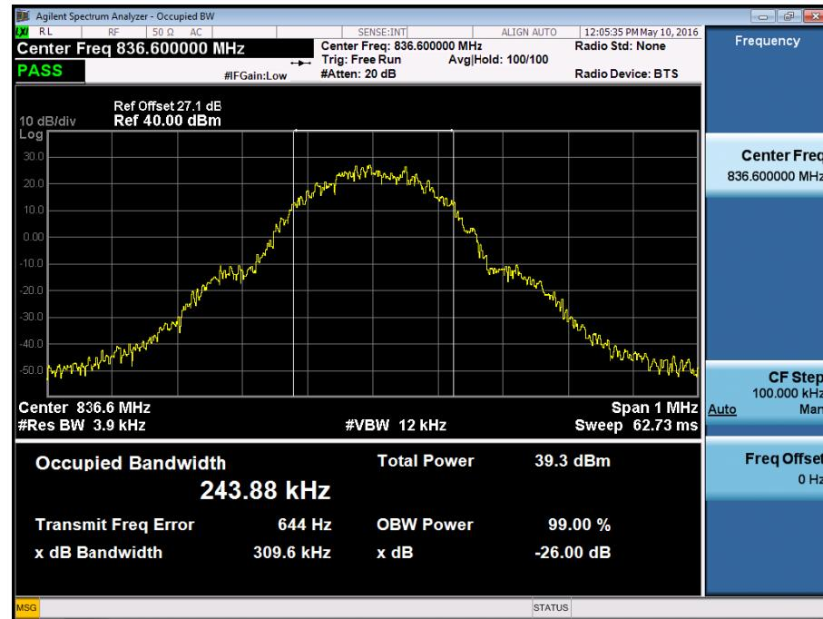
■ GSM850 MODE (251 CH.) Occupied Bandwidth
