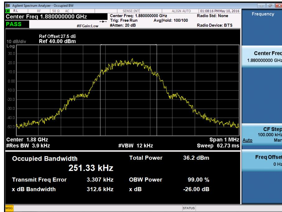
■ GSM1900 MODE (810 CH.) Occupied Bandwidth
