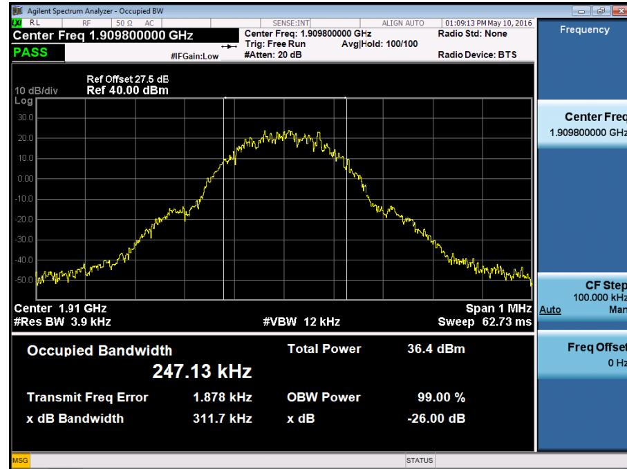
■ GSM1900 EDGE (661 CH.) Occupied Bandwidth
