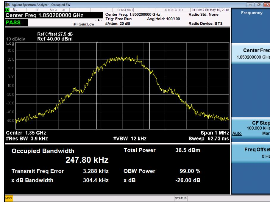
■ GSM1900 MODE (661 CH.) Occupied Bandwidth
