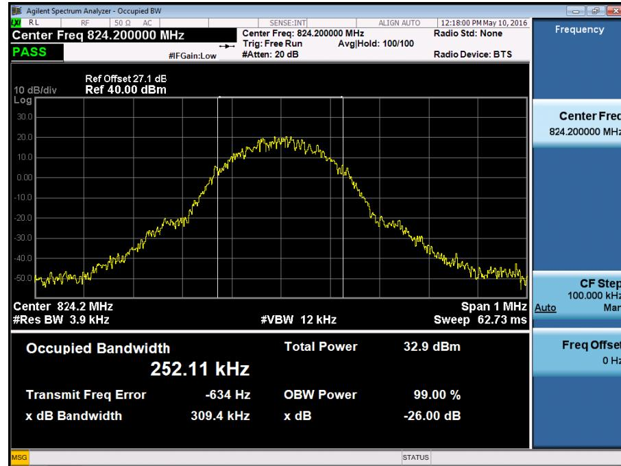
■ GSM1900 MODE (512 CH.) Occupied Bandwidth
