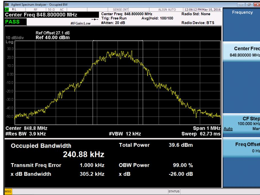
■ GSM850 EDGE (128 CH.) Occupied Bandwidth
