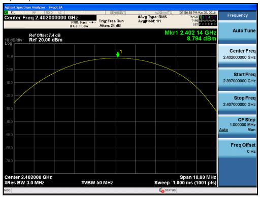
Test Plots (GFSK) Peak Power (CH.39)
