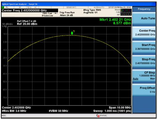
Test Plots (π/4DQPSK) Peak Power (CH.39)
