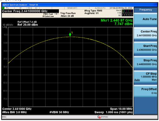
Test Plots (8DPSK) Peak Power (CH.78)
