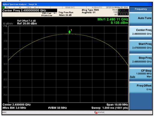
Test Plots (8DPSK) Peak Power (CH.0)
