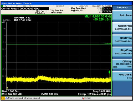
Test Plots (8DPSK)- 5 GHz - 7 GHz Spurious Emission (CH.78)
