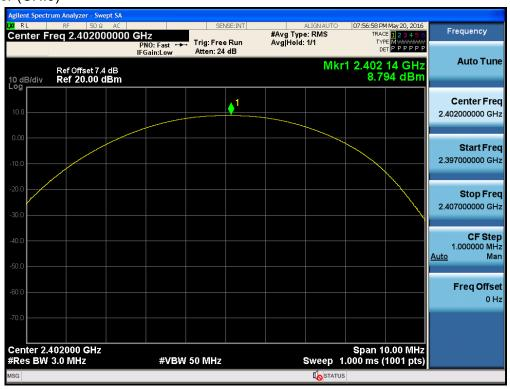
Test Plots (GFSK) Peak Power (CH.39)
