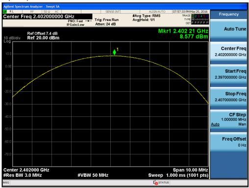
Test Plots (π/4DQPSK) Peak Power (CH.39)
