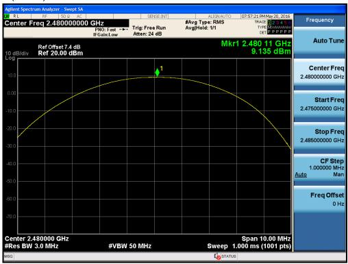
Test Plots (8DPSK) Peak Power (CH.0)
