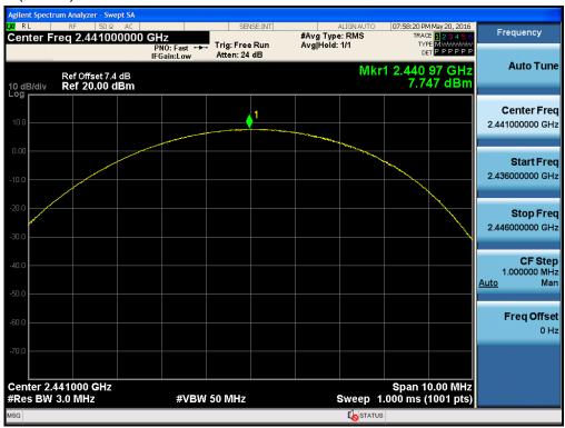
Test Plots (8DPSK) Peak Power (CH.78)
