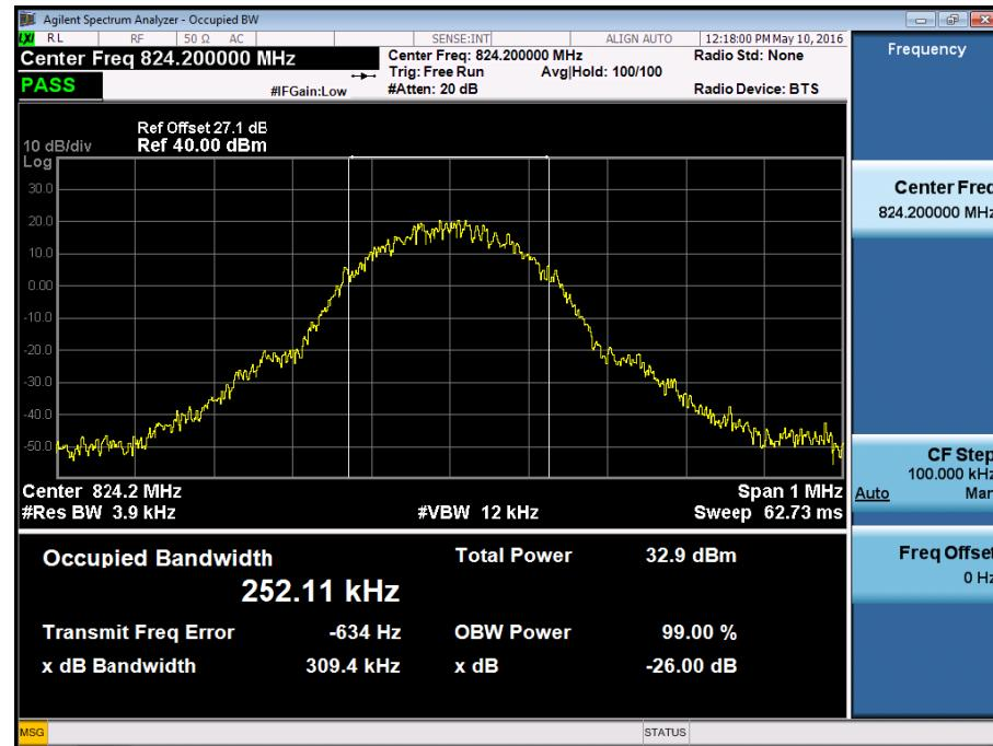
■ GSM1900 MODE (512 CH.) Occupied Bandwidth
