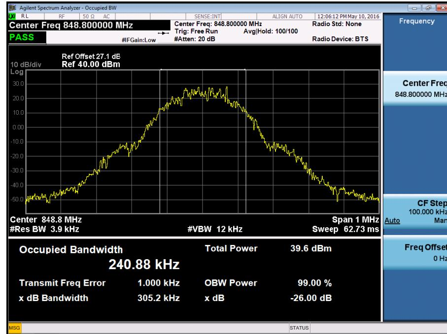
■ GSM850 EDGE (128 CH.) Occupied Bandwidth
