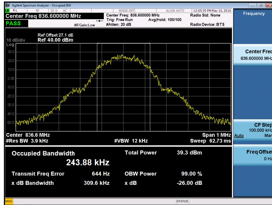
■ GSM850 MODE (251 CH.) Occupied Bandwidth
