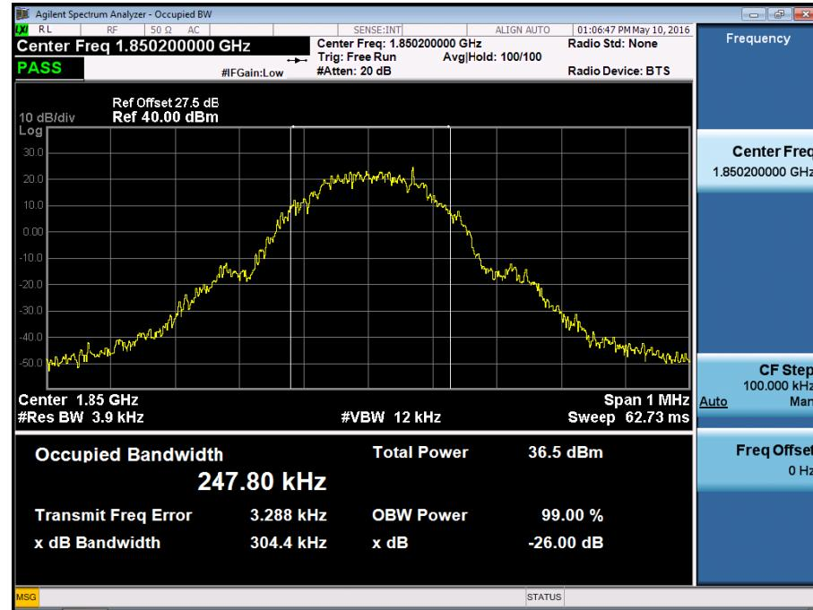
■ GSM1900 MODE (661 CH.) Occupied Bandwidth
