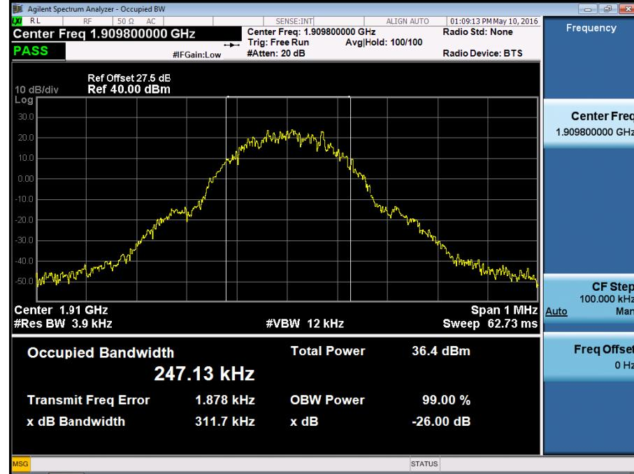
■ GSM1900 EDGE (661 CH.) Occupied Bandwidth
