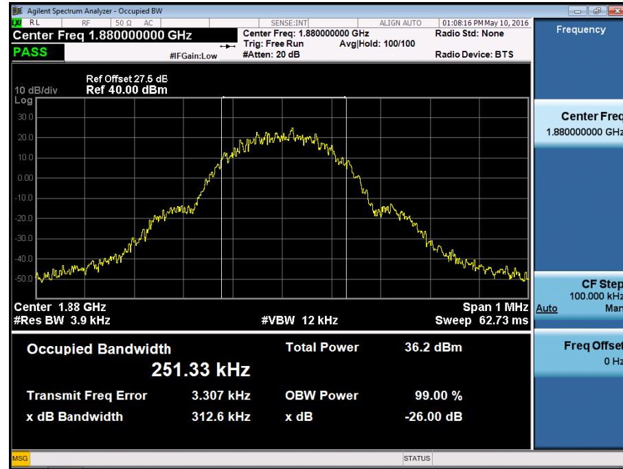
■ GSM1900 MODE (810 CH.) Occupied Bandwidth
