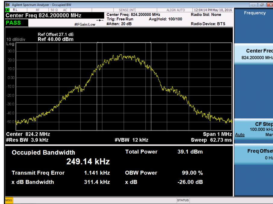
■ GSM850 MODE (190 CH.) Occupied Bandwidth
