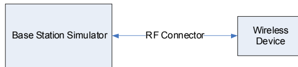
Figure 9-2 Power Measurement Setup
