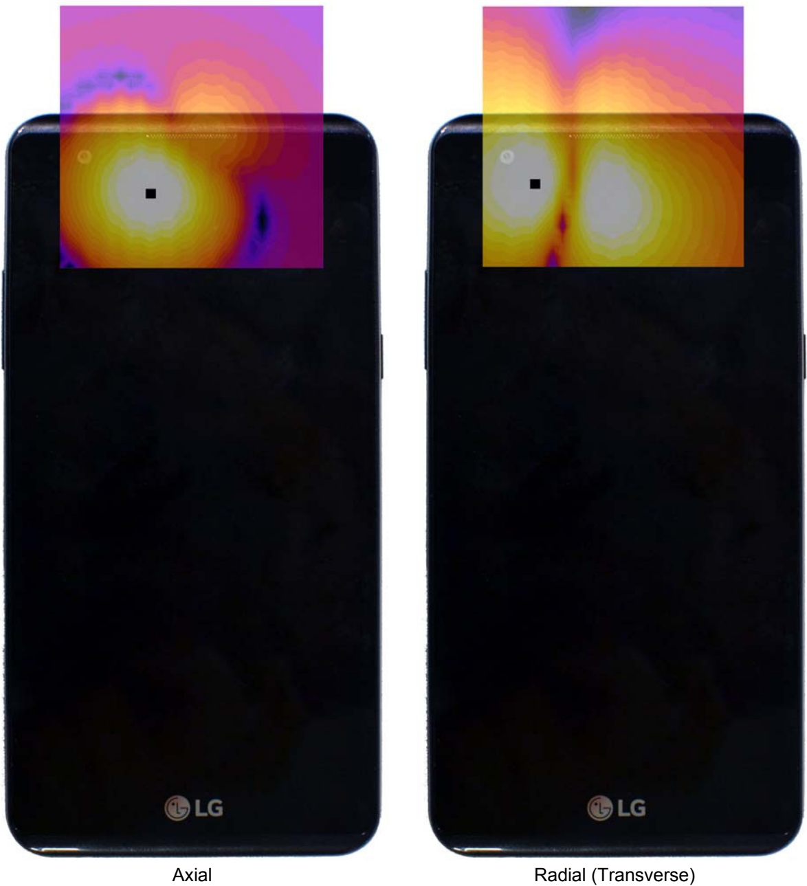
Figure 14-3 T-Coil Scan Overlay Magnetic Field Distributions
