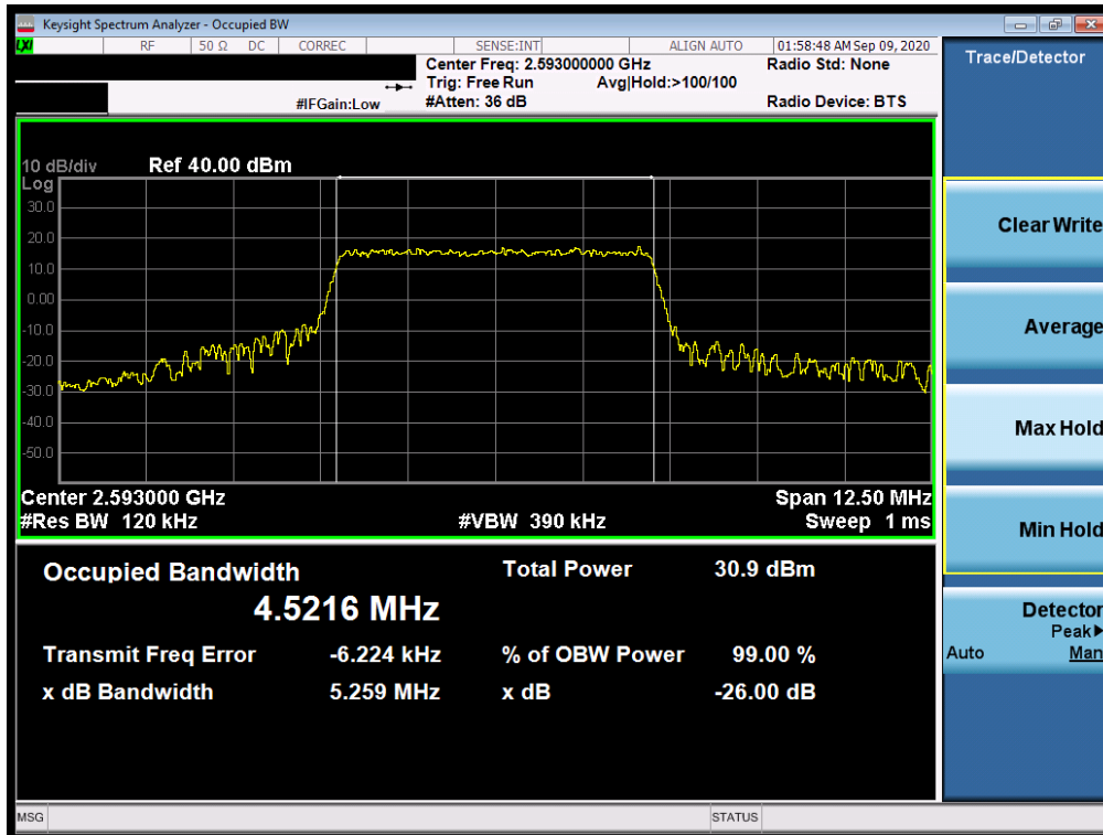
Plot 7-12. Occupied Bandwidth Plot (LTE Band 41(PC2) - 5MHz 64-QAM - Full RB Configuration)
