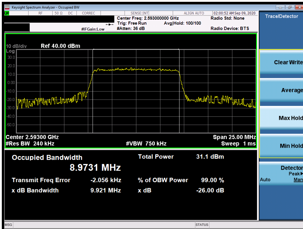
Plot 7-8. Occupied Bandwidth Plot (LTE Band 41(PC2) - 10MHz 16-QAM - Full RB Configuration)
