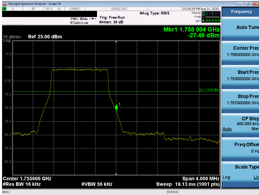
Plot 7-110. Upper Band Edge Plot (LTE Band 4 – 1.4MHz QPSK – Full RB Configuration)
