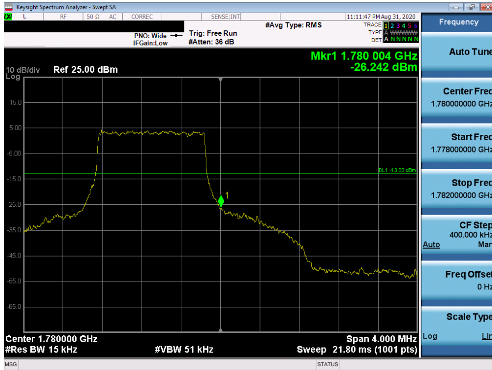
Plot 7-112. Upper Band Edge Plot (LTE Band 66 – 1.4MHz QPSK – Full RB Configuration)
