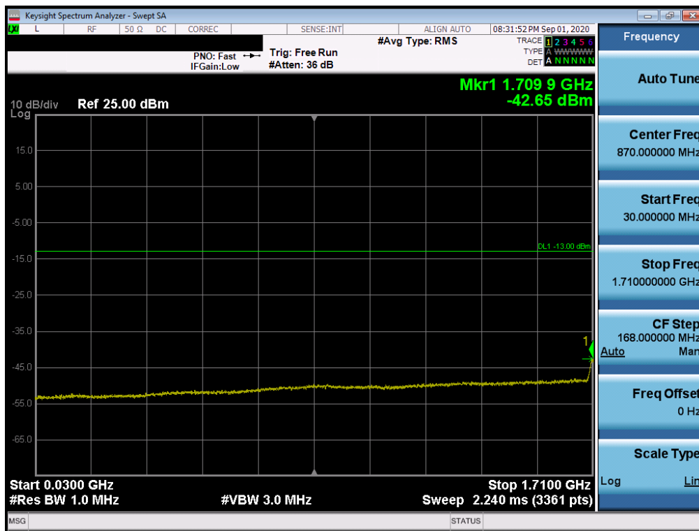
Plot 7-138. Conducted Spurious Plot (LTE Band 66/4 - 20MHz QPSK - RB Size 1, RB Offset 0 - MidChannel)
