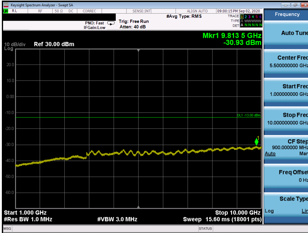
Plot 7-122. Conducted Spurious Plot (LTE Band 71 - 20MHz QPSK - RB Size 1, RB Offset 0 - High Channel)
