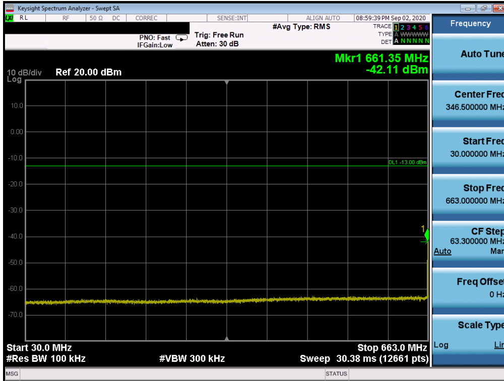
Plot 7-120. Conducted Spurious Plot (LTE Band 71 - 20MHz QPSK - RB Size 1, RB Offset 0 - High Channel)
