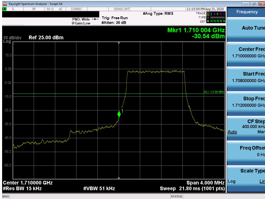
Plot 7-108. Lower Band Edge Plot (LTE Band 66/4 – 1.4MHz QPSK – Full RB Configuration)
