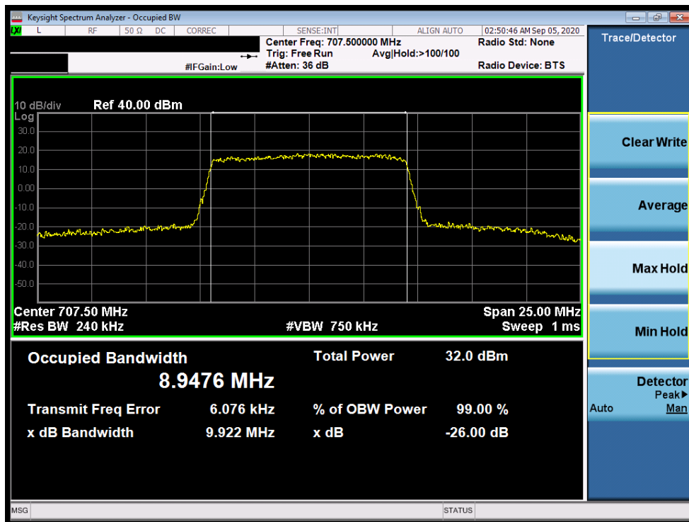
Plot 7-14. Occupied Bandwidth Plot (LTE Band 12 - 10MHz 16-QAM - Full RB Configuration)
