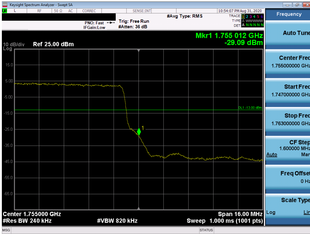
Plot 7-80. Upper Band Edge Plot (LTE Band 4 - 20MHz QPSK – Full RB Configuration)
