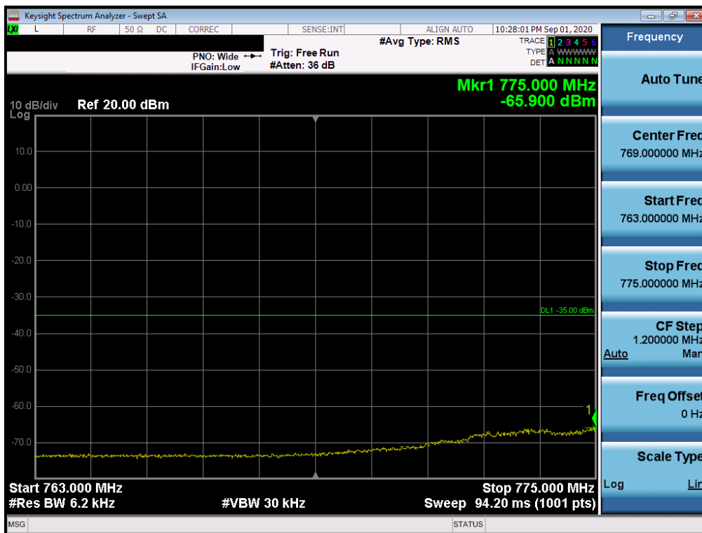
Plot 7-67. Lower Emission Mask Plot (LTE Band 13 - 10MHz QPSK – Full RB Configuration)
