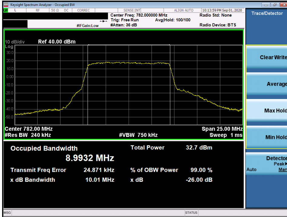
Plot 7-25. Occupied Bandwidth Plot (LTE Band 13 - 10MHz QPSK - Full RB Configuration)
