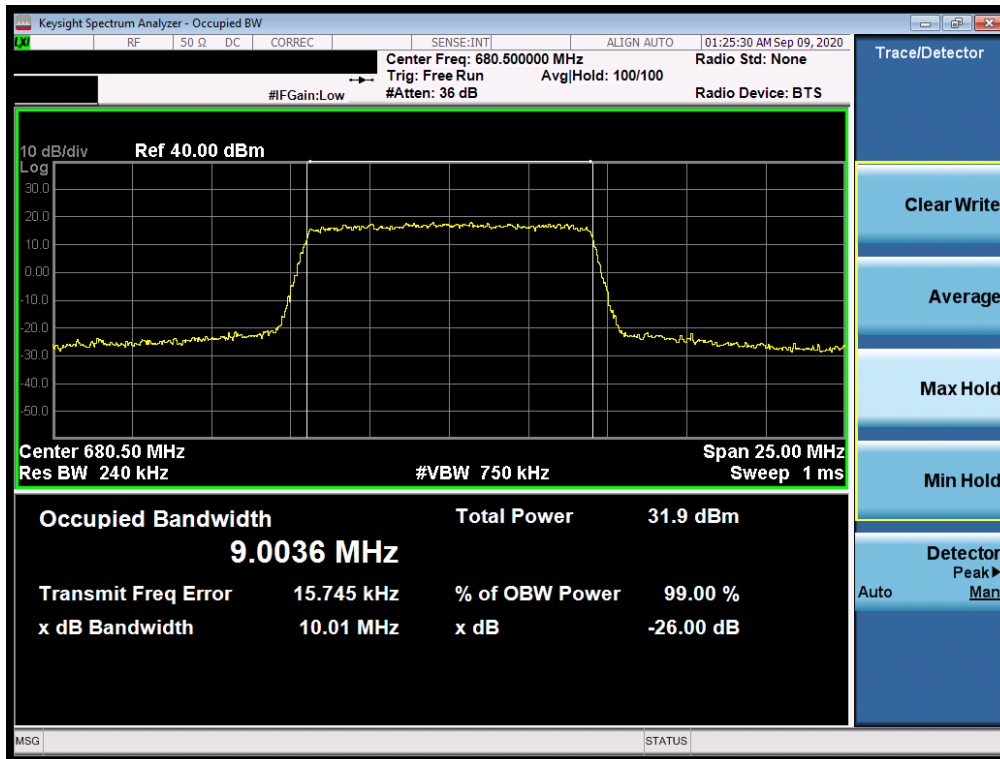
Plot 7-7. Occupied Bandwidth Plot (LTE Band 71 - 10MHz QPSK - Full RB Configuration)
