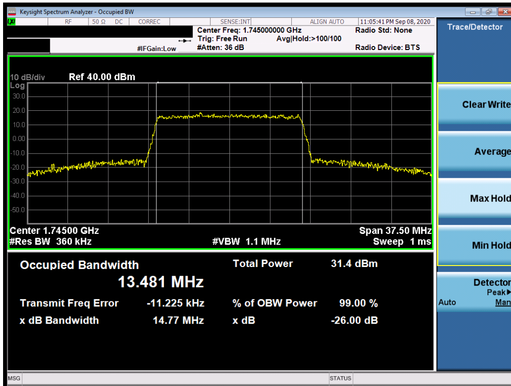
Plot 7-37. Occupied Bandwidth Plot (LTE Band 66/4 - 15MHz 64-QAM - Full RB Configuration)
