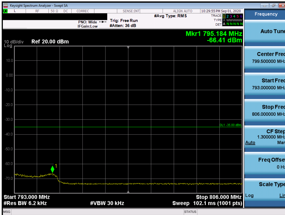
Plot 7-69. Upper Emission Mask Plot (LTE Band 13 - 10MHz QPSK – Full RB Configuration)
