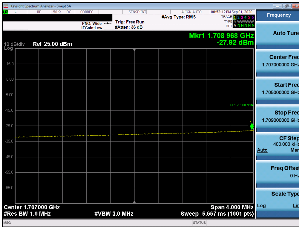
Plot 7-79. Lower Extended Band Edge Plot (LTE Band 66/4 - 20MHz QPSK – Full RB Configuration)
