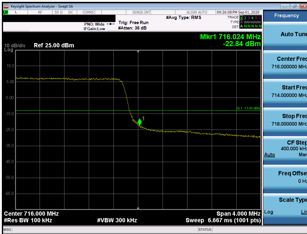
Plot 7-61. Upper Band Edge Plot (LTE Band 12 - 5MHz QPSK – Full RB Configuration)
