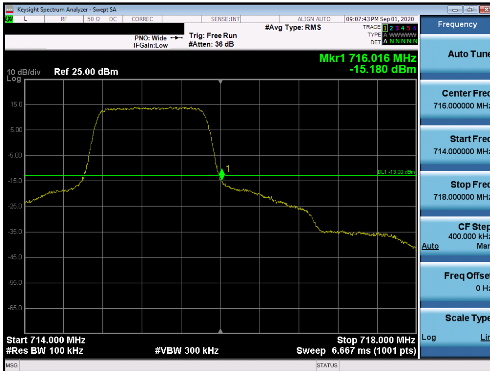
Plot 7-65. Upper Band Edge Plot (LTE Band 12 – 1.4MHz QPSK – Full RB Configuration)
