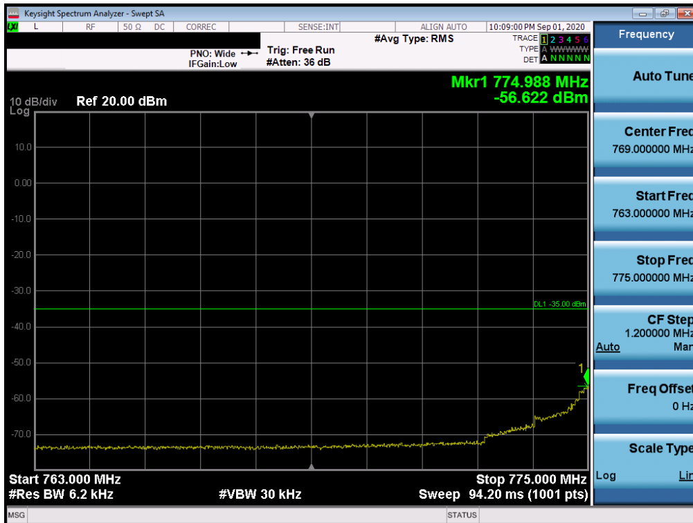
Plot 7-71. Lower Emission Mask Plot (LTE Band 13 - 5MHz QPSK – Full RB Configuration)
