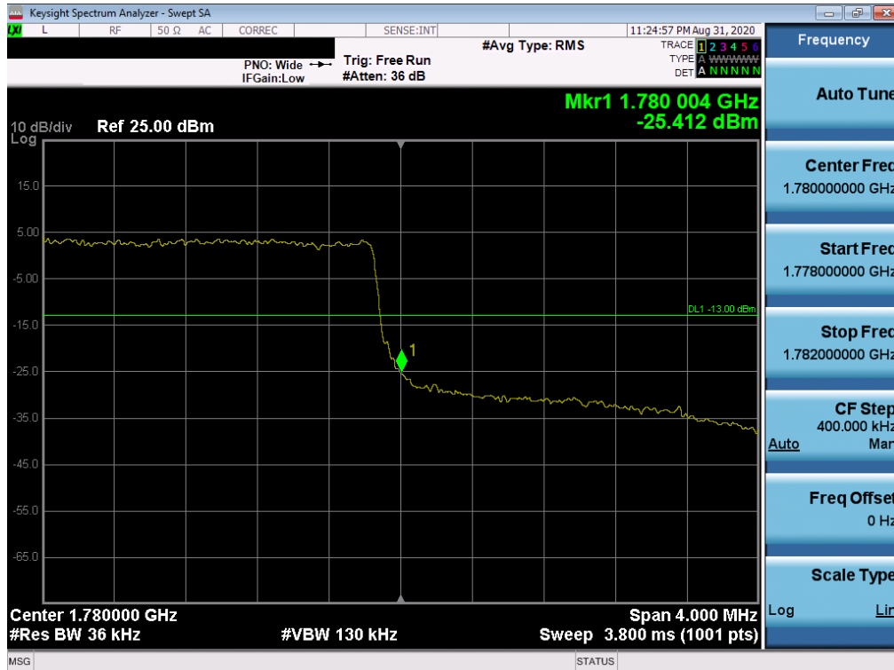
Plot 7-106. Upper Band Edge Plot (LTE Band 66 - 3MHz QPSK – Full RB Configuration)
