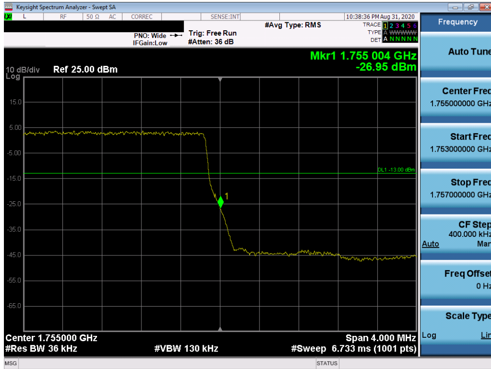
Plot 7-104. Upper Band Edge Plot (LTE Band 4 - 3MHz QPSK – Full RB Configuration)
