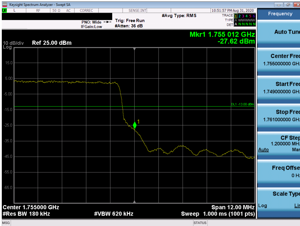
Plot 7-86. Upper Band Edge Plot (LTE Band 4 - 15MHz QPSK – Full RB Configuration)
