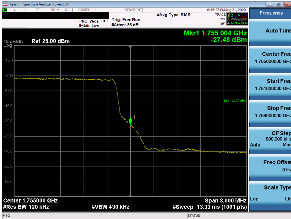
Plot 7-92. Upper Band Edge Plot (LTE Band 4 - 10MHz QPSK – Full RB Configuration)
