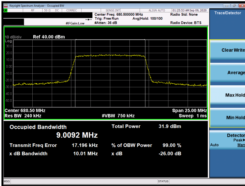
Plot 7-8. Occupied Bandwidth Plot (LTE Band 71 - 10MHz 16-QAM - Full RB Configuration)
