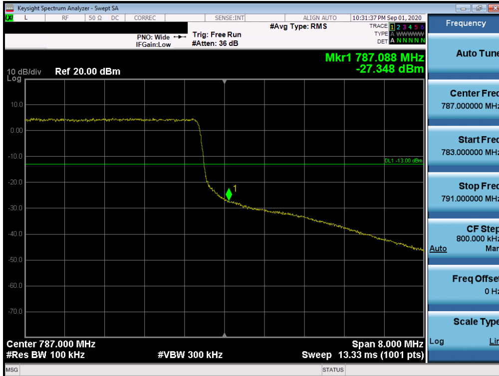
Plot 7-68. Upper Band Edge Plot (LTE Band 13 - 10MHz QPSK – Full RB Configuration)
