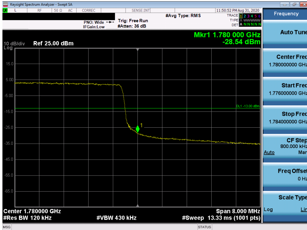
Plot 7-94. Upper Band Edge Plot (LTE Band 66 - 10MHz QPSK – Full RB Configuration)
