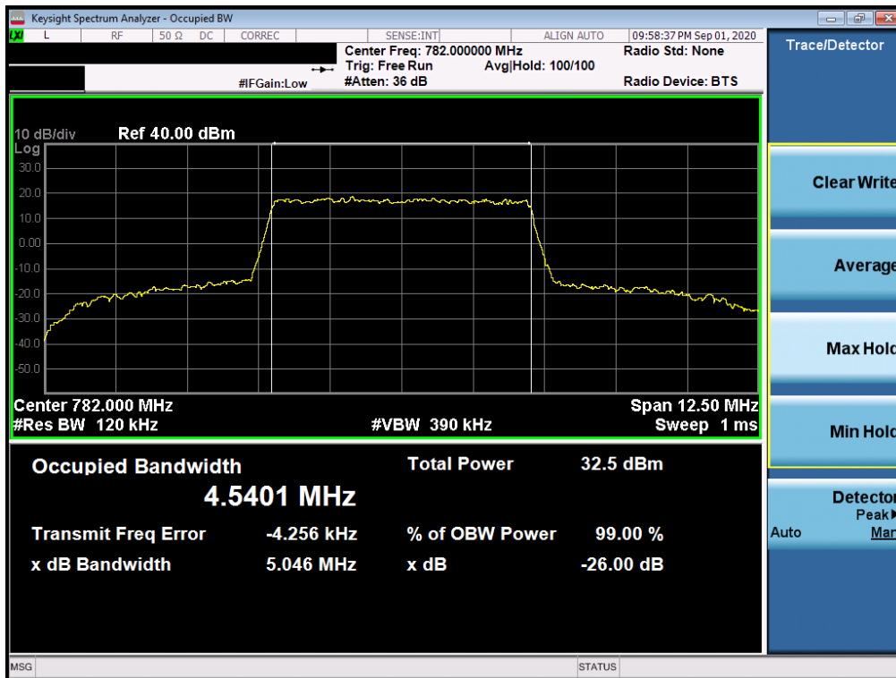
Plot 7-28. Occupied Bandwidth Plot (LTE Band 13 - 5MHz QPSK - Full RB Configuration)
