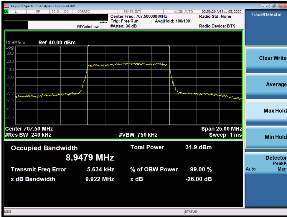
Plot 7-13. Occupied Bandwidth Plot (LTE Band 12 - 10MHz QPSK - Full RB Configuration)
