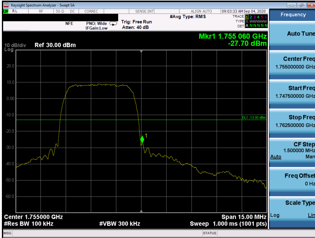
Plot 7-76. Upper Band Edge Plot (WCDMA AWS – Ch.1513)
