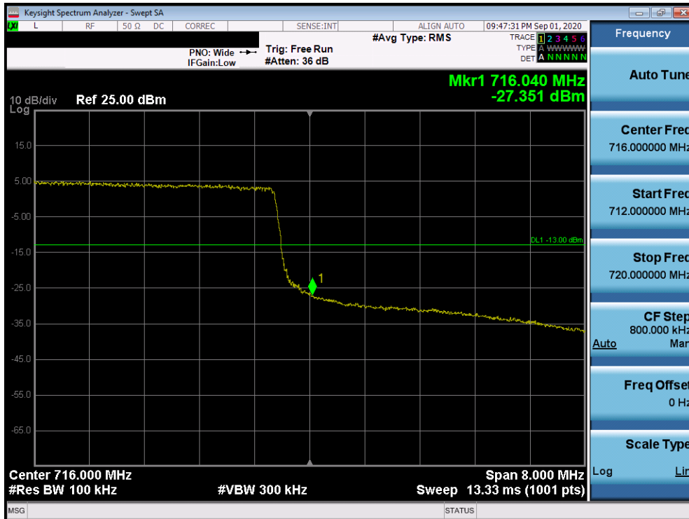
Plot 7-59. Upper Band Edge Plot (LTE Band 12 - 10MHz QPSK – Full RB Configuration)
