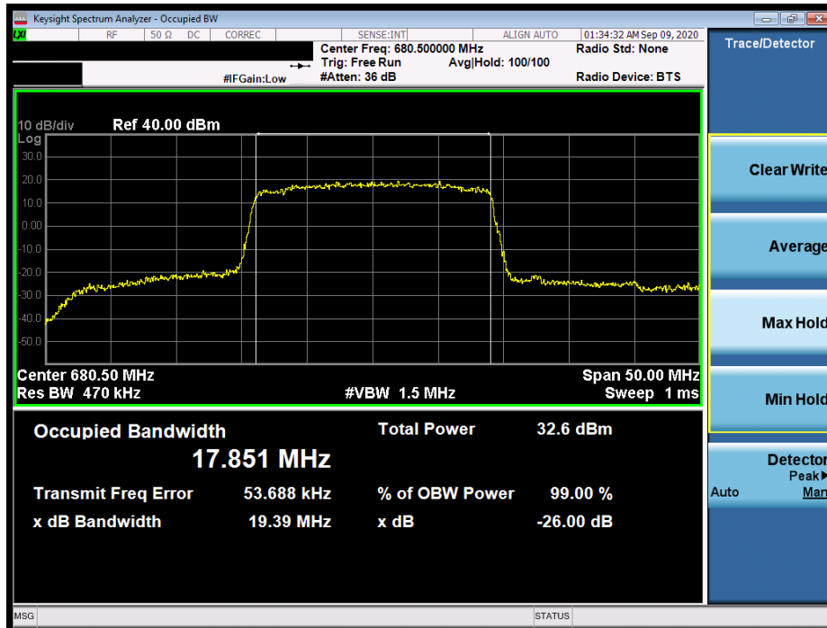
Plot 7-2. Occupied Bandwidth Plot (LTE Band 71 - 20MHz 16-QAM - Full RB Configuration)
