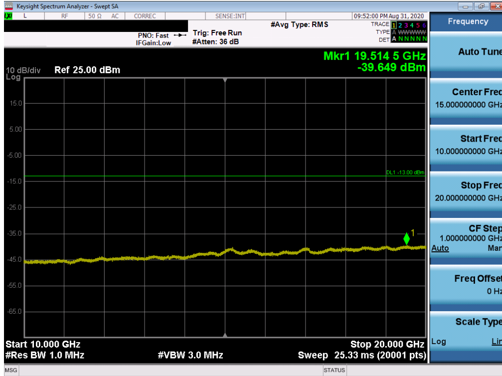
Plot 7-30. Conducted Spurious Plot (LTE Band 25/2 - 20MHz QPSK - RB Size 1, RB Offset 0 - High Channel)
