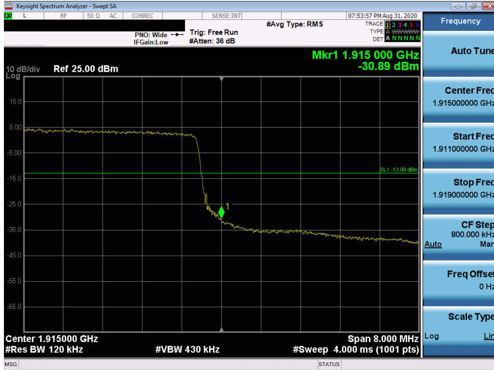
Plot 7-71. Upper Band Edge Plot (LTE Band 25 - 10MHz QPSK – Full RB Configuration)
