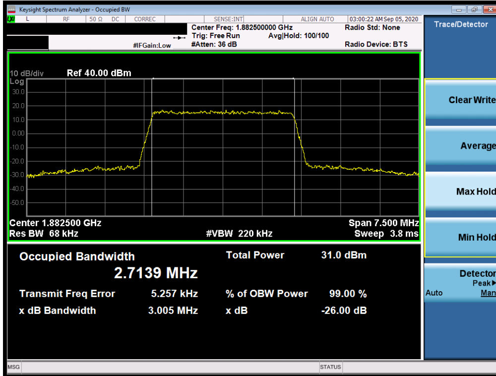
Plot 7-13. Occupied Bandwidth Plot (LTE Band 25/2 - 3MHz QPSK - Full RB Configuration)
