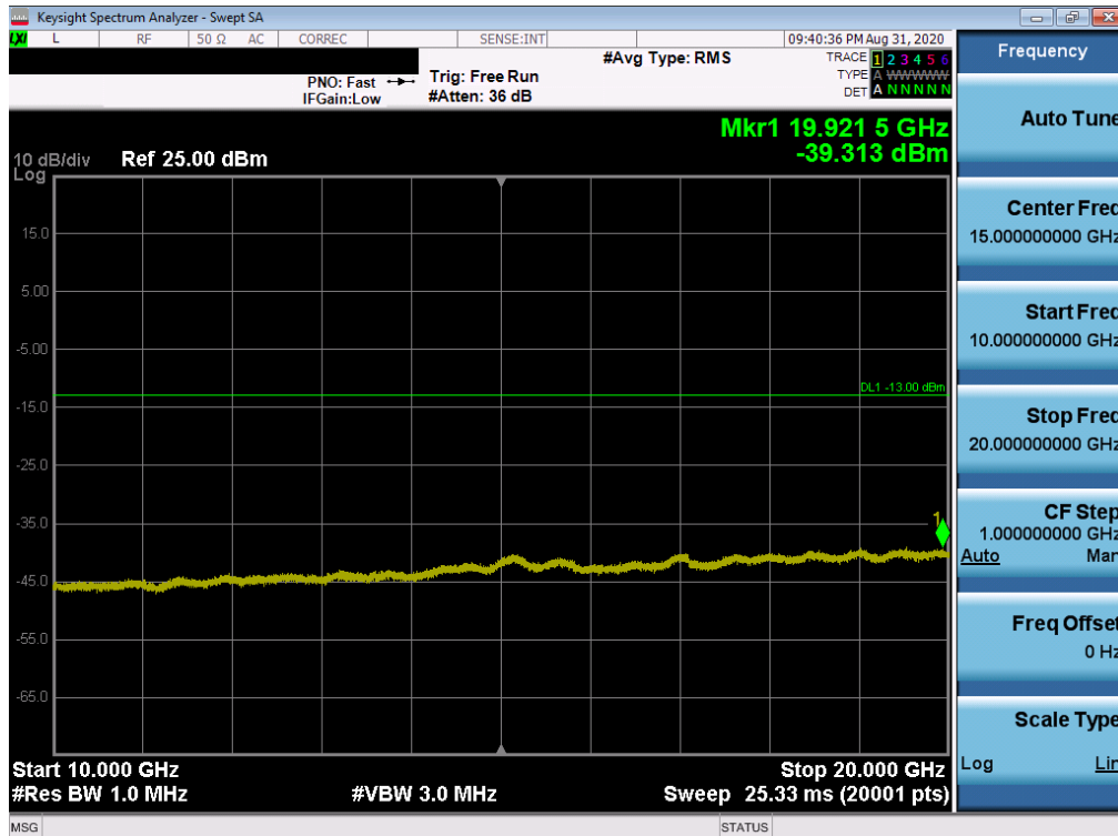
Plot 7-24. Conducted Spurious Plot (LTE Band 25/2 - 20MHz QPSK - RB Size 1, RB Offset 0 - Low Channel)
