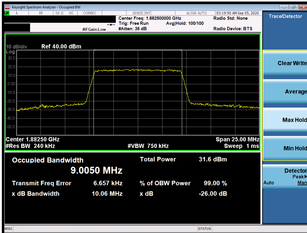
Plot 7-8. Occupied Bandwidth Plot (LTE Band 25/2 - 10MHz 16-QAM - Full RB Configuration)
