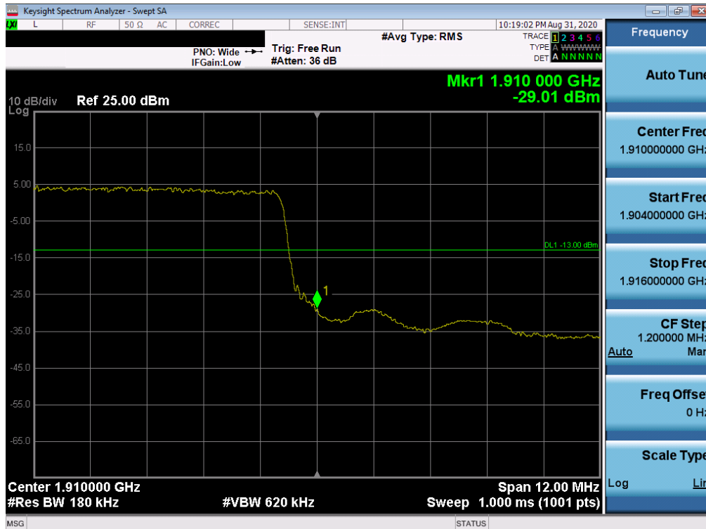
Plot 7-63. Upper Band Edge Plot (LTE Band 2 - 15MHz QPSK – Full RB Configuration)
