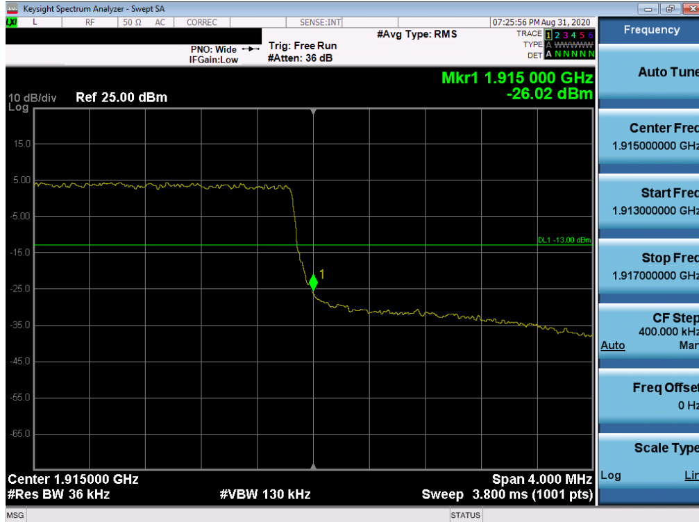
Plot 7-83. Upper Band Edge Plot (LTE Band 25 - 3MHz QPSK – Full RB Configuration)
