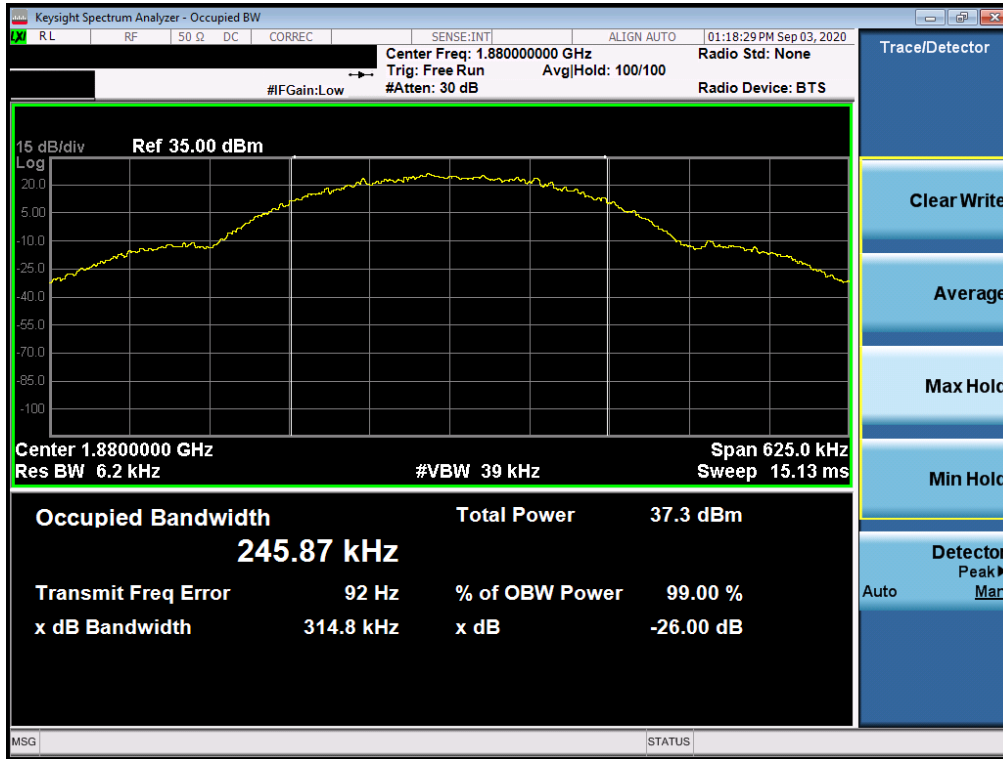
Plot 7-19. Occupied Bandwidth Plot (GPRS, Ch. 661)
