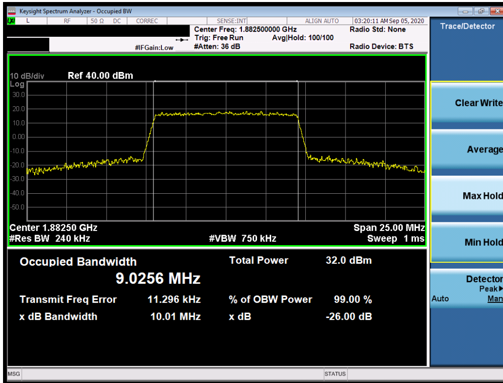
Plot 7-9. Occupied Bandwidth Plot (LTE Band 25/2 - 10MHz 64-QAM - Full RB Configuration)
