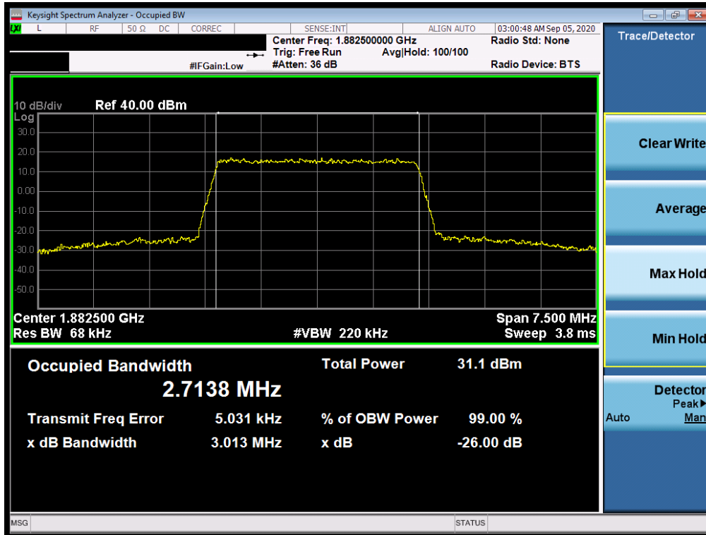
Plot 7-14. Occupied Bandwidth Plot (LTE Band 25/2 - 3MHz 16-QAM - Full RB Configuration)
