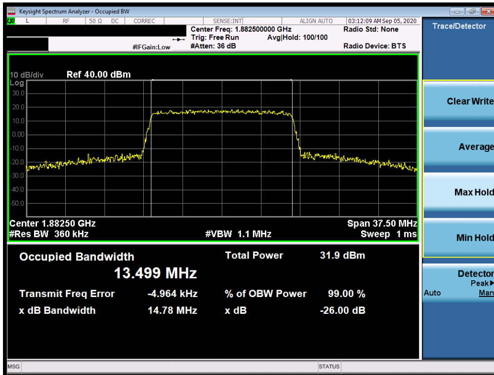
Plot 7-6. Occupied Bandwidth Plot (LTE Band 25/2 - 15MHz 64-QAM - Full RB Configuration)
