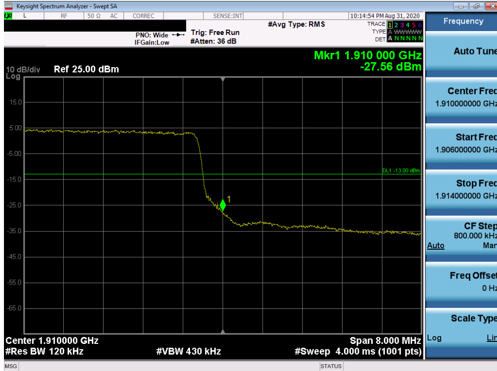
Plot 7-69. Upper Band Edge Plot (LTE Band 2 - 10MHz QPSK – Full RB Configuration)
