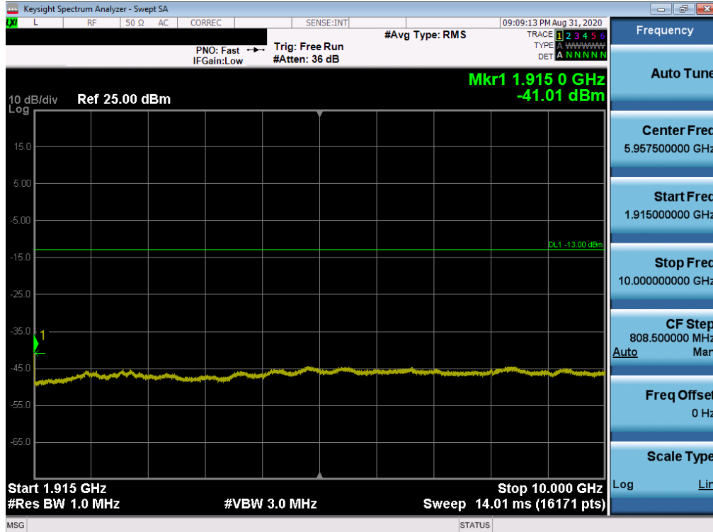
Plot 7-26. Conducted Spurious Plot (LTE Band 25/2 - 20MHz QPSK - RB Size 1, RB Offset 0 - Mid Channel)
