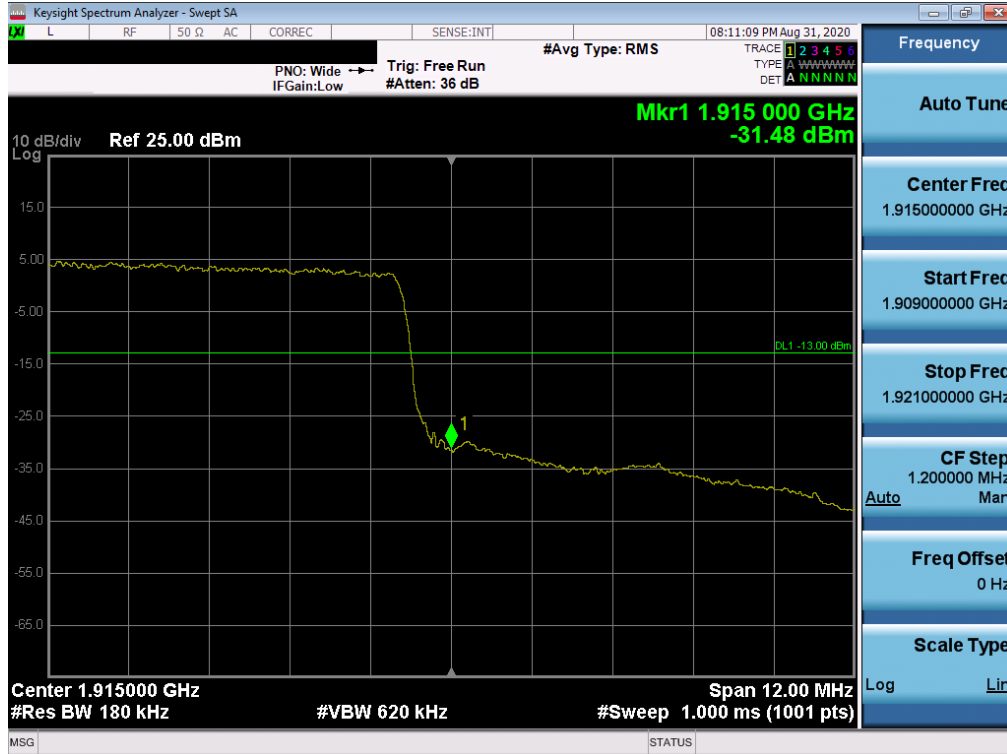
Plot 7-65. Upper Band Edge Plot (LTE Band 25 - 15MHz QPSK – Full RB Configuration)
