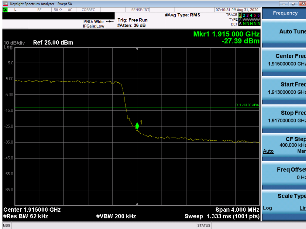
Plot 7-77. Upper Band Edge Plot (LTE Band 25 - 5MHz QPSK – Full RB Configuration)
