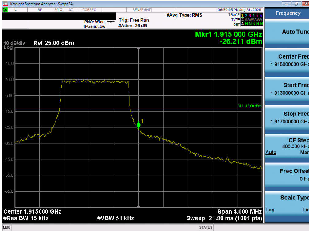
Plot 7-89. Upper Band Edge Plot (LTE Band 25 – 1.4MHz QPSK – Full RB Configuration)
