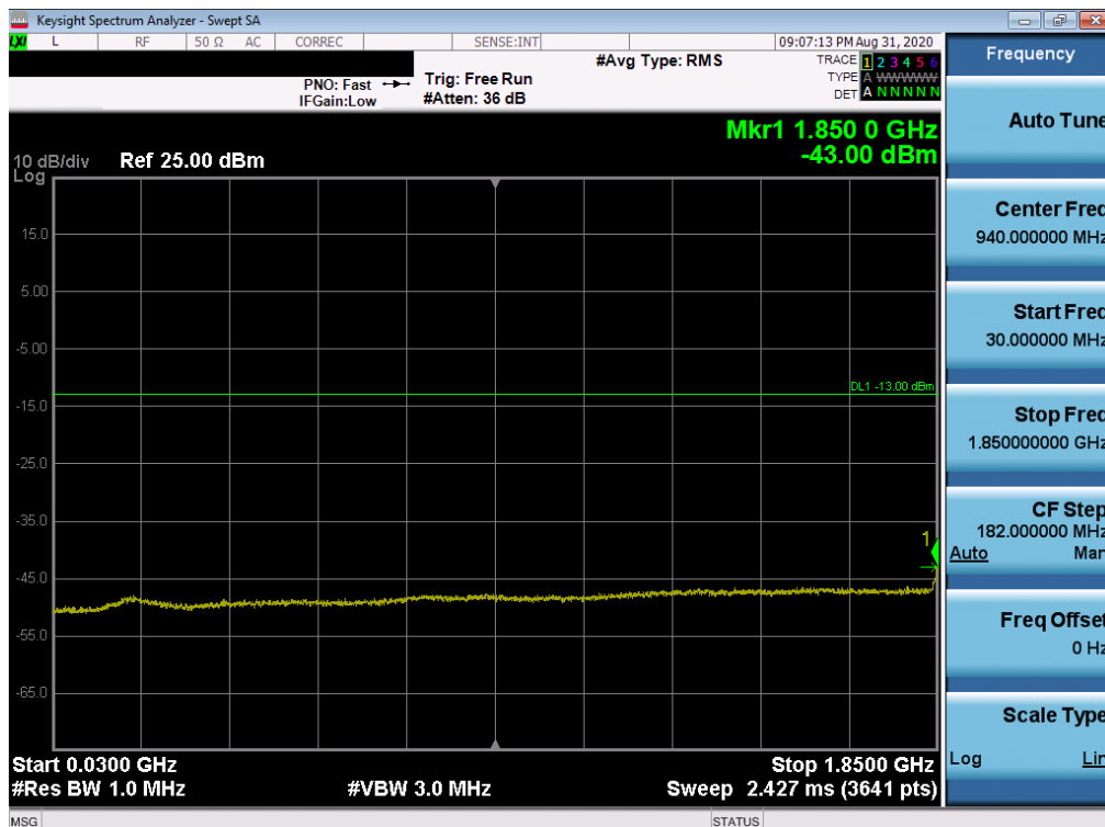
Plot 7-25. Conducted Spurious Plot (LTE Band 25/2 - 20MHz QPSK - RB Size 1, RB Offset 0 - Mid Channel)
