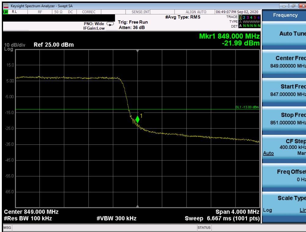
Plot 7-33. Upper Band Edge Plot (LTE Band 26/5 - 5MHz QPSK – Full RB Configuration)
