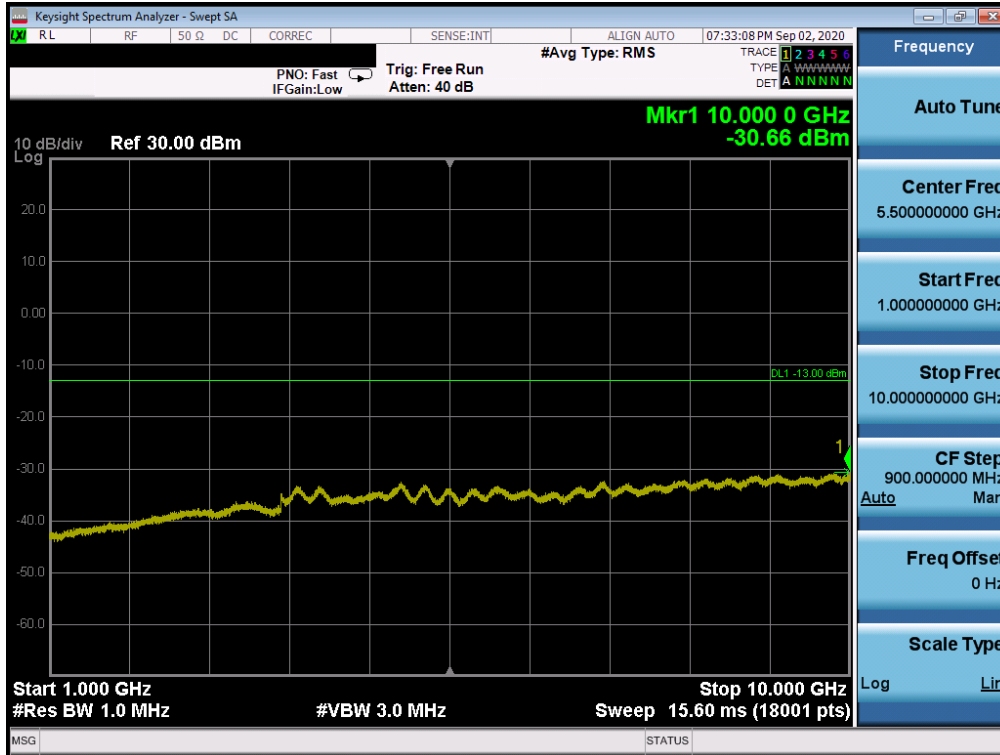
Plot 7-21. Conducted Spurious Plot (LTE Band 26/5 - 10MHz QPSK - RB Size 1, RB Offset 0 - Low Channel)
