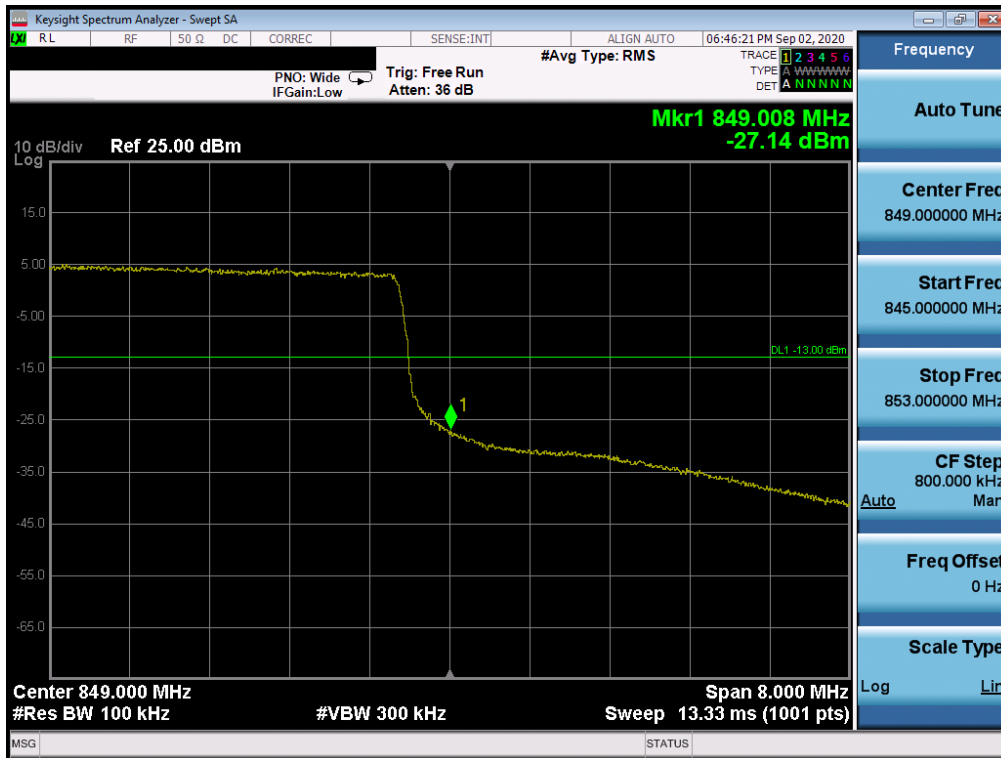
Plot 7-31. Upper Band Edge Plot (LTE Band 26/5 - 10MHz QPSK – Full RB Configuration)
