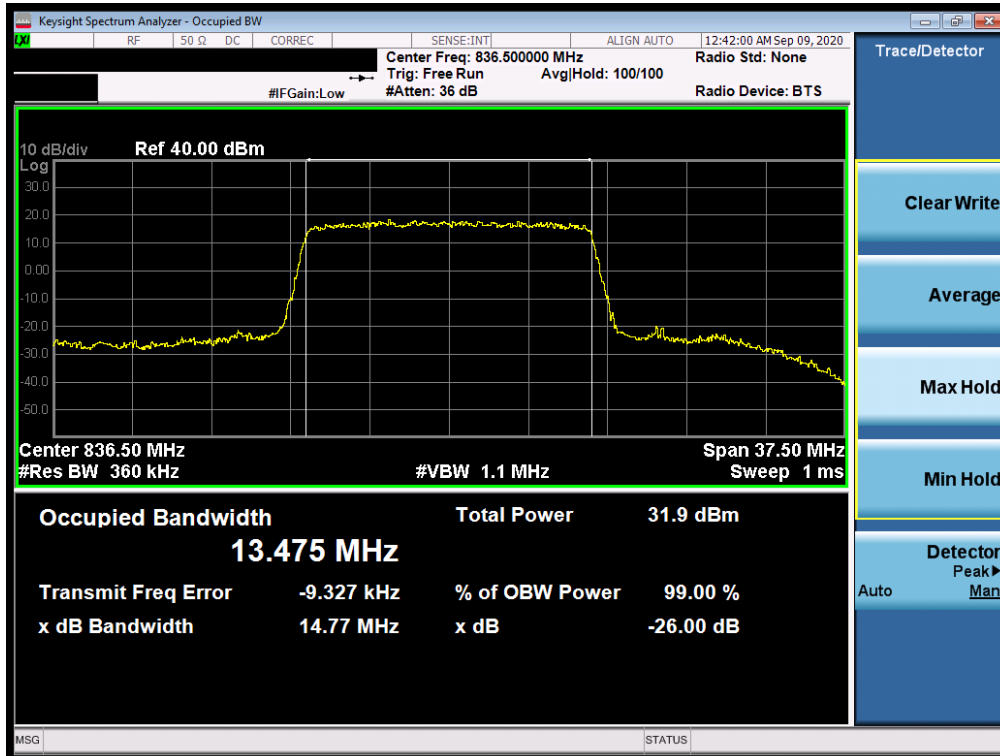
Plot 7-1. Occupied Bandwidth Plot (LTE Band 26 - 15MHz QPSK - Full RB Configuration)
