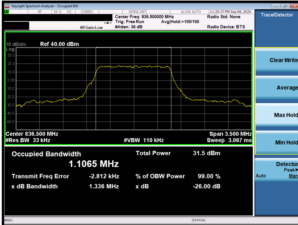
Plot 7-13. Occupied Bandwidth Plot (LTE Band 26/5 - 1.4MHz QPSK - Full RB Configuration)
