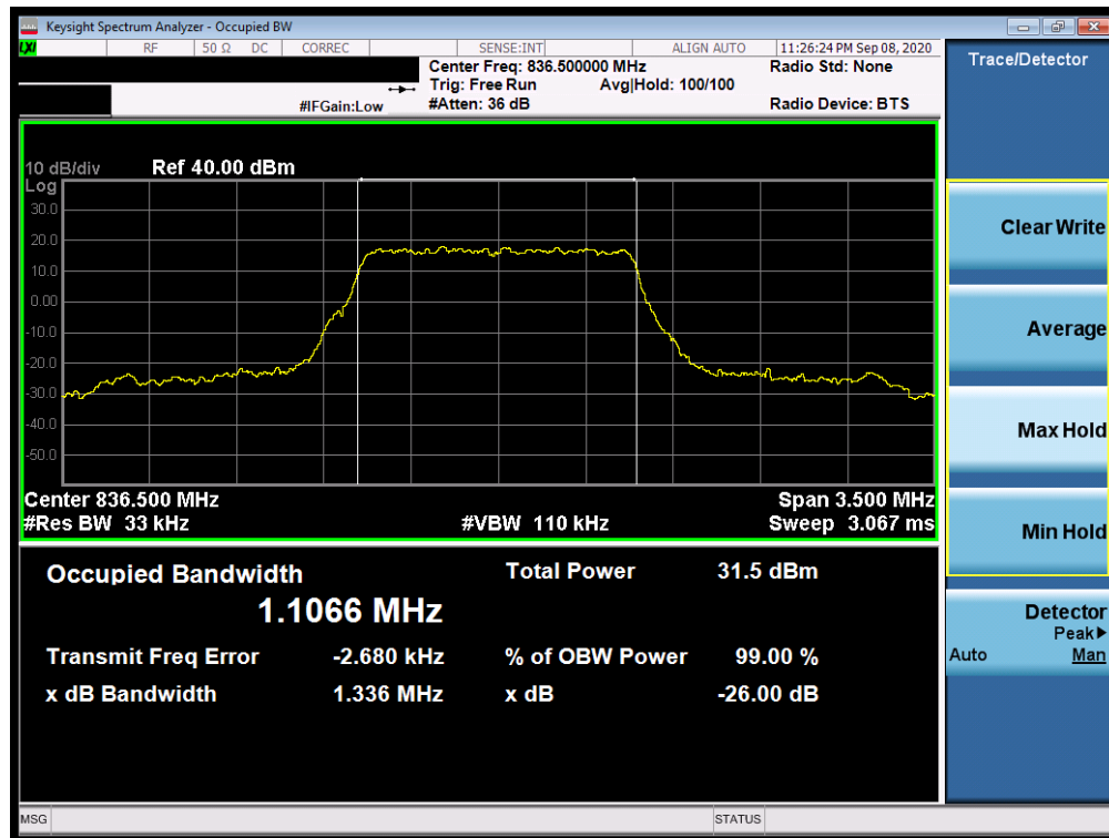
Plot 7-14. Occupied Bandwidth Plot (LTE Band 26/5 - 1.4MHz 16-QAM - Full RB Configuration)
