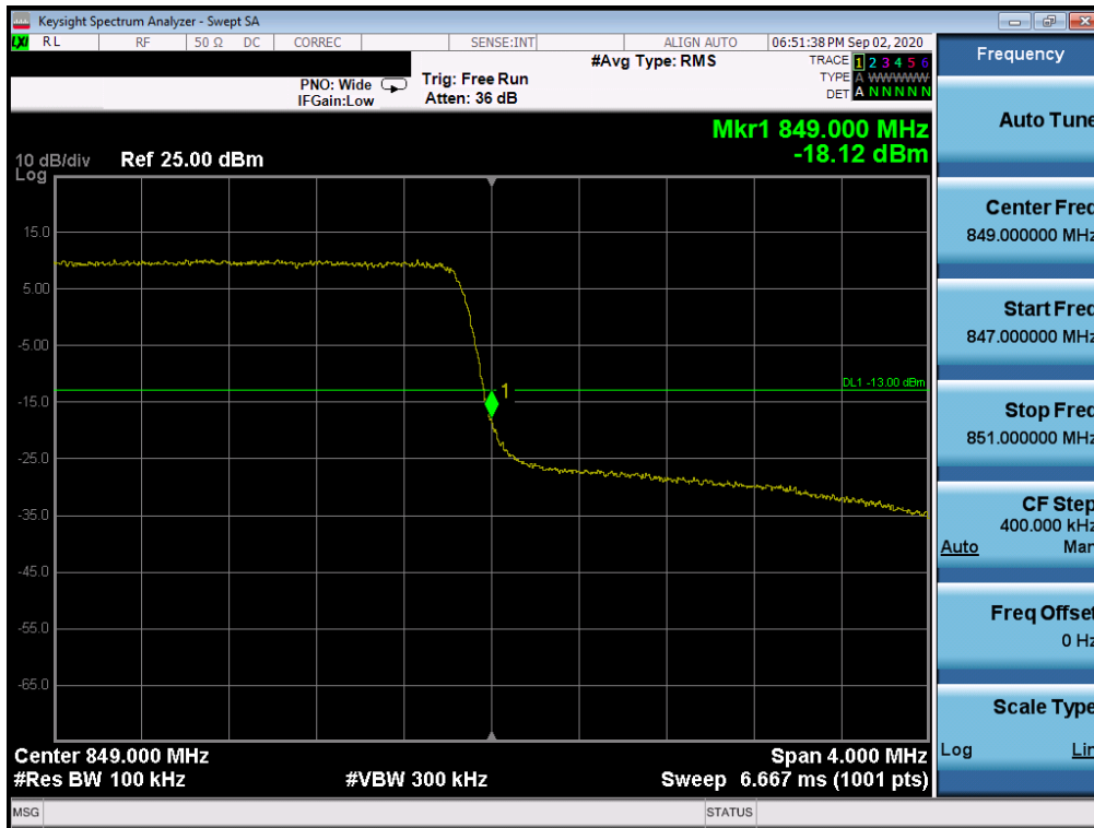
Plot 7-35. Upper Band Edge Plot (LTE Band 26/5 - 3MHz QPSK – Full RB Configuration)
