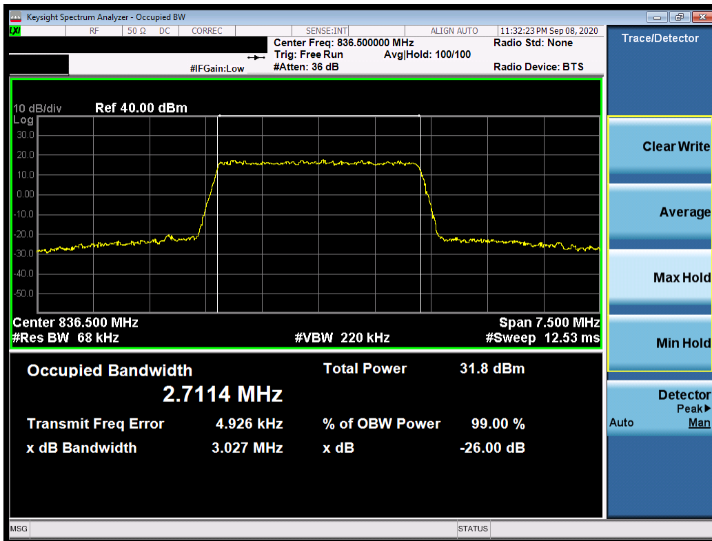
Plot 7-10. Occupied Bandwidth Plot (LTE Band 26/5 - 3MHz QPSK - Full RB Configuration)
