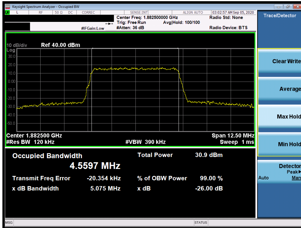
Plot 7-11. Occupied Bandwidth Plot (LTE Band 25/2 - 5MHz 16-QAM - Full RB Configuration)
