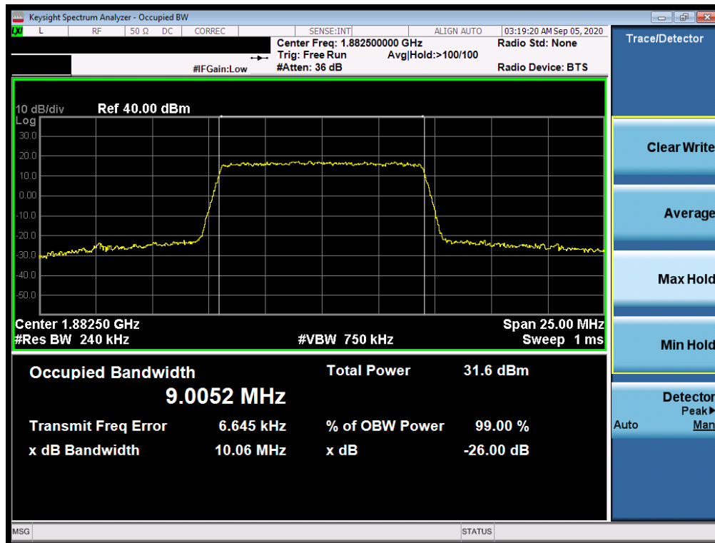
Plot 7-7. Occupied Bandwidth Plot (LTE Band 25/2 - 10MHz QPSK - Full RB Configuration)
