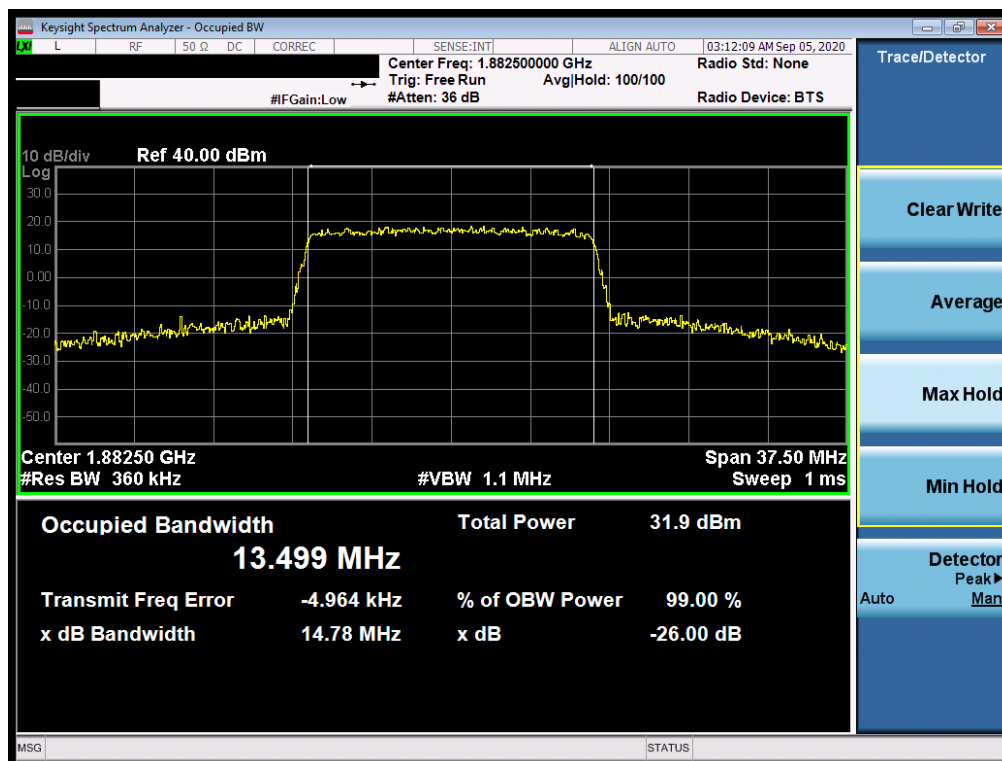
Plot 7-6. Occupied Bandwidth Plot (LTE Band 25/2 - 15MHz 64-QAM - Full RB Configuration)
