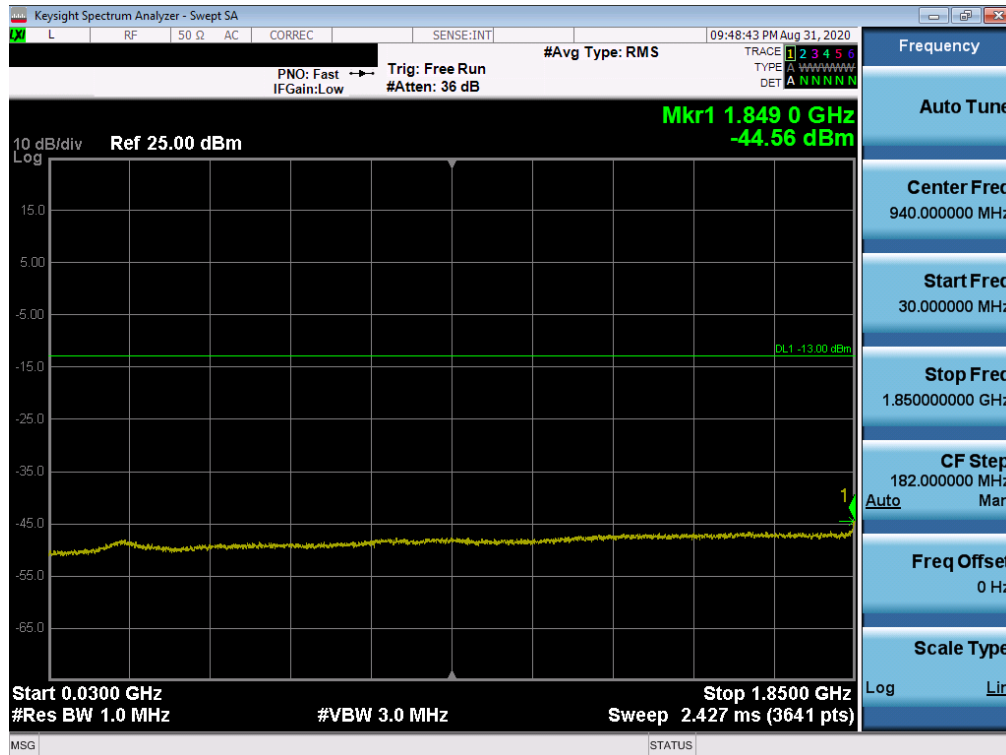
Plot 7-29. Conducted Spurious Plot (LTE Band 25/2 - 20MHz QPSK - RB Size 1, RB Offset 0 - High Channel)
