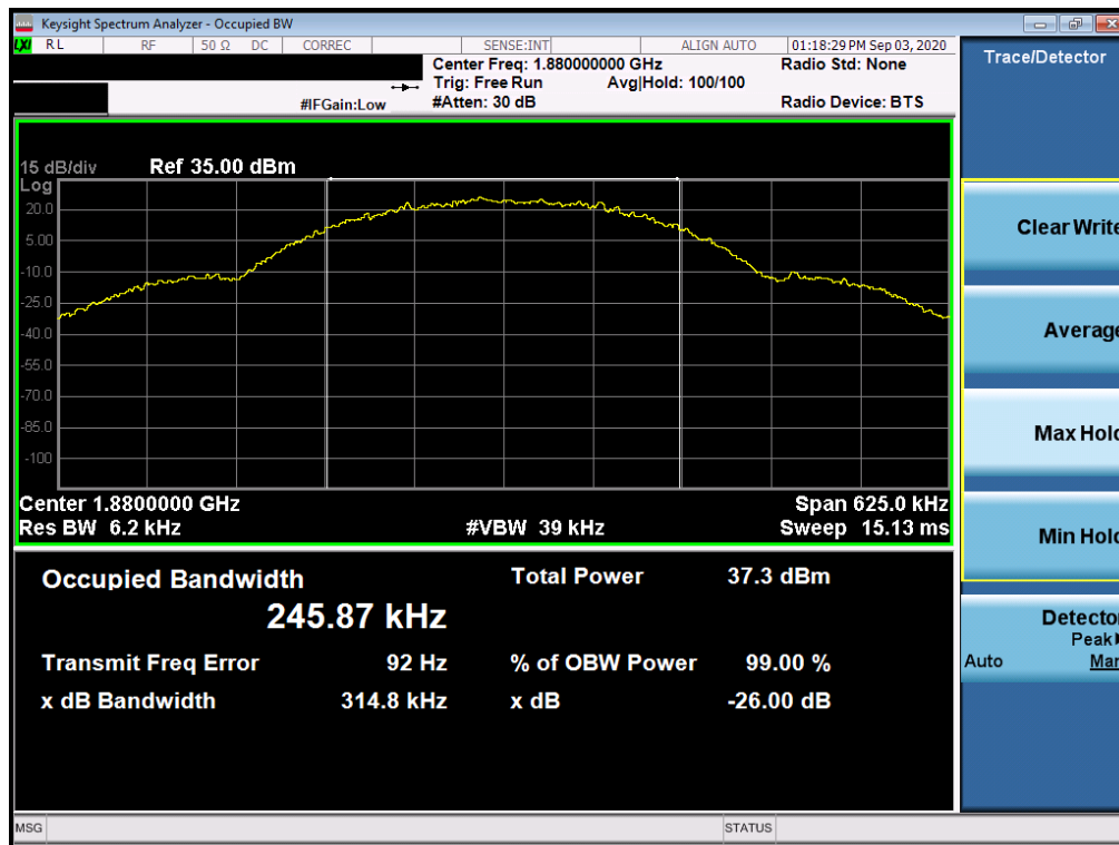
Plot 7-19. Occupied Bandwidth Plot (GPRS, Ch. 661)
