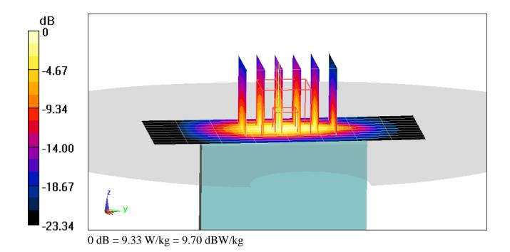
DUT: ZNFK200QM; Type: Portable Handset; Serial: 00277
