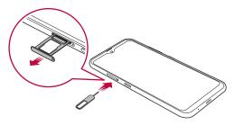
2 Place the SIM card or memory card on the card tray and then insert the card tray into the device in the direction of the arrow.
