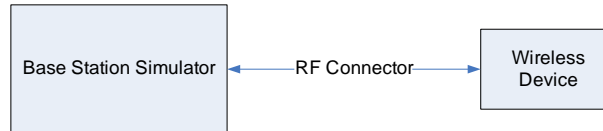
Figure 9-4 Power Measurement Setup
