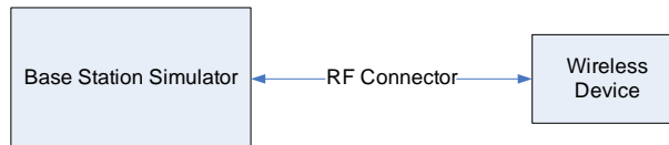
Figure 9-3 Power Measurement Setup
