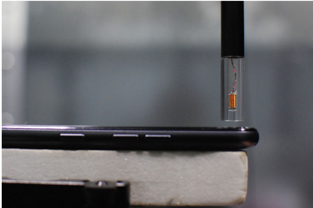
Figure 15-2 Test Setup for Wireless Device
