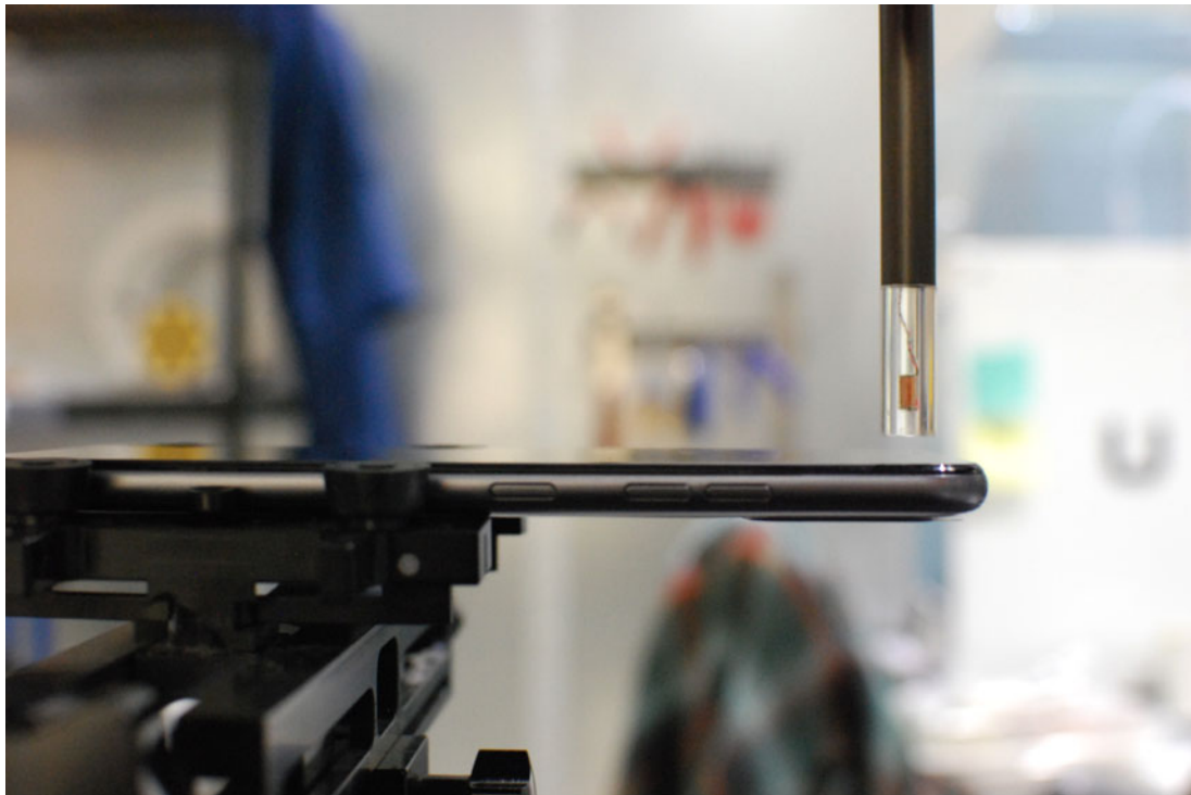
Figure 16-2 Test Setup for Wireless Device
