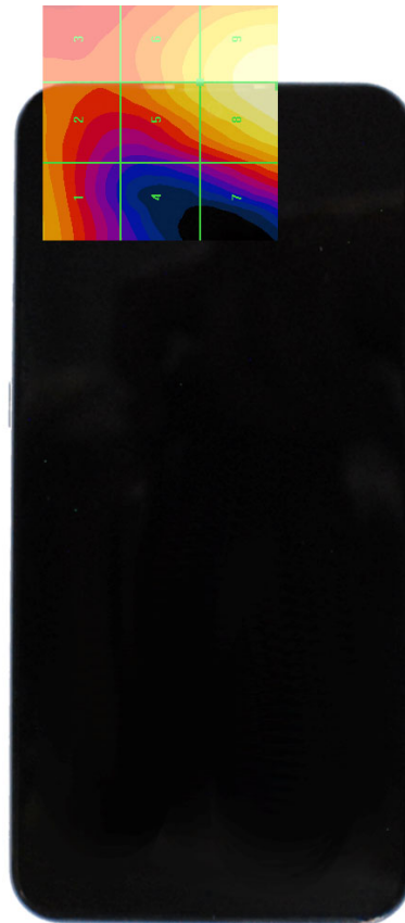
Figure 17-3 5x5 Scan grid above WD (Acoustic scan area pictured)
