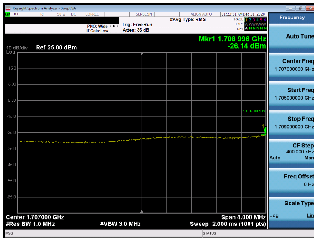
Plot 7-64. Lower Extended Band Edge Plot (LTE Band 4 - 15MHz QPSK – Full RB Configuration)
