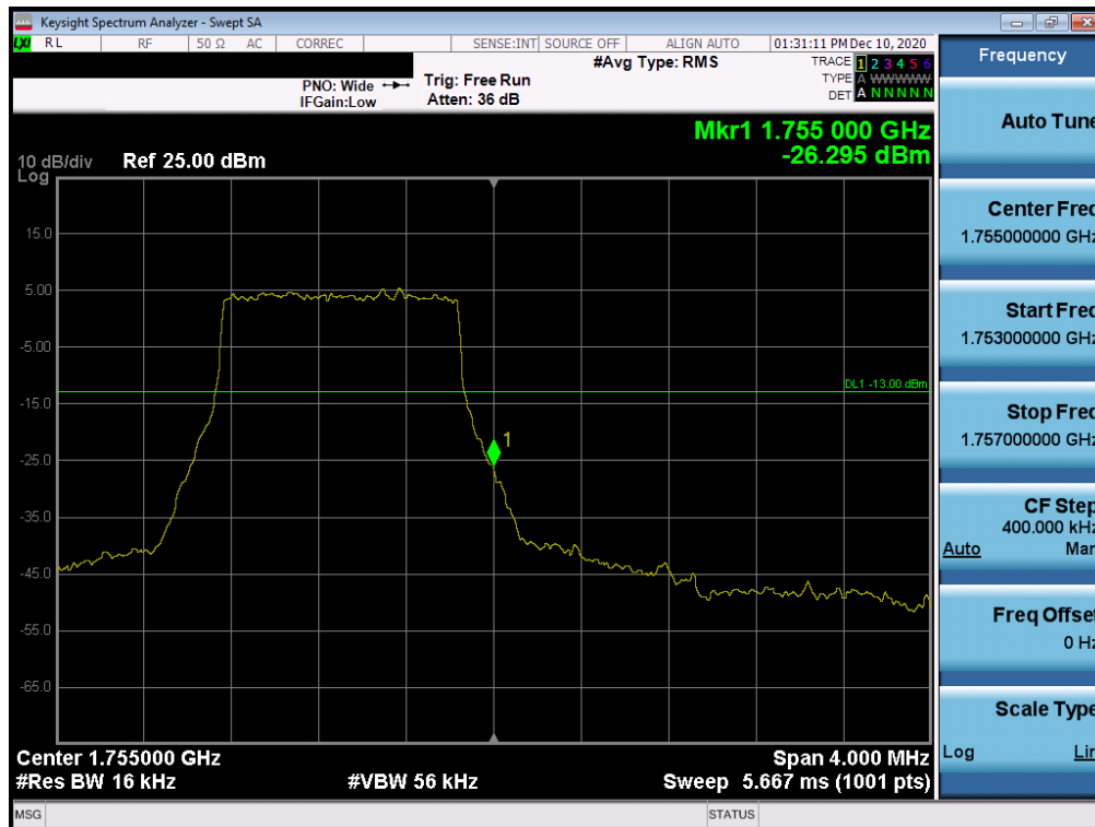
Plot 7-81. Upper Band Edge Plot (LTE Band 4 – 1.4MHz QPSK – Full RB Configuration)
