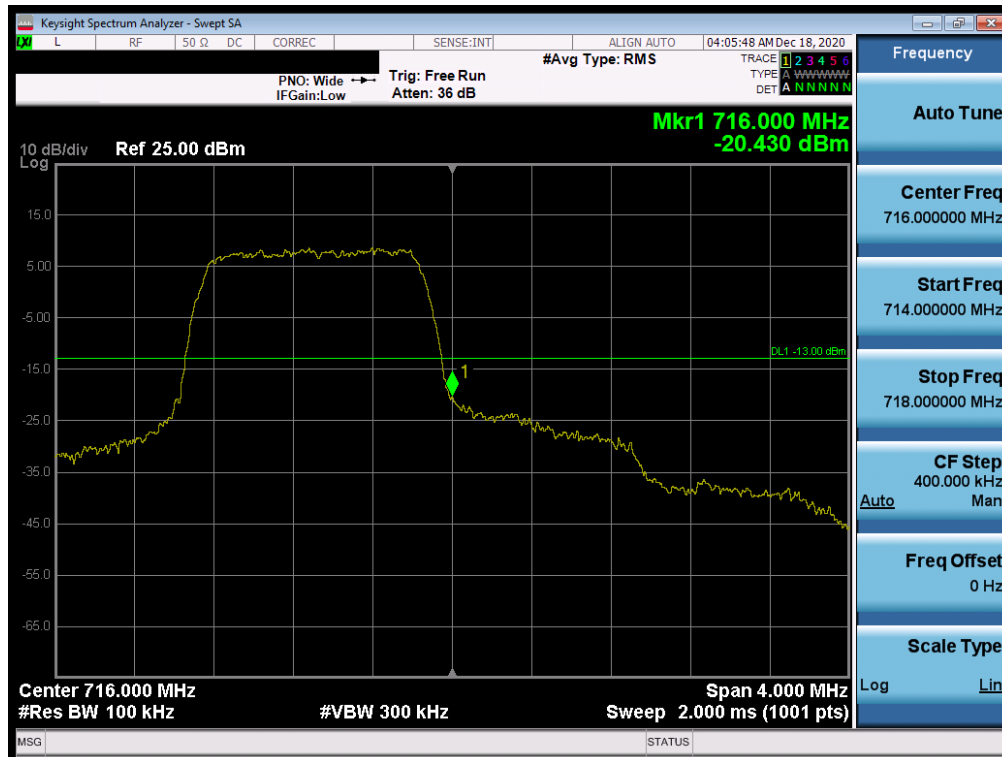
Plot 7-97. Upper Band Edge Plot (LTE Band 12 – 1.4MHz QPSK – Full RB Configuration)
