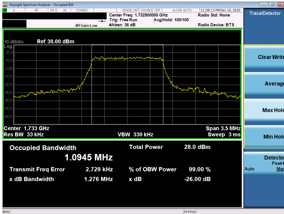
Plot 7-18. Occupied Bandwidth Plot (LTE Band 4 - 1.4MHz 64-QAM - Full RB Configuration)
