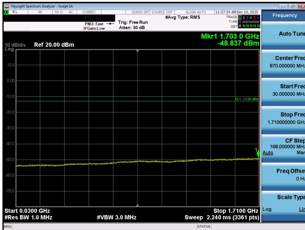
Plot 7-38. Conducted Spurious Plot (LTE Band 4 - 20MHz QPSK - RB Size 1, RB Offset 0 - High Channel)
