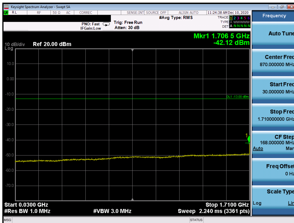
Plot 7-35. Conducted Spurious Plot (LTE Band 4 - 20MHz QPSK - RB Size 1, RB Offset 0 - Mid Channel)
