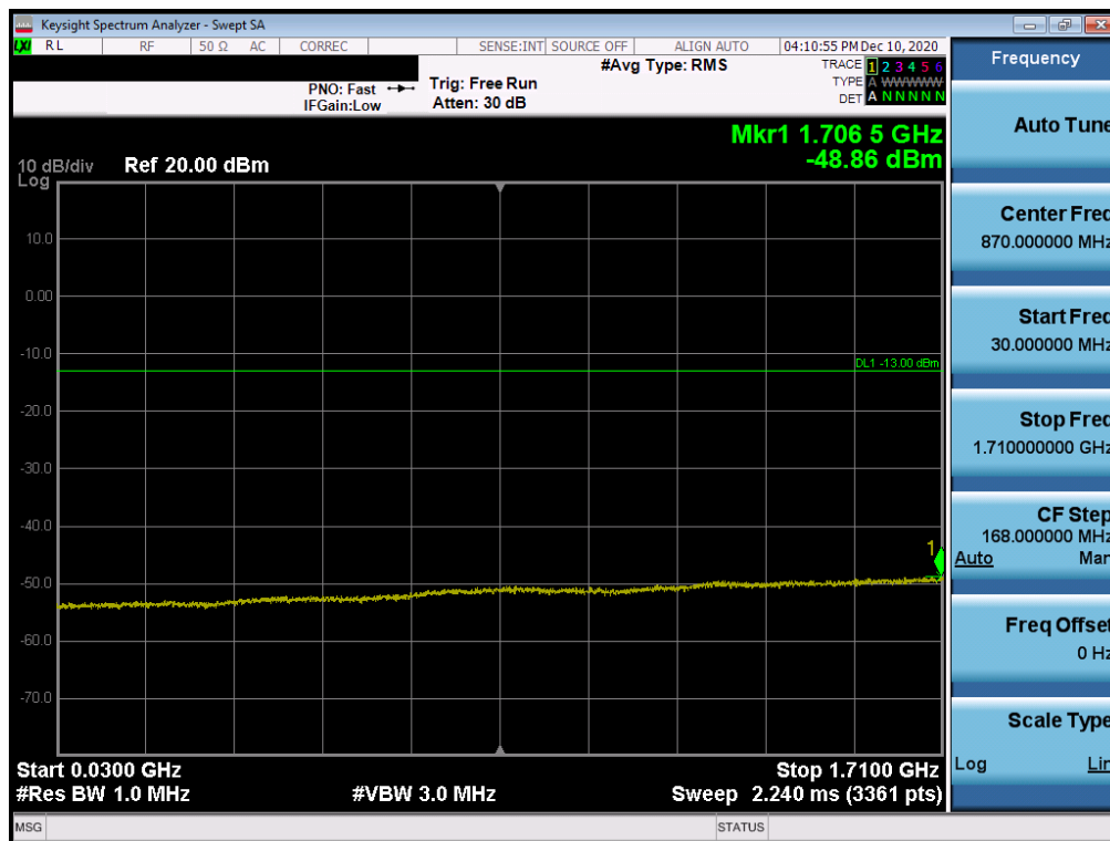
Plot 7-53. Conducted Spurious Plot (WCDMA Ch. 1413- Mid Channel)
