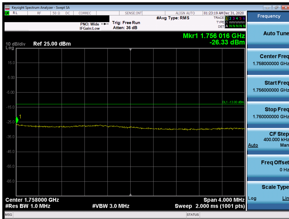
Plot 7-66. Upper Extended Band Edge Plot (LTE Band 4 - 15MHz QPSK – Full RB Configuration)
