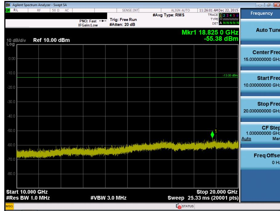
BAND 4. Conducted Spurious Plot\_1 (20175ch\_5MHz\_QPSK\_RB 1\_0)
