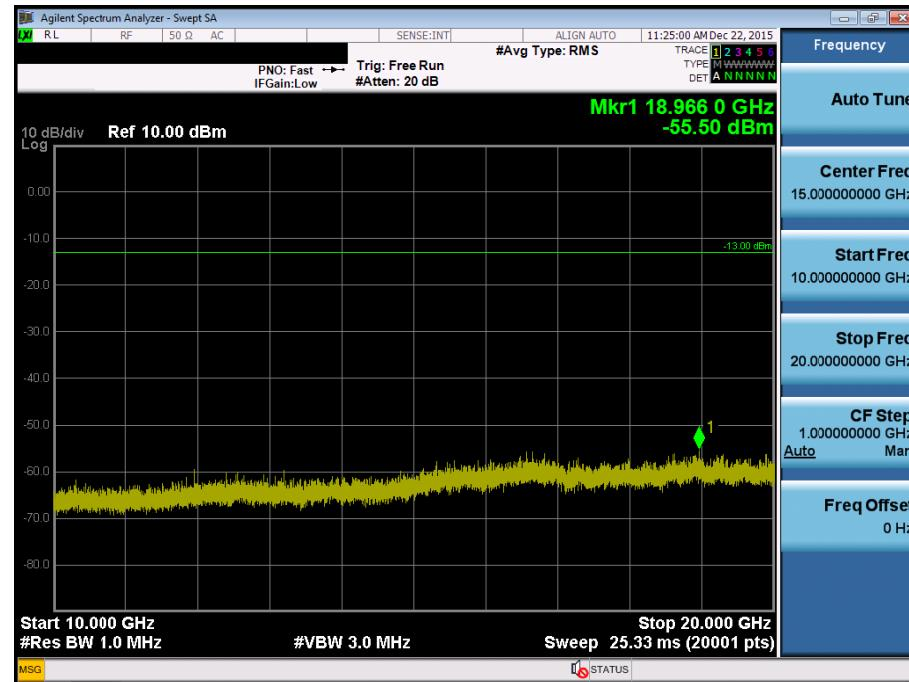
BAND 4. Conducted Spurious Plot\_1 (20385ch\_3MHz\_QPSK\_RB 1\_0)
