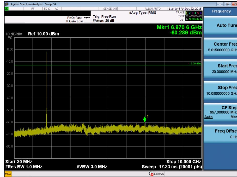
BAND 4. Conducted Spurious Plot\_2 (20350ch\_10MHz\_QPSK\_RB 1\_0)
