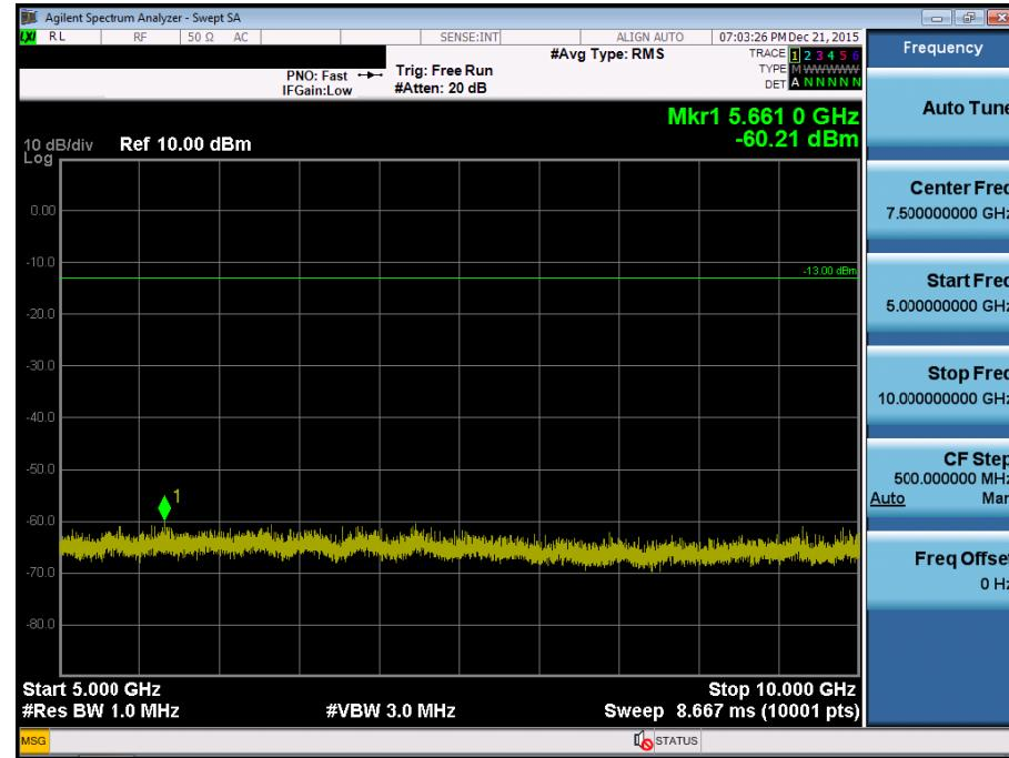
BAND 17. Conducted Spurious Plot\_1 (23790ch\_10MHz\_QPSK\_RB 1\_0)
