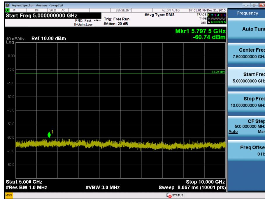
BAND 17. Conducted Spurious Plot\_1 (23790ch\_5MHz\_QPSK\_RB 1\_0)
