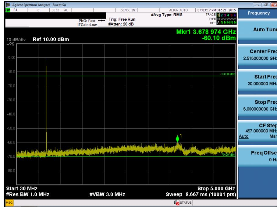
BAND 17. Conducted Spurious Plot\_2 (23780ch\_10MHz\_QPSK\_RB 1\_0)
