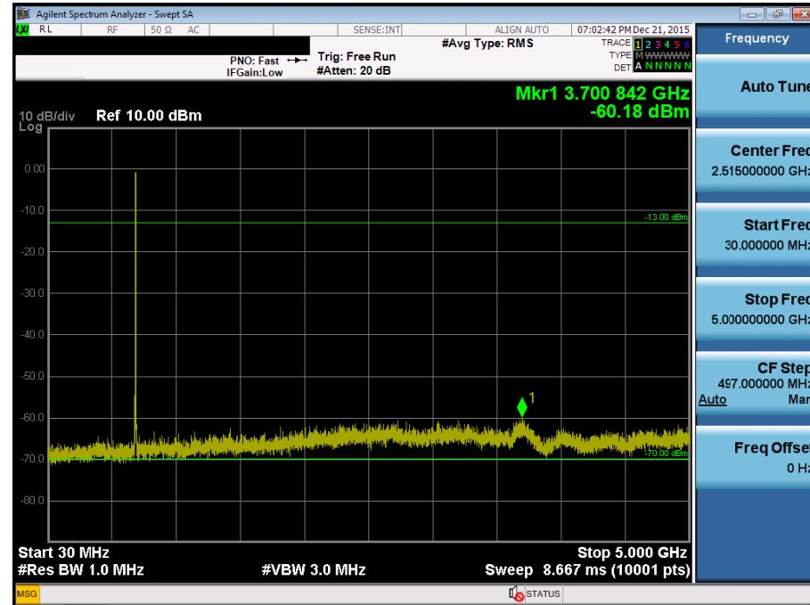
BAND 17. Conducted Spurious Plot\_2 (23825ch\_5MHz\_QPSK\_RB 1\_0)
