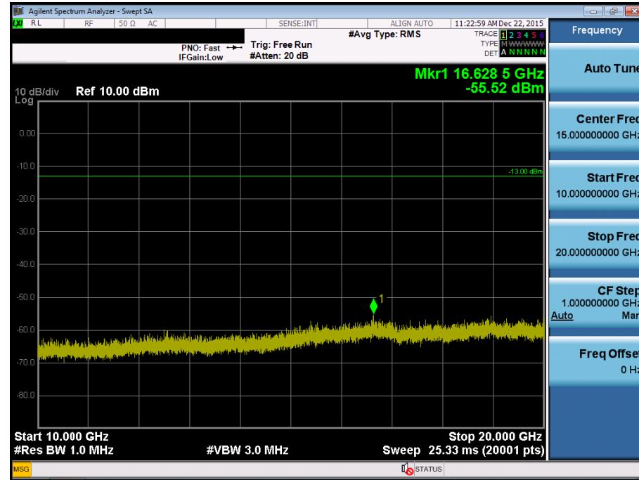
BAND 4. Conducted Spurious Plot\_1 (19965ch\_3MHz\_QPSK\_RB 1\_0)
