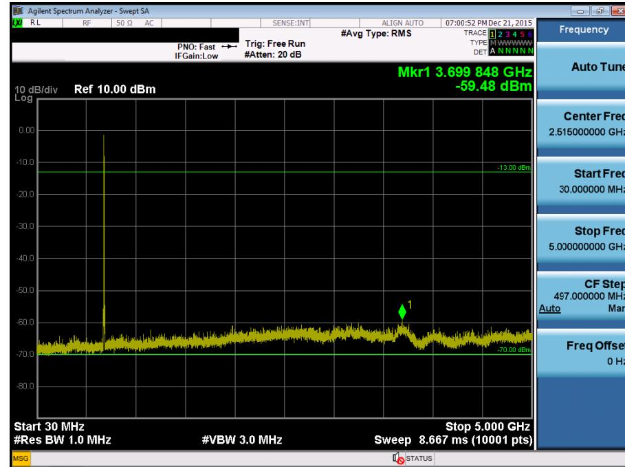
BAND 17. Conducted Spurious Plot\_2 (23755ch\_5MHz\_QPSK\_RB 1\_0)
