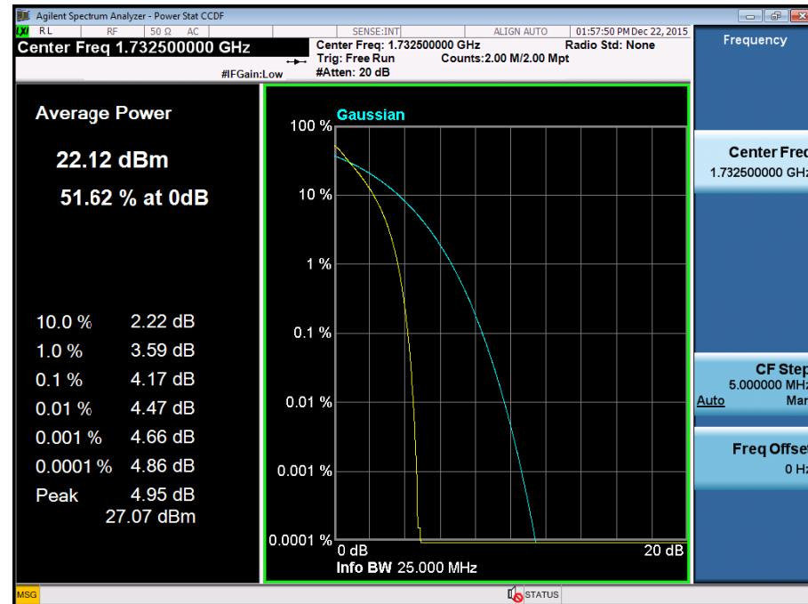
BAND 4. PAR Plot (15M BW\_Ch.20175\_16QAM\_RB75\_0)
