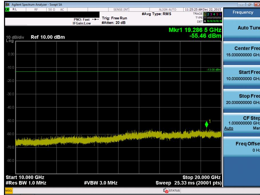
BAND 4. Conducted Spurious Plot\_1 (19975ch\_5MHz\_QPSK\_RB 1\_0)
