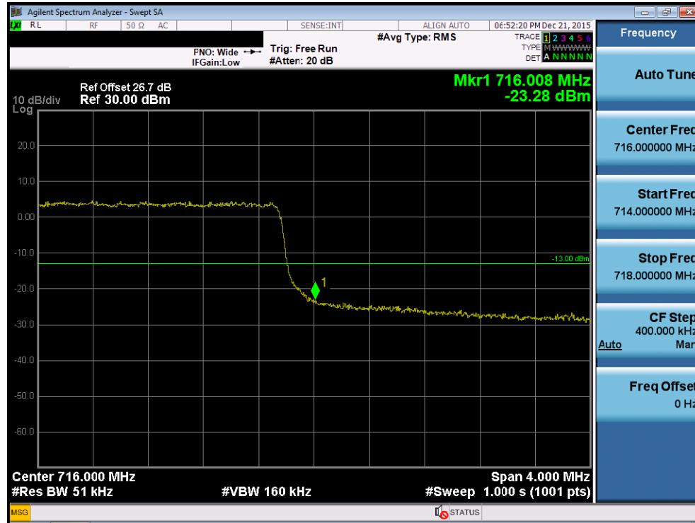
Band 17 Upper Extended Band Edge Plot (5M BW Ch.23825 QPSK\_RB25\_0)
