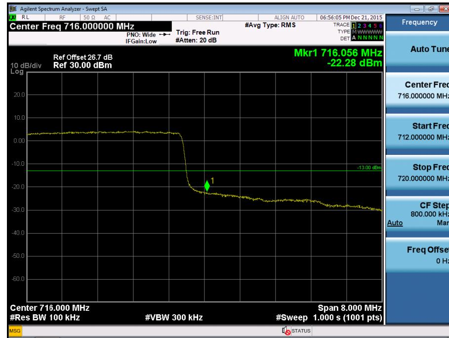
Band 17 Upper Extended Band Edge Plot (10M BW Ch.23800 QPSK\_RB50\_0)
