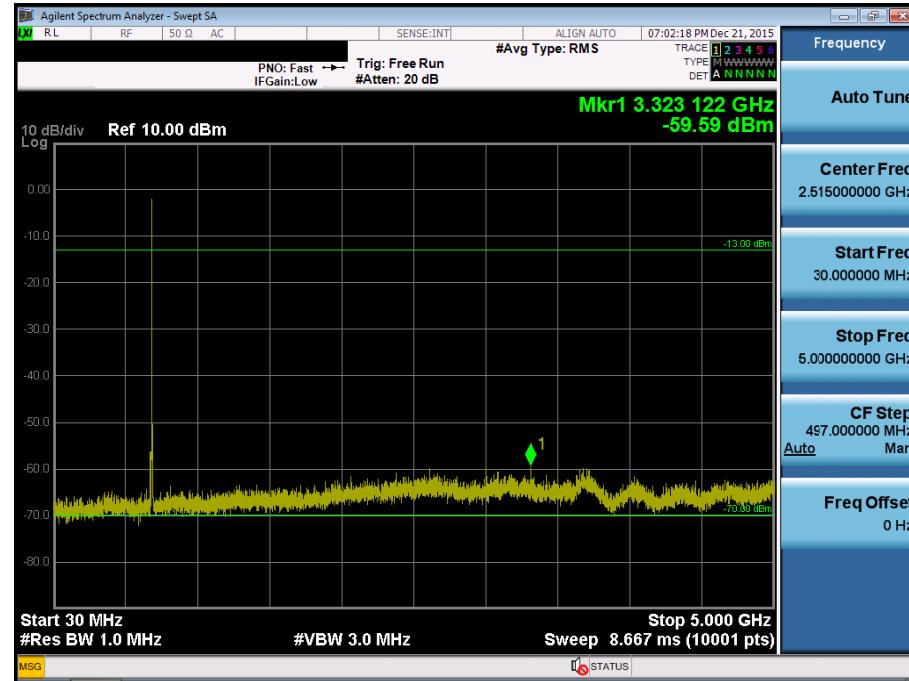
BAND 17. Conducted Spurious Plot\_2 (23790ch\_5MHz\_QPSK\_RB 1\_0)
