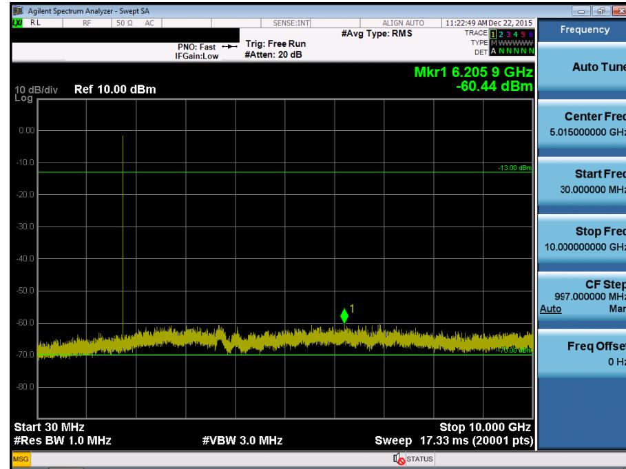
BAND 4. Conducted Spurious Plot\_2 (20393ch\_1.4MHz\_QPSK\_RB 1\_0)
