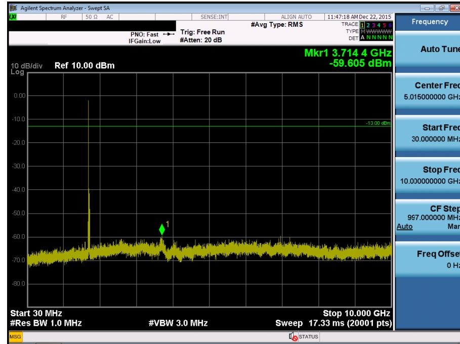
BAND 4. Conducted Spurious Plot\_2 (20050ch\_20MHz\_QPSK\_RB 1\_0)
