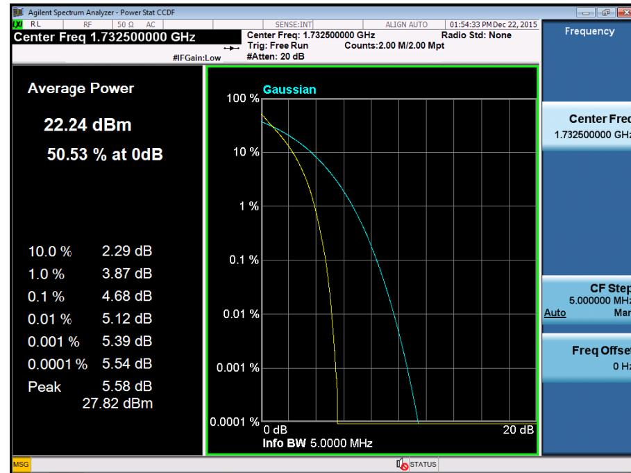
BAND 4. PAR Plot (5M BW\_Ch.20175\_16QAM\_RB25\_0)
