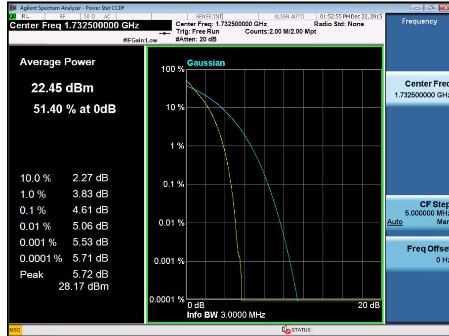
BAND 4. PAR Plot (3M BW\_Ch.20175\_16QAM\_RB15\_0)
