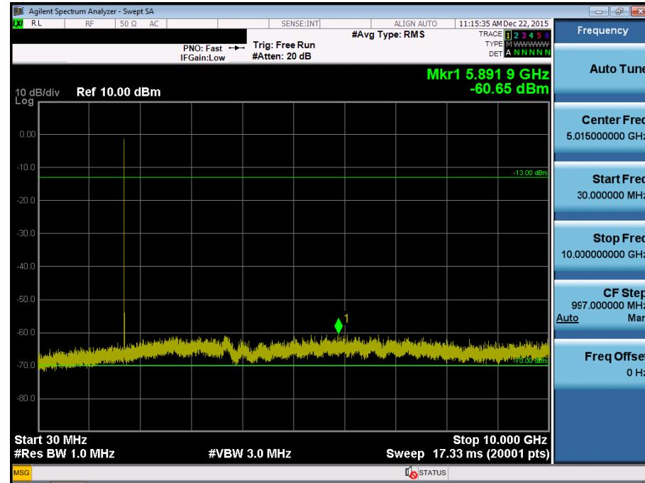
BAND 4. Conducted Spurious Plot\_2 (19957ch\_1.4MHz\_QPSK\_RB 1\_0)
