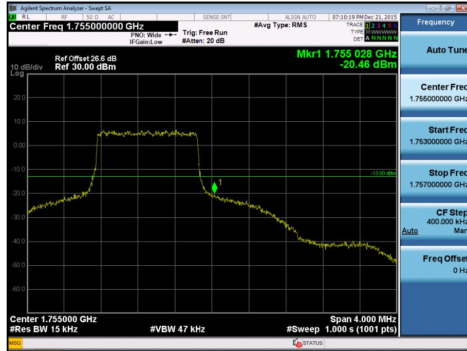
BAND 4. Upper Extended Band Edge Plot (1.4M BW Ch. 20393 QPSK\_RB6\_0) -3
