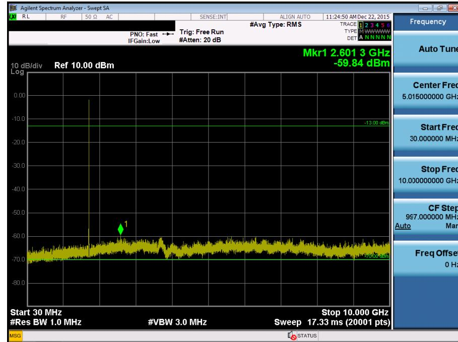
BAND 4. Conducted Spurious Plot\_2 (20175ch\_3MHz\_QPSK\_RB 1\_0)
