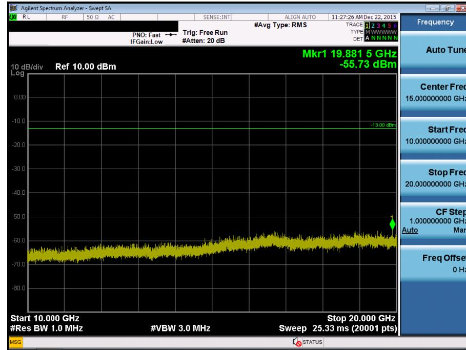
BAND 4. Conducted Spurious Plot\_1 (20375ch\_5MHz\_QPSK\_RB 1\_0)
