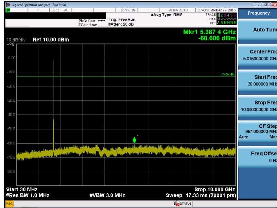
BAND 4. Conducted Spurious Plot\_2 (20025ch\_15MHz\_QPSK\_RB 1\_0)
