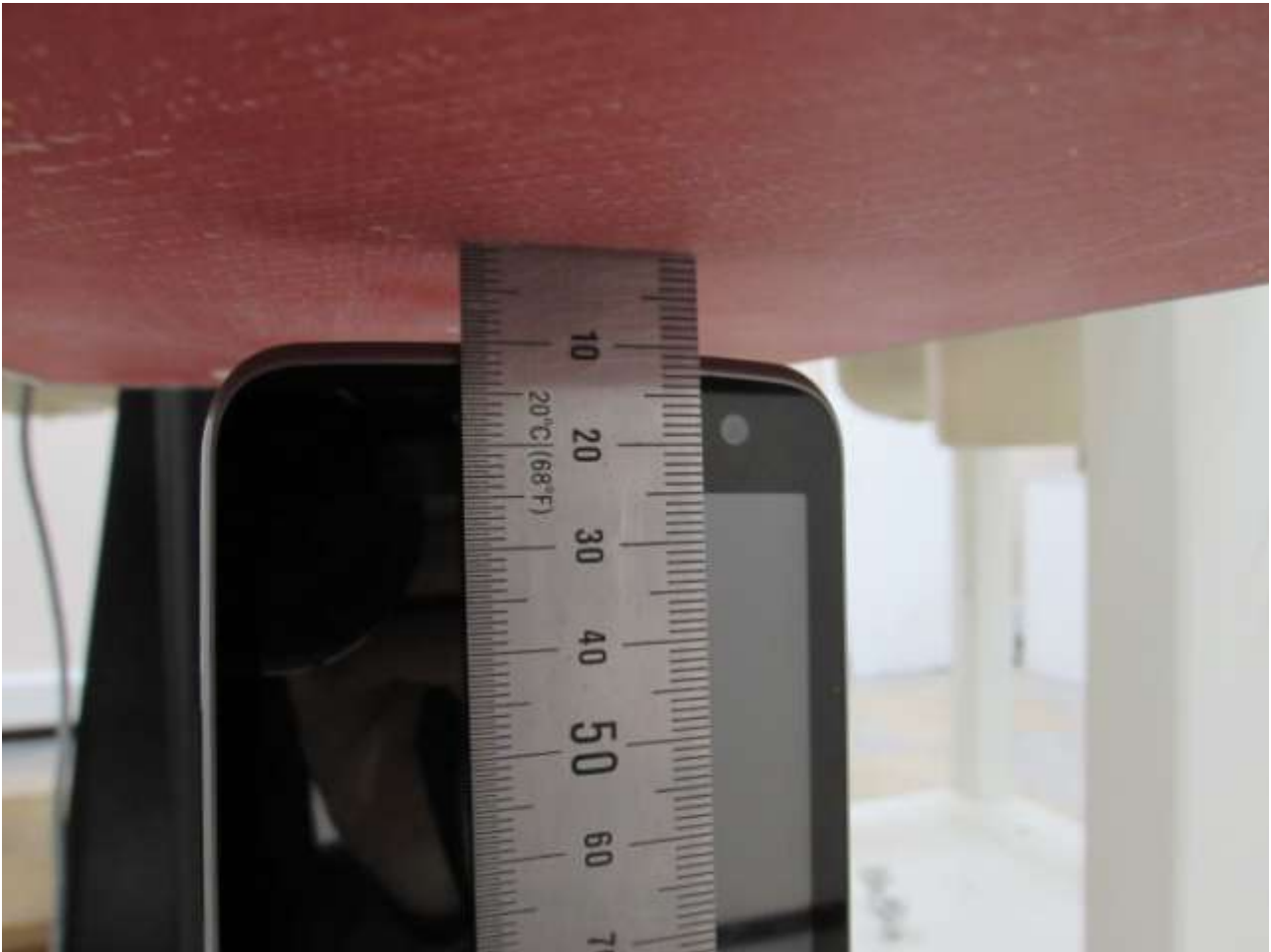
[Distance of 1.0 cm from the EUT]
