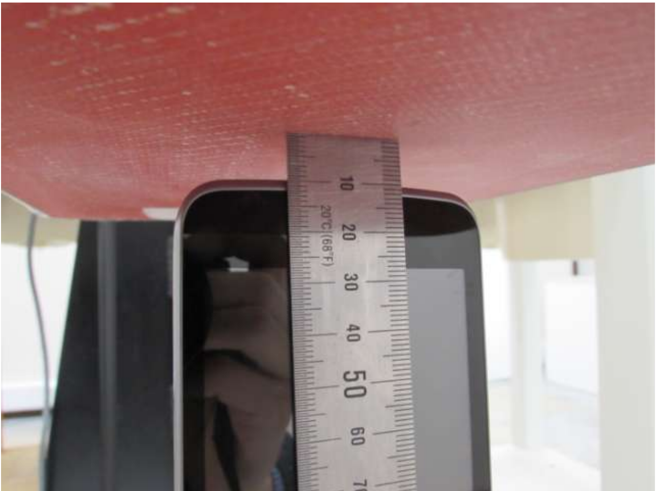
[Distance of 1.0 cm from the EUT]
