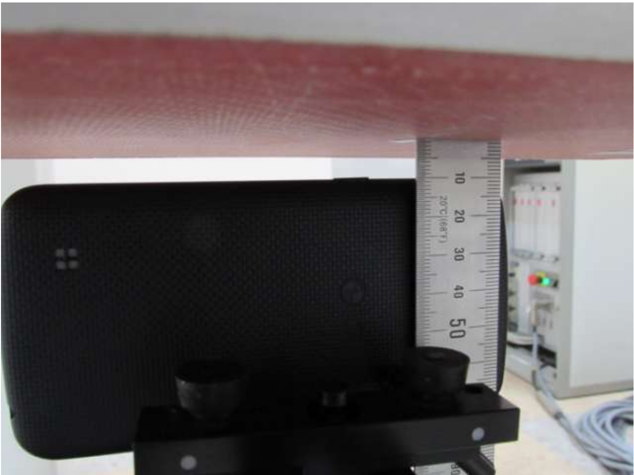
[Distance of 1.0 cm from the EUT]
