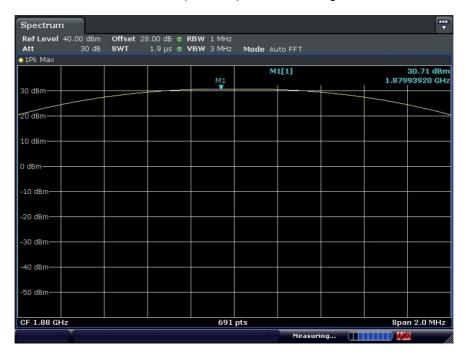
■ GSM1900 MODE (661 CH.) Peak-to-Average Ratio P<sub>Avq</sub>
