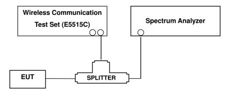
(Configuration of conducted Emission measurement)
