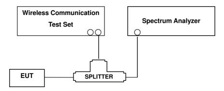
(Configuration of conducted Emission measurement)
