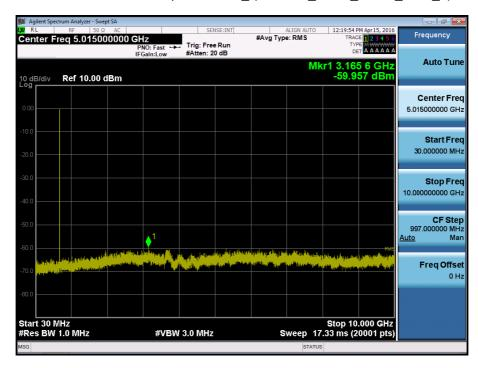
BAND 17. Conducted Spurious Plot\_ (23790ch\_5MHz\_QPSK\_RB 1\_0)
