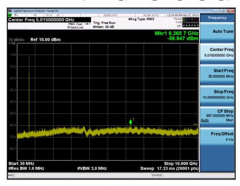
BAND 17. Conducted Spurious Plot\_ (23800ch\_10MHz\_QPSK\_RB 1\_0)
