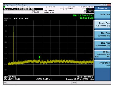
BAND 17. Conducted Spurious Plot\_ (23780ch\_10MHz\_QPSK\_RB 1\_0)
