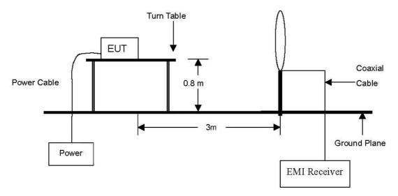
The diagram below shows the test setup that is utilized to make the measurements for emission from 30 Mz to 1  $\mathbb{G}$ .
