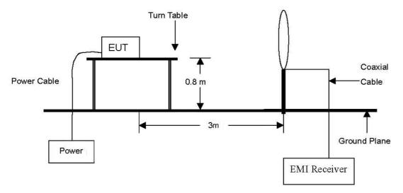
The diagram below shows the test setup that is utilized to make the measurements for emission from 30 Mz to 1  $\oplus$  Emissions.
