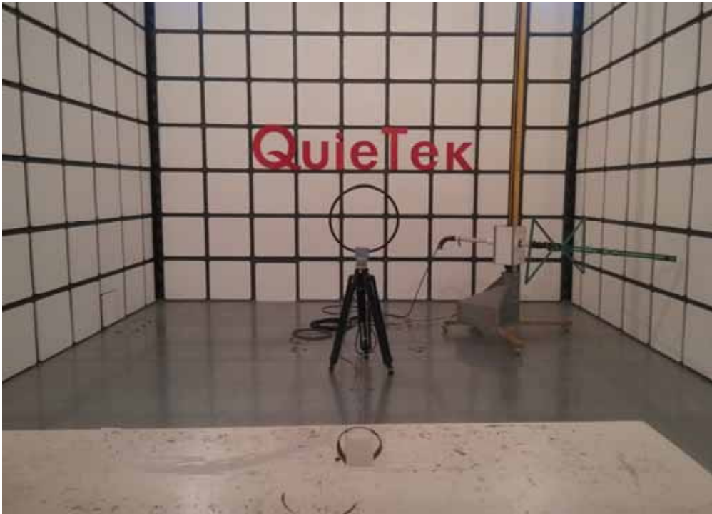
Description: Radiated Emission Test Setup for Below 30MHz
