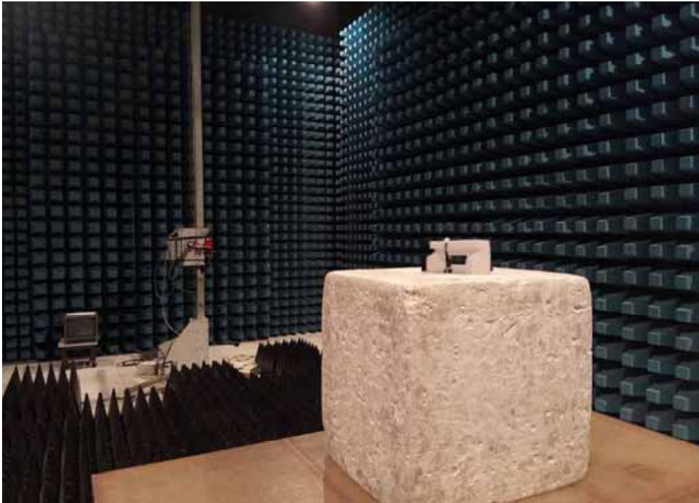
Description: Radiated Emission Test Setup for 1~18GHz
