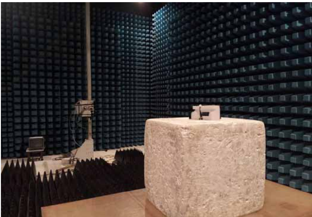
Description: Radiated Emission Test Setup for Above 18GHz
