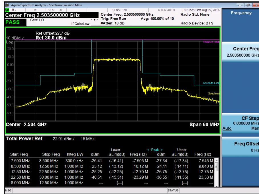
BAND 41. Mid Channel Edge Plot (15 MHz Ch.40620 QPSK RB 75)
