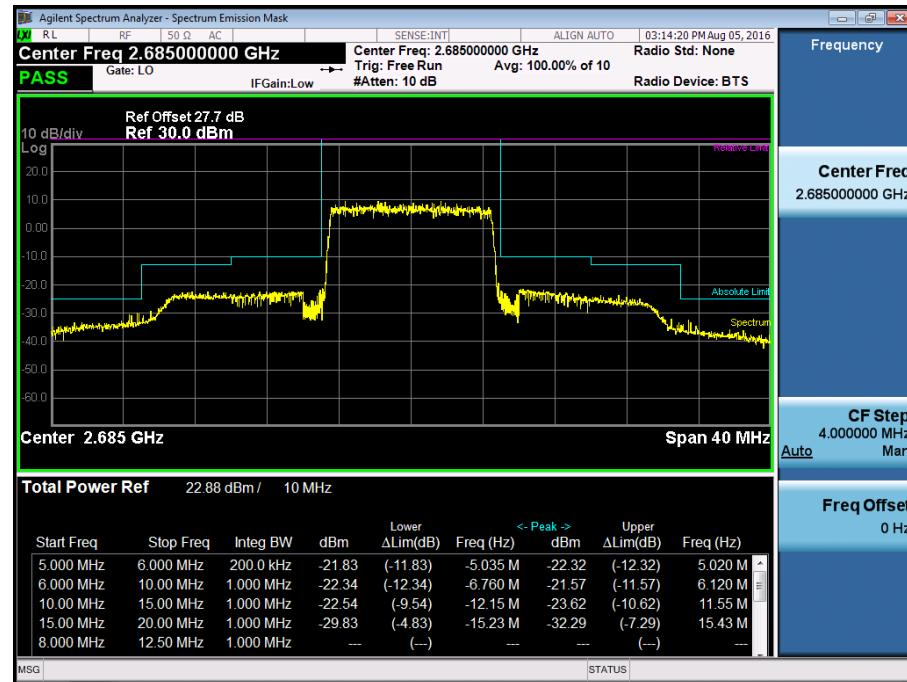
BAND 41. Low Channel Edge Plot (15 MHz Ch.39725 QPSK RB 75)
