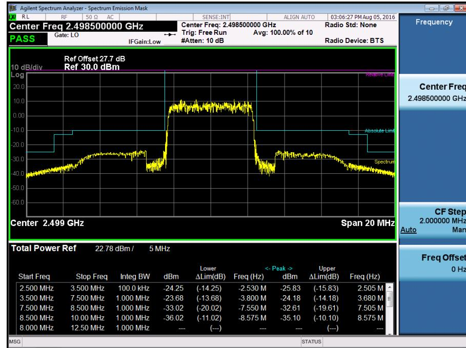
BAND 41. Mid Channel Edge Plot (5 MHz Ch.40620 QPSK RB 25)
