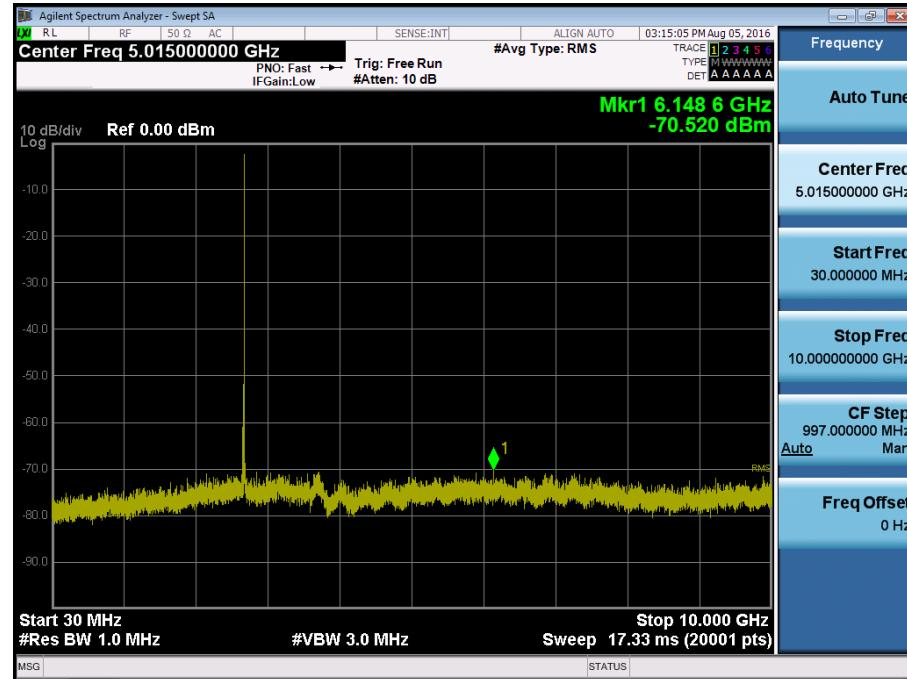
BAND 41. Conducted Spurious Plot 2 (10 MHz Ch. 41540 QPSK RB 1, Offset 0)
