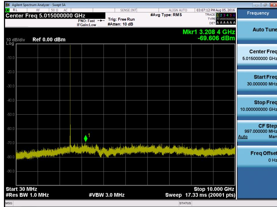
BAND 41. Conducted Spurious Plot 2 (5 MHz Ch. 39675 QPSK RB 1, Offset 0)
