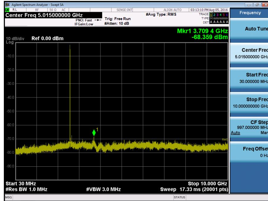
BAND 41. Conducted Spurious Plot 2 (10 MHz Ch. 40620 QPSK RB 1, Offset 0)
