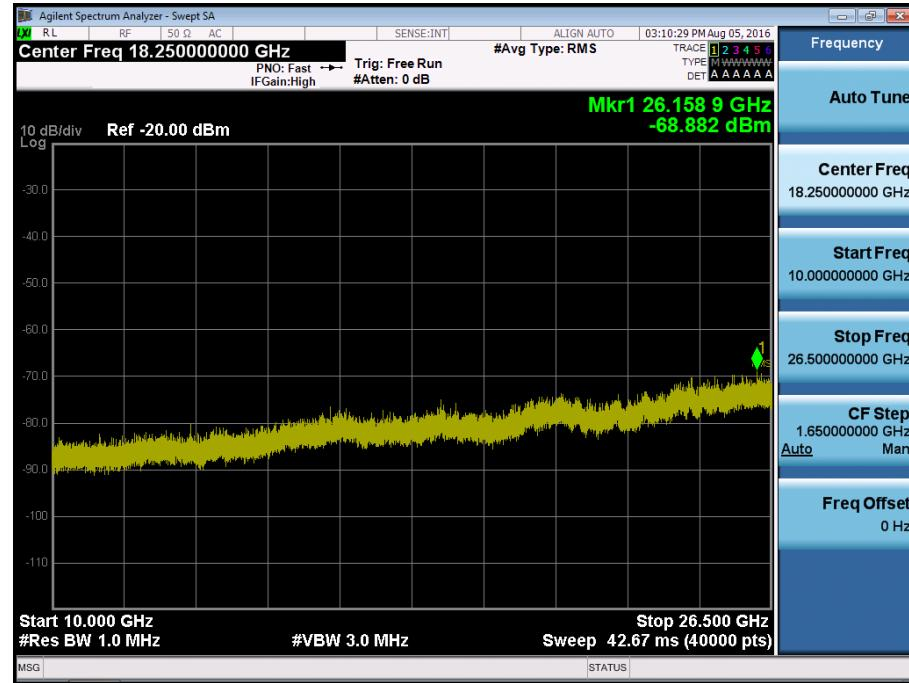
BAND 41. Conducted Spurious Plot 1 (10 MHz Ch.39700 QPSK RB 1, Offset 0)
