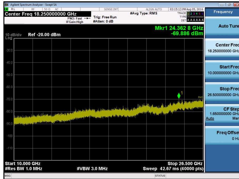
BAND 41. Conducted Spurious Plot 1 (15 MHz Ch.39725 QPSK RB 1, Offset 0)
