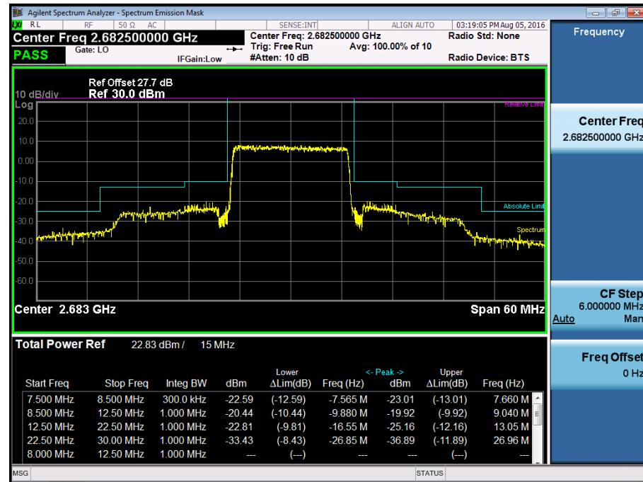
BAND 41. Low Channel Edge Plot (20 MHz Ch.39750 QPSK RB 100)
