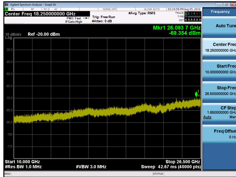
BAND 41. Conducted Spurious Plot 1 (20 MHz Ch.39750 QPSK RB 1, Offset 0)
