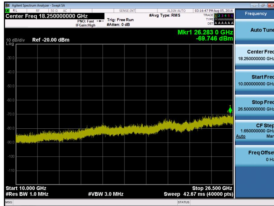
BAND 41. Conducted Spurious Plot 1 (15 MHz Ch.40620 QPSK RB 1, Offset 0)
