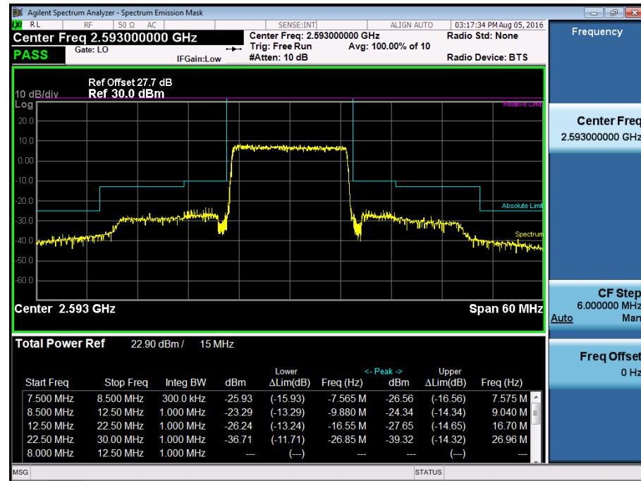
BAND 41. High Channel Edge Plot (15 MHz Ch.41515 QPSK RB 75)
