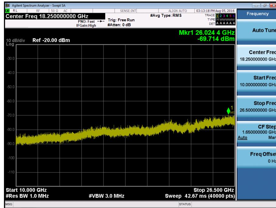
BAND 41. Conducted Spurious Plot 1 (10 MHz Ch.41540 QPSK RB 1, Offset 0)
