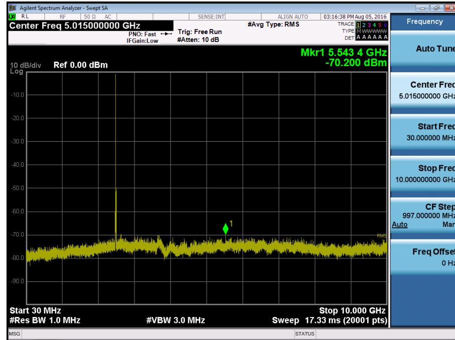
BAND 41. Conducted Spurious Plot 2 (15 MHz Ch. 39725 QPSK RB 1, Offset 0)
