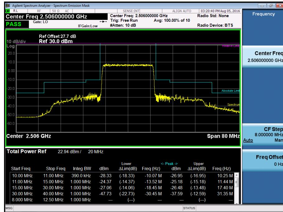
BAND 41. Mid Channel Edge Plot (20 MHz Ch.40620 QPSK RB 100)
