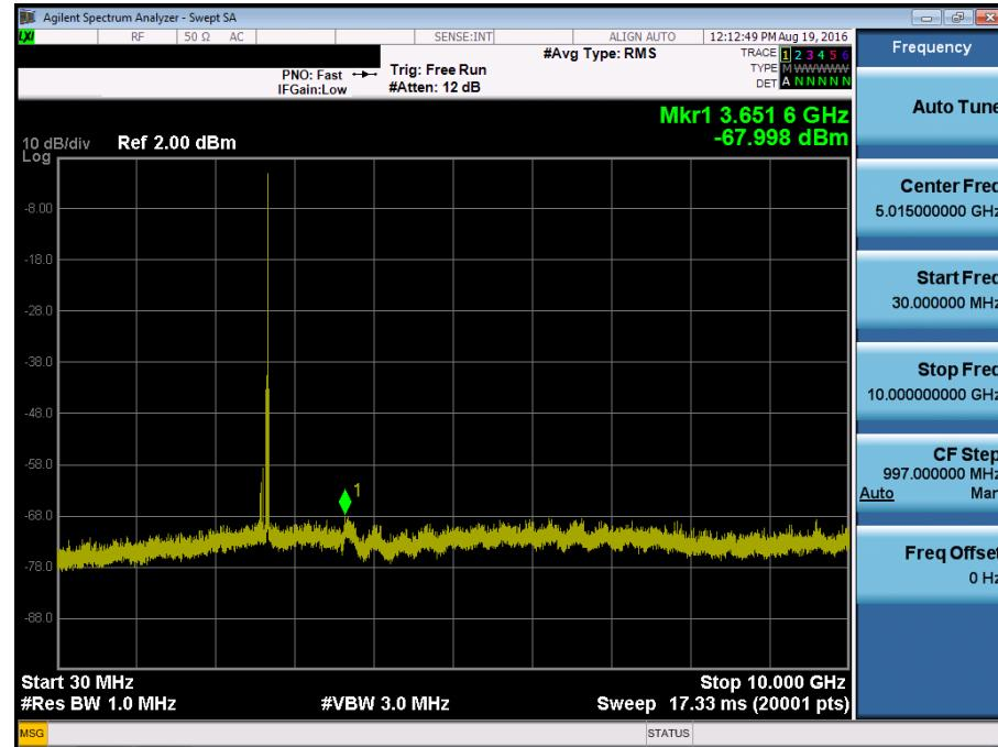
BAND 41. Conducted Spurious Plot 2 (15 MHz Ch. 41515 QPSK RB 1, Offset 0)
