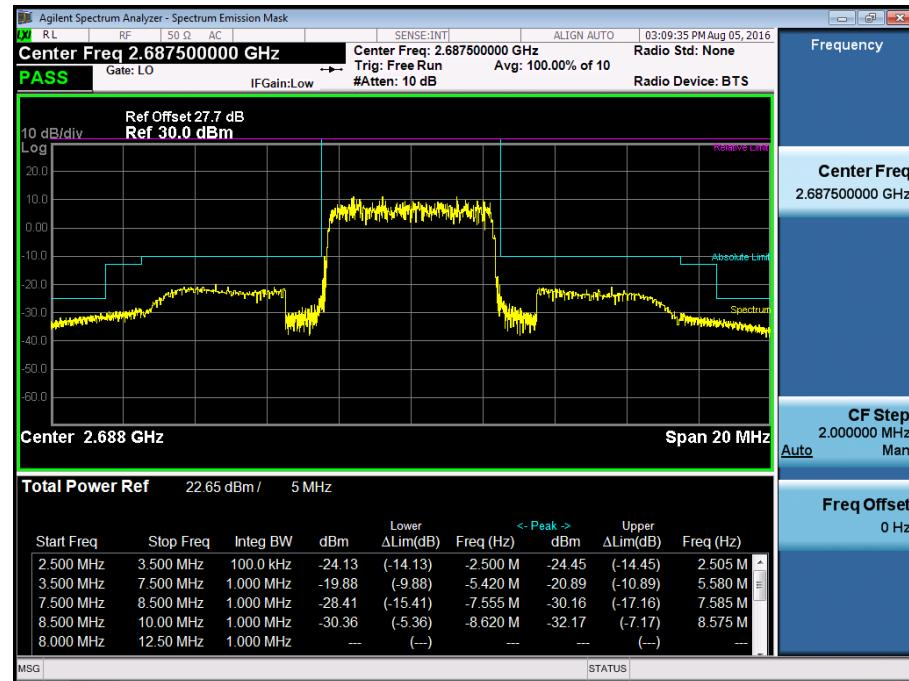
BAND 41. Low Channel Edge Plot (10 MHz Ch.39700 QPSK RB 50)
