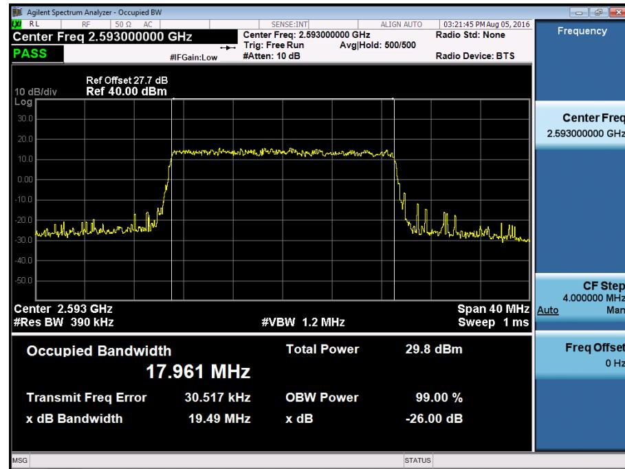
BAND 41. Low Channel Edge Plot (5 MHz Ch.39675 QPSK RB 25)
