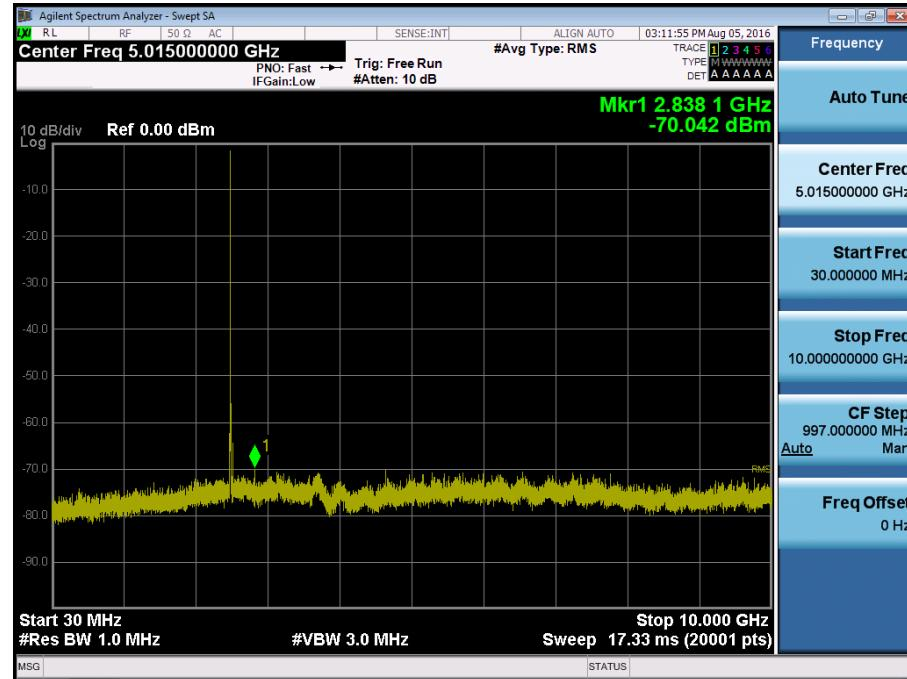
BAND 41. Conducted Spurious Plot 2 (10 MHz Ch. 39700 QPSK RB 1, Offset 0)
