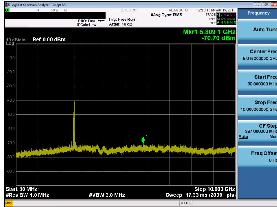
BAND 41. Conducted Spurious Plot 2 (20 MHz Ch. 41490 QPSK RB 1, Offset 0)
