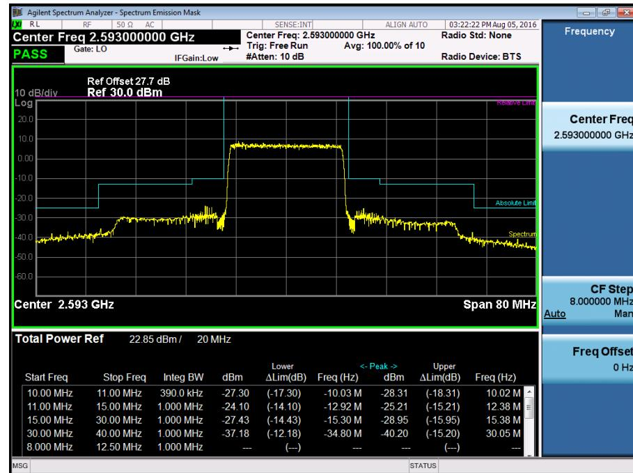
BAND 41. High Channel Edge Plot (20 MHz Ch.41490 QPSK RB 100)
