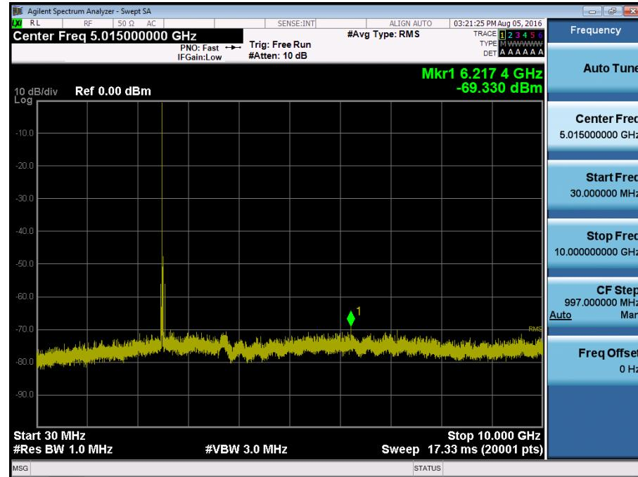
BAND 41. Conducted Spurious Plot 2 (20 MHz Ch. 39750 QPSK RB 1, Offset 0)
