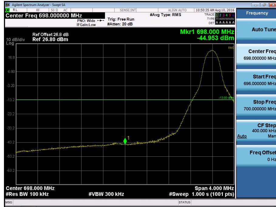
BAND 12 / 17. Lower Band Edge Plot (10M BW Ch.23060 QPSK\_RB50\_Offset 0)
