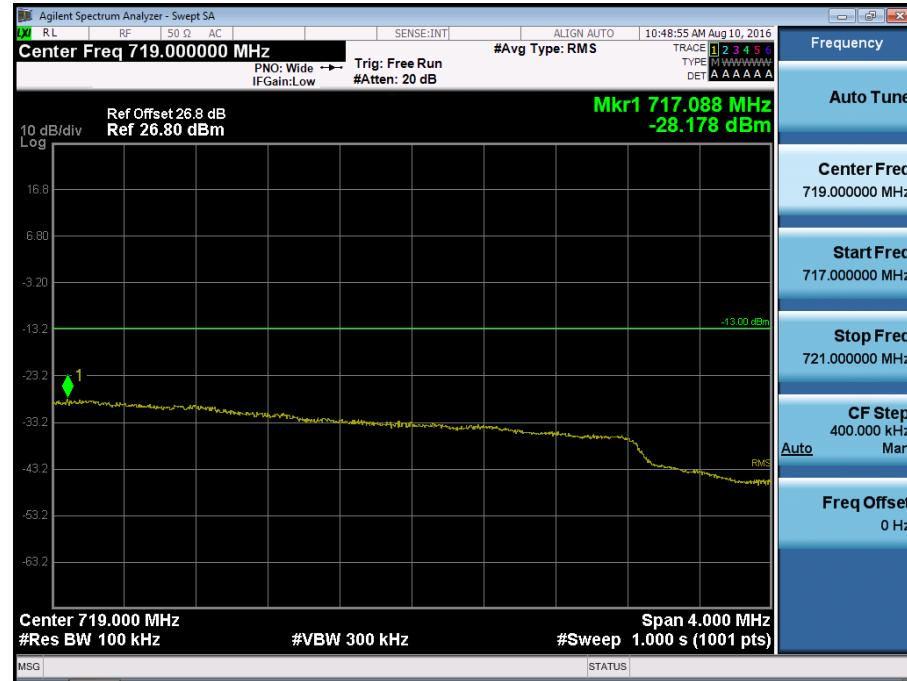
BAND 12 / 17. Upper Band Edge Plot (10M BW Ch.23130 QPSK\_RB1\_Offset 49)
