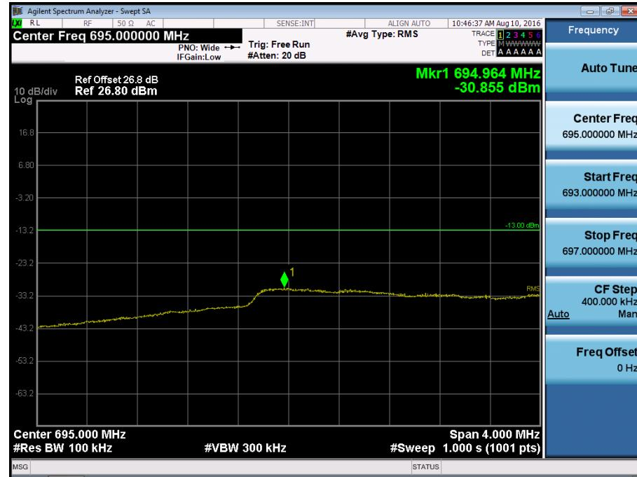
BAND 12 / 17. Lower Band Edge Plot (10M BW Ch.23060 QPSK\_RB1\_Offset 0)
