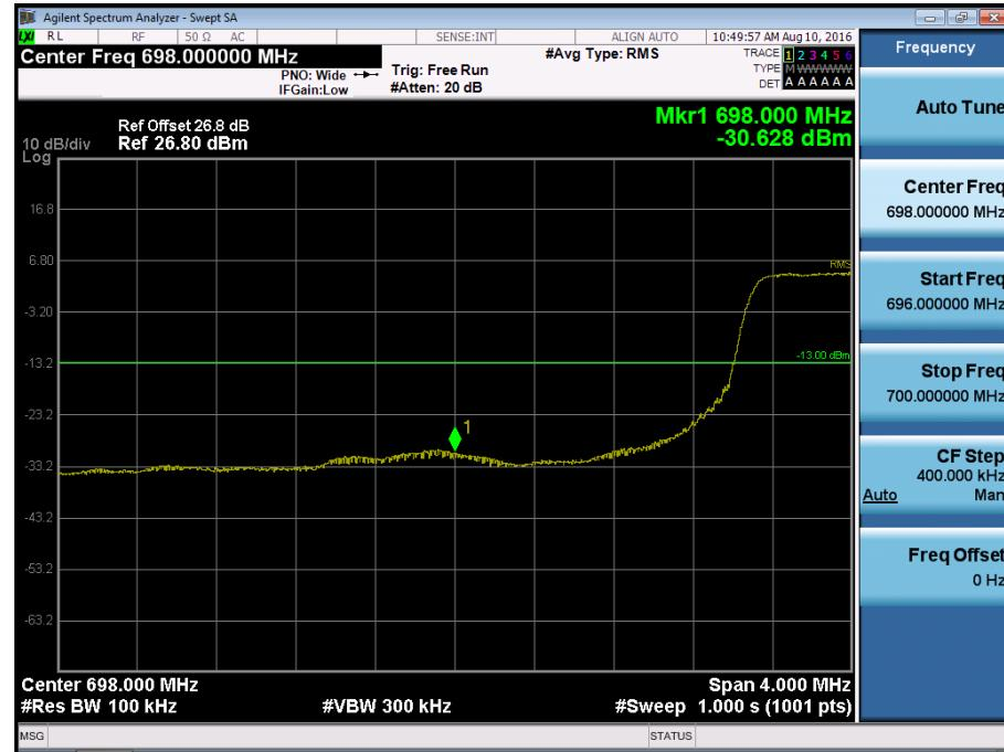
BAND 12 / 17. Lower Extended Band Edge Plot (10M BW Ch.23060 QPSK\_RB50\_0)
