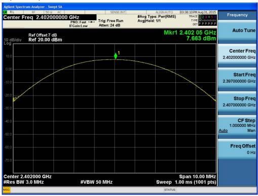
Test Plots (π/4DQPSK) Peak Power (Mid-CH)
