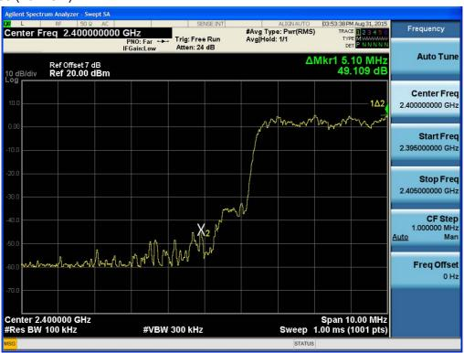
Test Plots with hopping ( $\pi$ /4DQPSK) Band Edges (High-CH)
