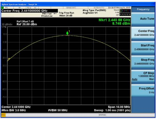
Test Plots (8DPSK) Peak Power (High-CH)
