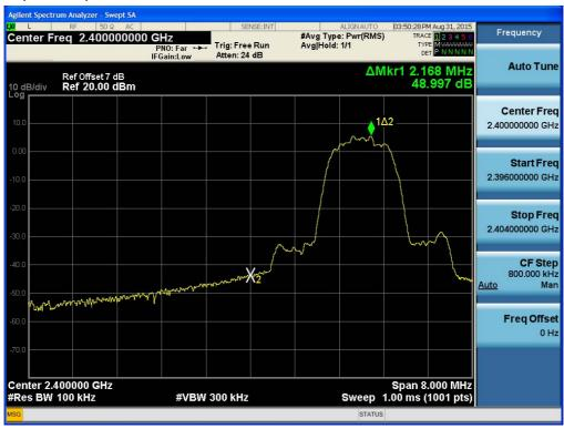
Test Plots without hopping (8DPSK) Band Edges (High-CH)
