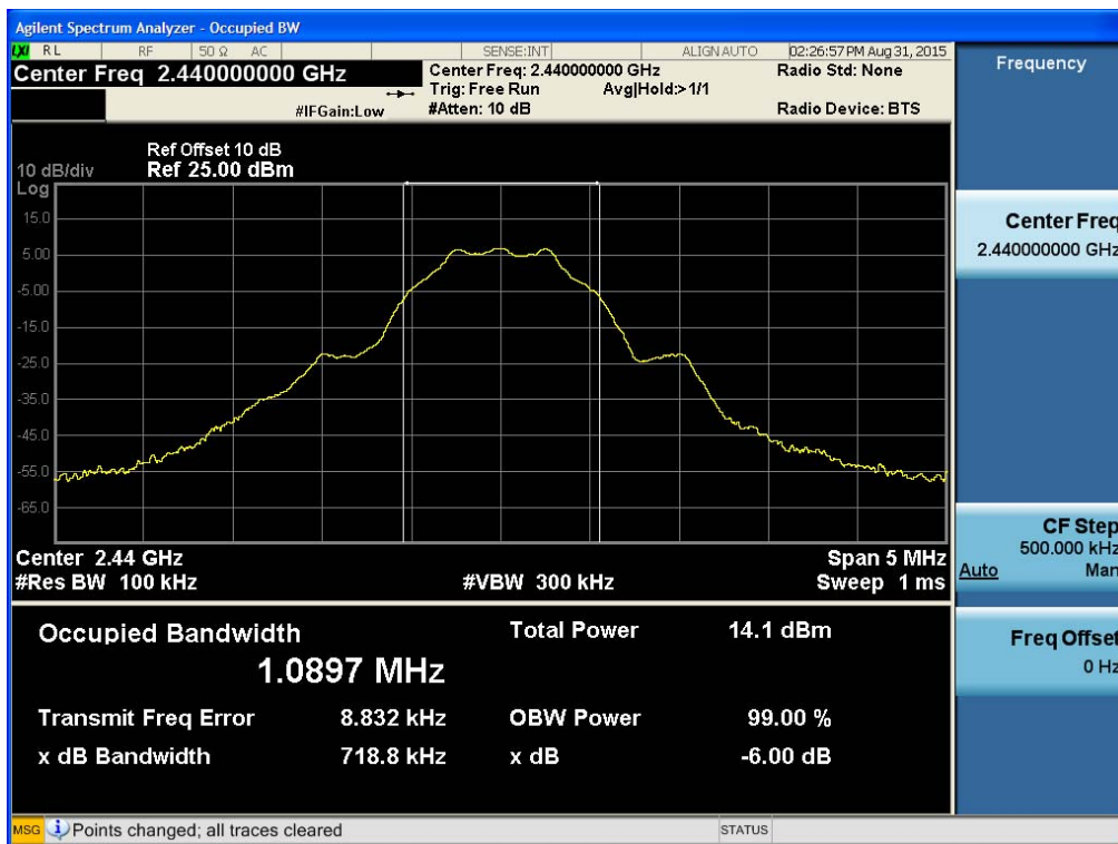
6dB Bandwidth plot (Mid-CH 19)
