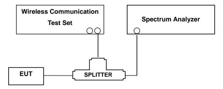
(Configuration of conducted Emission measurement)
