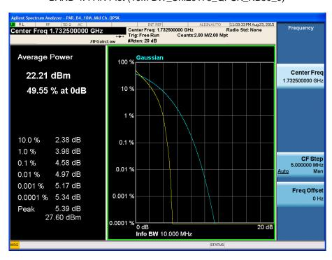
BAND 4. PAR Plot (10M BW\_Ch.20175\_16QAM\_RB50\_0)
