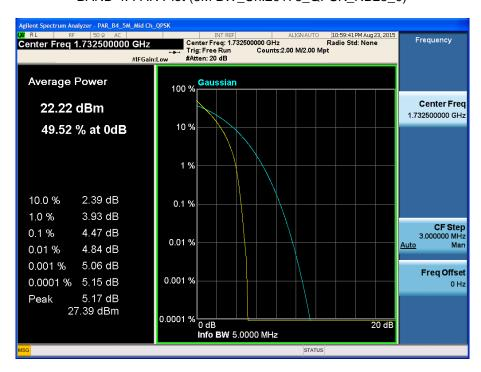
BAND 4. PAR Plot (5M BW\_Ch.20175\_16QAM\_RB25\_0)
