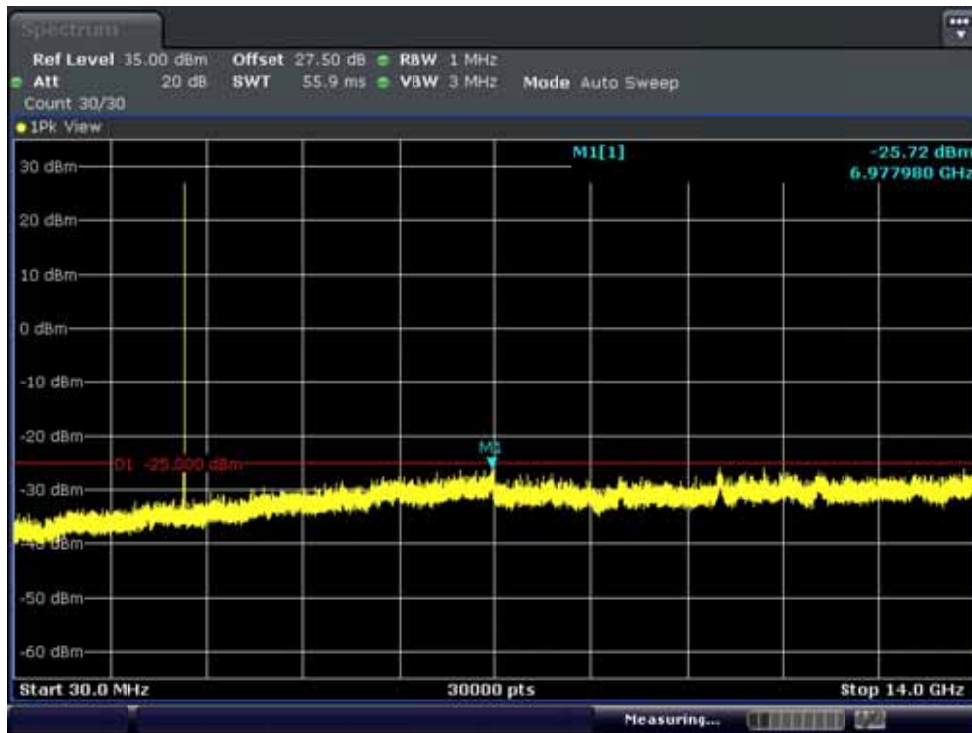
BAND7. Conducted Spurious Plot 1 (10MHz Ch.20800 QPSK RB 1, Offset 0)
