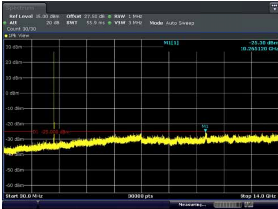
BAND7. Conducted Spurious Plot 1 (10MHz Ch.21400 QPSK RB 1, Offset 0)
