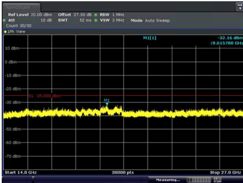
BAND7. Conducted Spurious Plot 2 (15MHz Ch.21100 QPSK RB 1, Offset 0)
