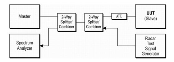
Figure 3-1. Conducted Test Setup for DFS
