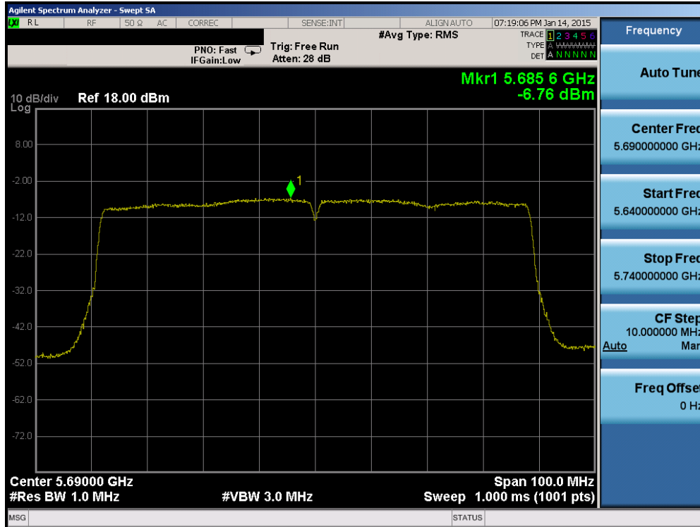
Plot 6-66. Power Spectral Density Plot (80MHz BW 802.11ac (UNII Band 2C) – Ch. 138)
