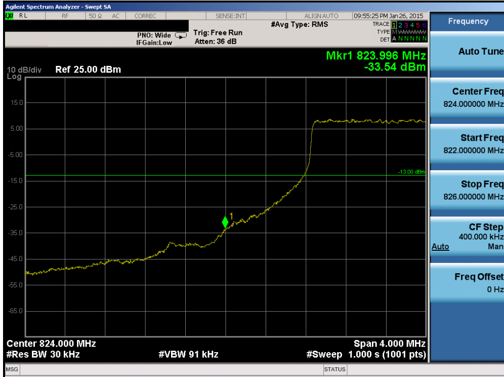
Plot 6-100. Lower Band Edge Plot (Band 5 – 3.0MHz QPSK – RB Size 15)
