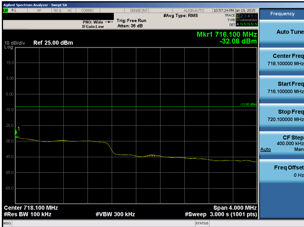
Plot 6-95. Upper Extended Band Edge Plot (Band 12 – 10.0MHz QPSK – RB Size 50)
