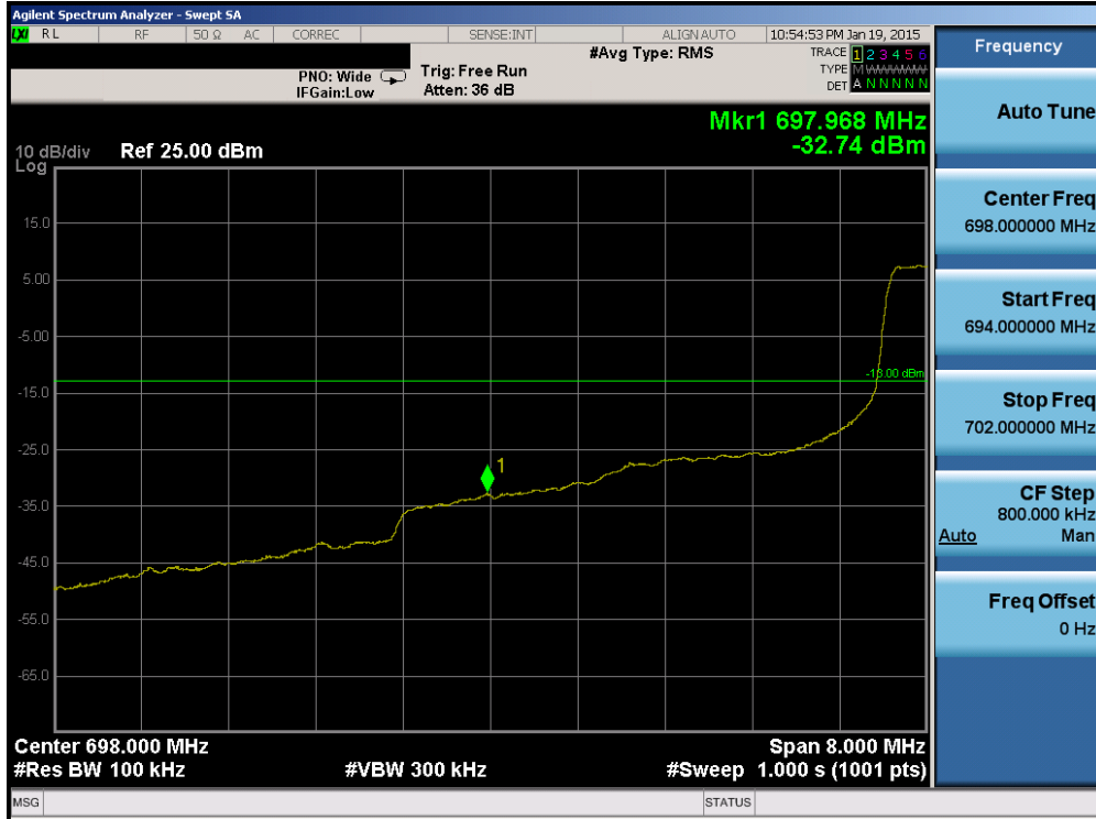
Plot 6-92. Lower Band Edge Plot (Band 12 – 10.0MHz QPSK – RB Size 50)
