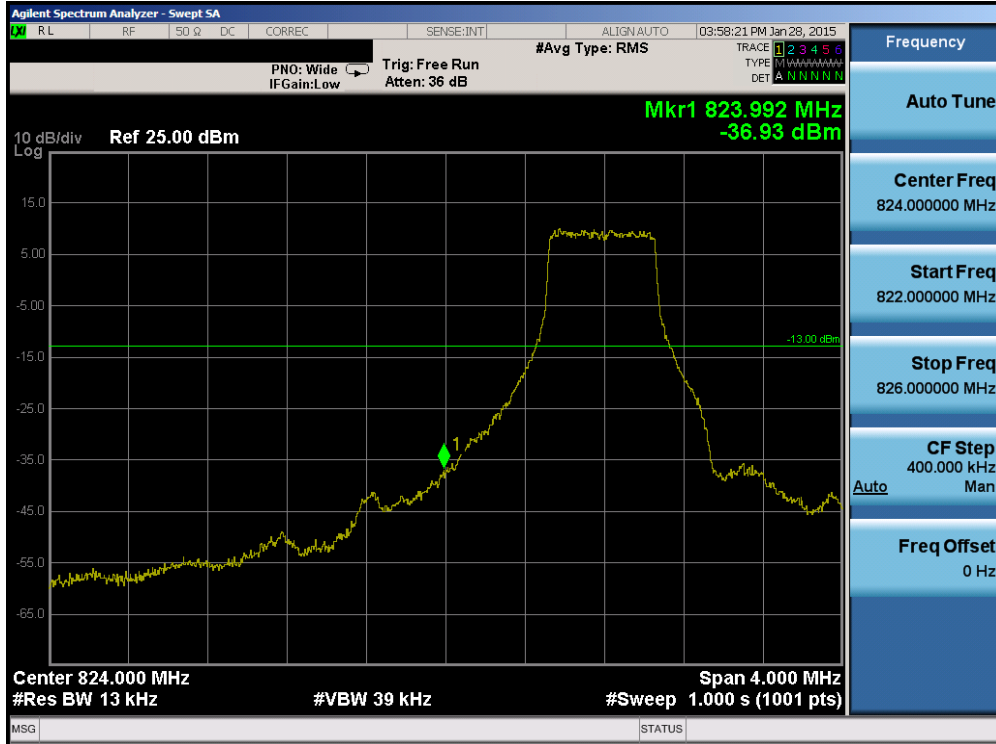
Plot 6-96. Lower Band Edge Plot (Band 5 – 1.4MHz QPSK – RB Size 6)
