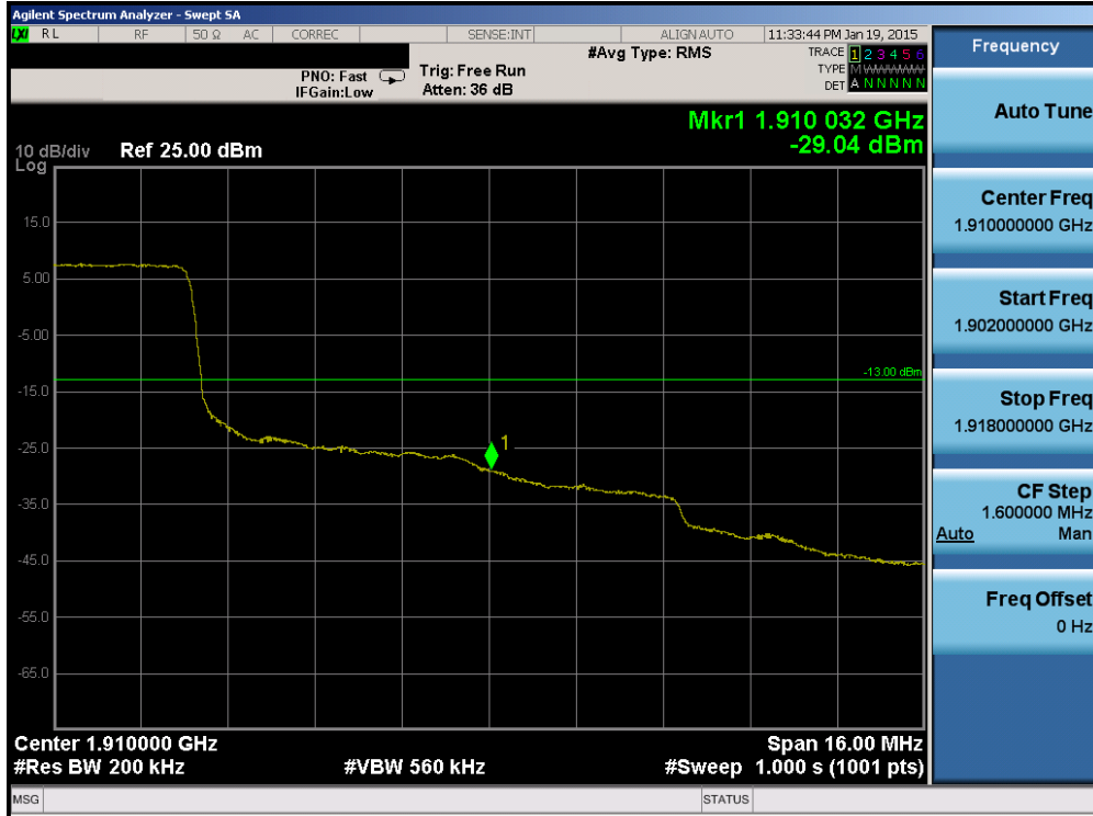
Plot 6-156. Upper Band Edge Plot (Band 2 – 20.0MHz QPSK – RB Size 100)
