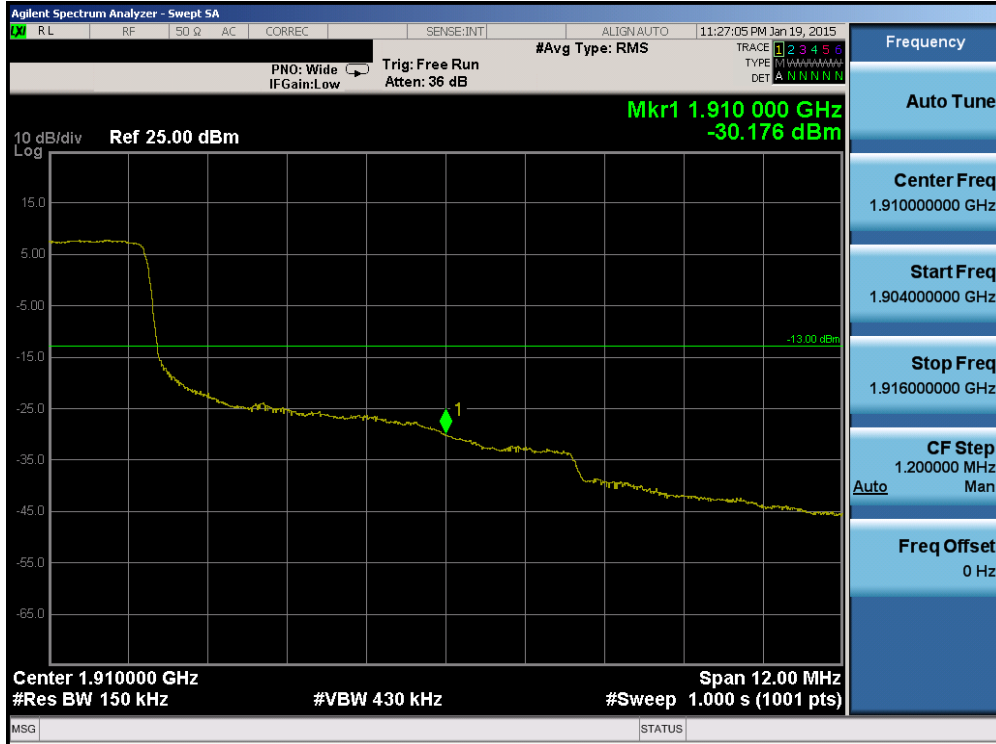
Plot 6-152. Upper Band Edge Plot (Band 2 – 15.0MHz QPSK – RB Size 75)
