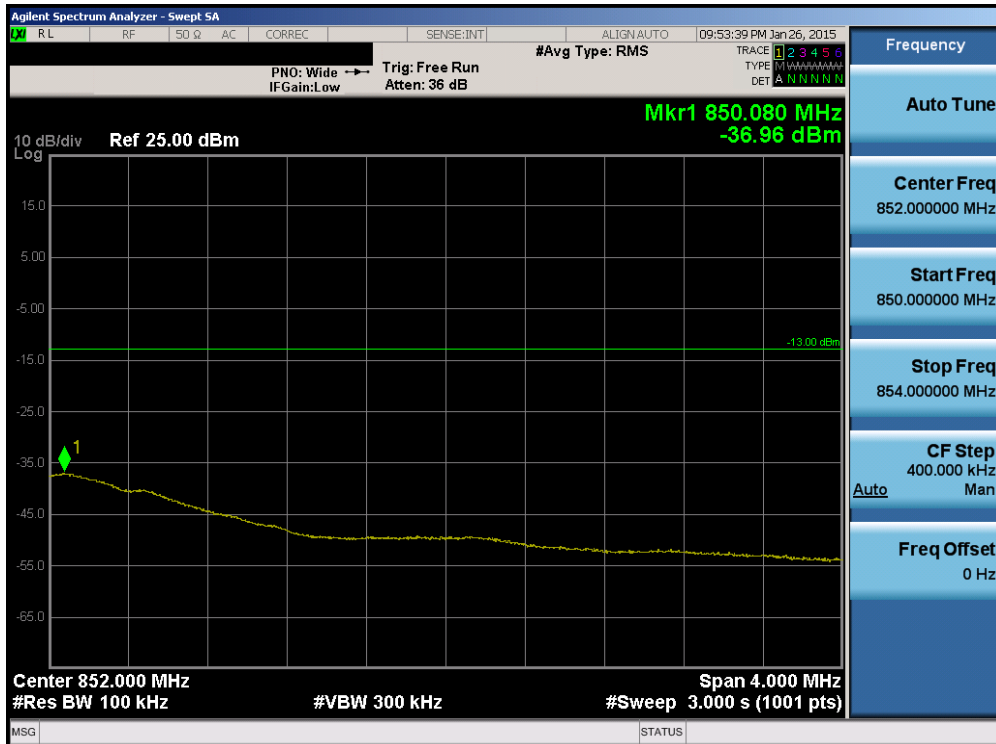
Plot 6-103. Upper Extended Band Edge Plot (Band 5 – Band 5 – 3.0MHz QPSK – RB Size 15)
