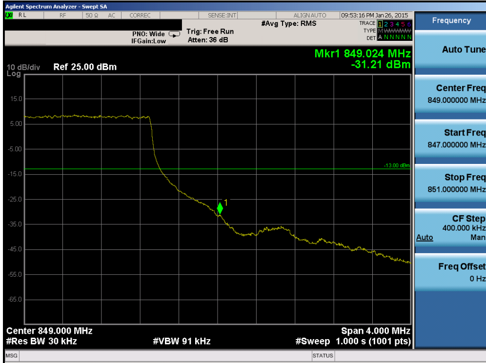
Plot 6-102. Upper Band Edge Plot (Band 5 – 3.0MHz QPSK – RB Size 15)
