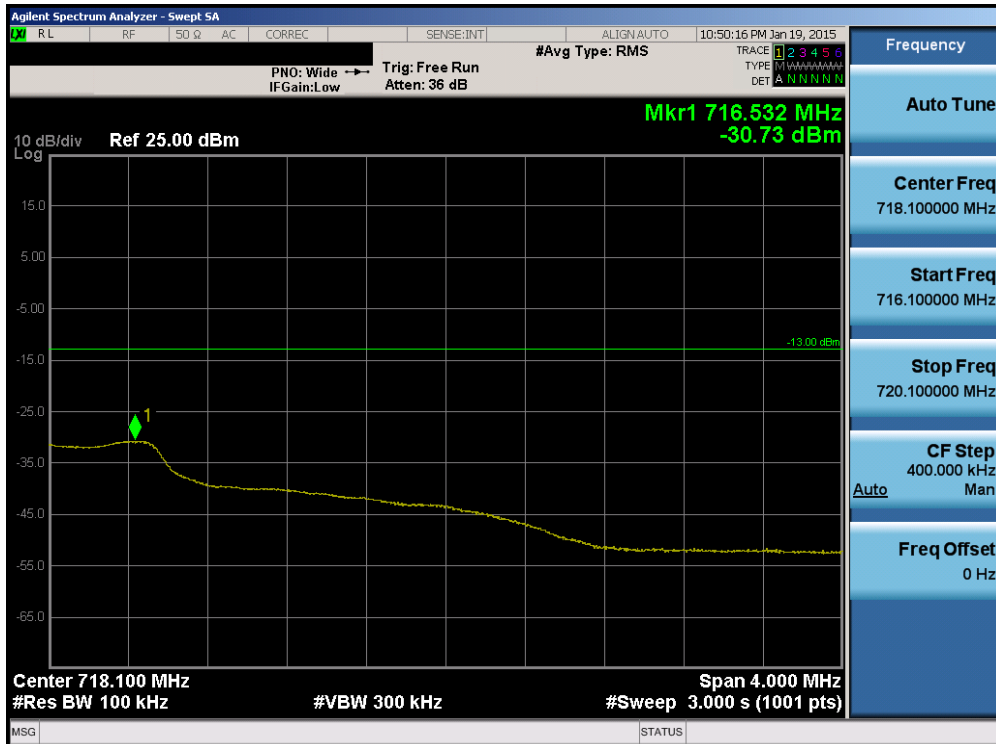
Plot 6-91. Upper Extended Band Edge Plot (Band 12 – 5.0MHz QPSK – RB Size 25)
