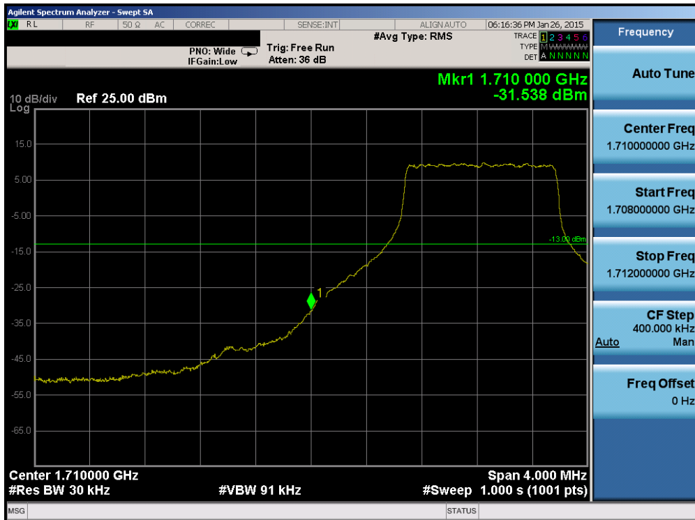
Plot 6-115. Lower Band Edge Plot (Band 4 – 3.0MHz QPSK – RB Size 15)
