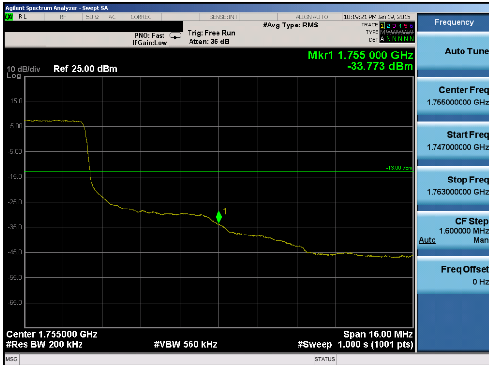
Plot 6-133. Upper Band Edge Plot (Band 4 – 20.0MHz QPSK – RB Size 100)
