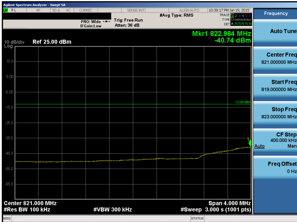
Plot 6-109. Lower Extended Band Edge Plot (Band 5 – 10.0MHz QPSK – RB Size 50)
