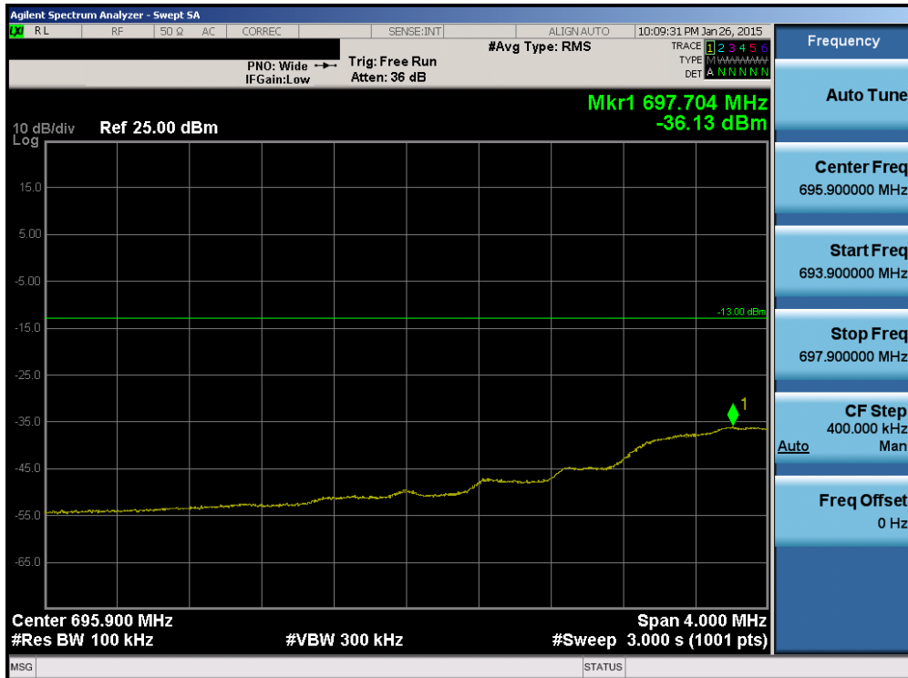
Plot 6-85. Lower Extended Band Edge Plot (Band 12 – 3.0MHz QPSK – RB Size 15)
