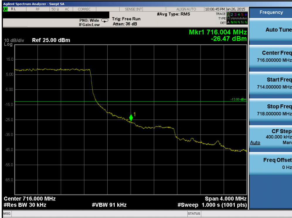
Plot 6-86. Upper Band Edge Plot (Band 12 – 3.0MHz QPSK – RB Size 15)
