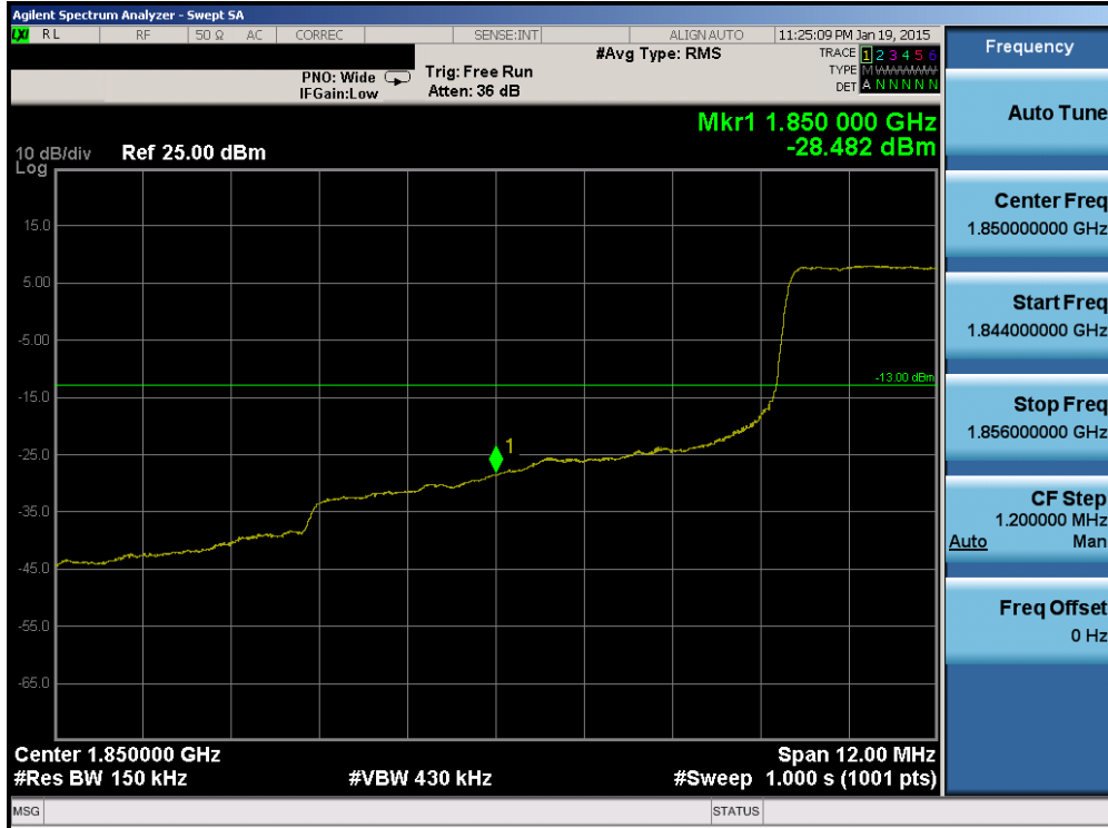
Plot 6-150. Lower Band Edge Plot (Band 2 – 15.0MHz QPSK – RB Size 75)
