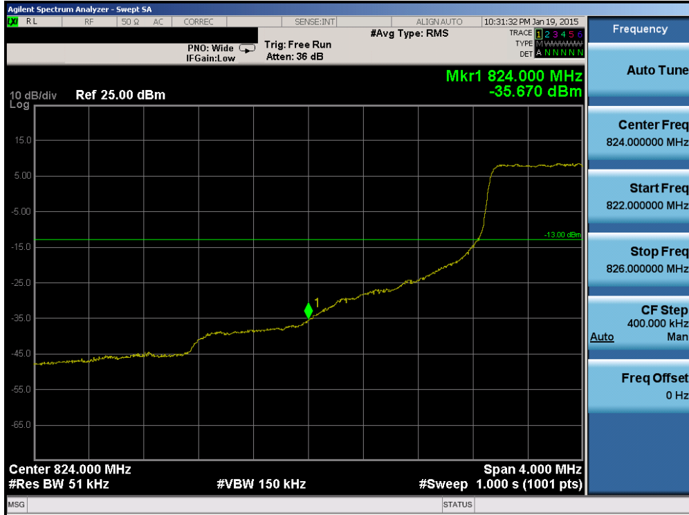
Plot 6-104. Lower Band Edge Plot (Band 5 – 5.0MHz QPSK – RB Size 25)
