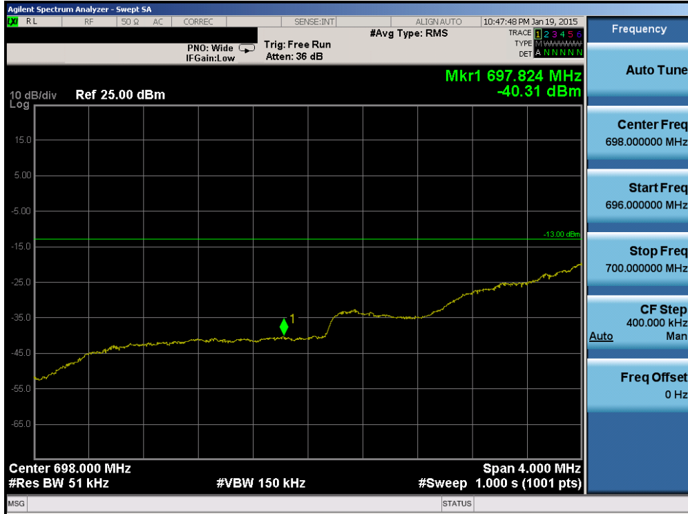
Plot 6-88. Lower Band Edge Plot (Band 12 – 5.0MHz QPSK – RB Size 25)
