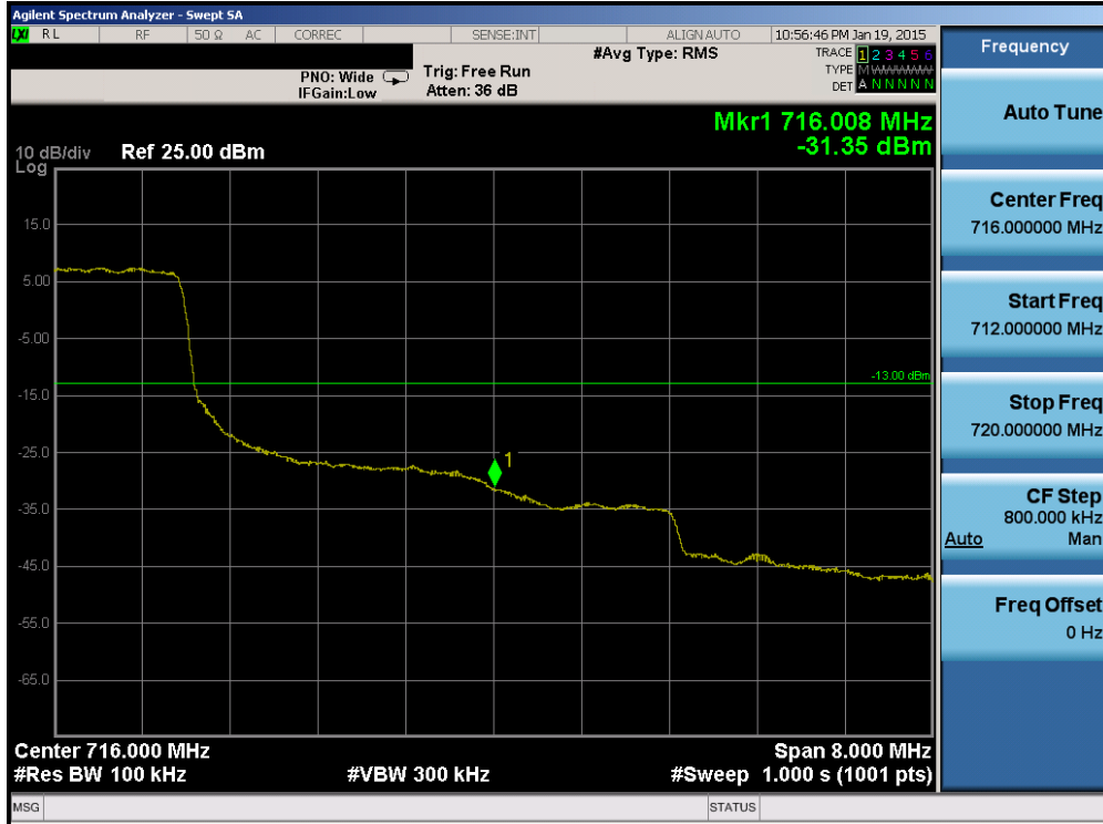
Plot 6-94. Upper Band Edge Plot (Band 12 – 10.0MHz QPSK – RB Size 50)
