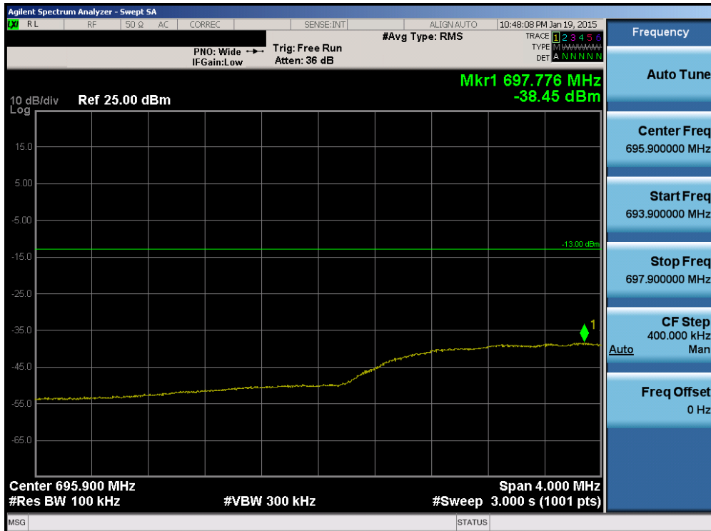
Plot 6-89. Lower Extended Band Edge Plot (Band 12 – 5.0MHz QPSK – RB Size 25)
