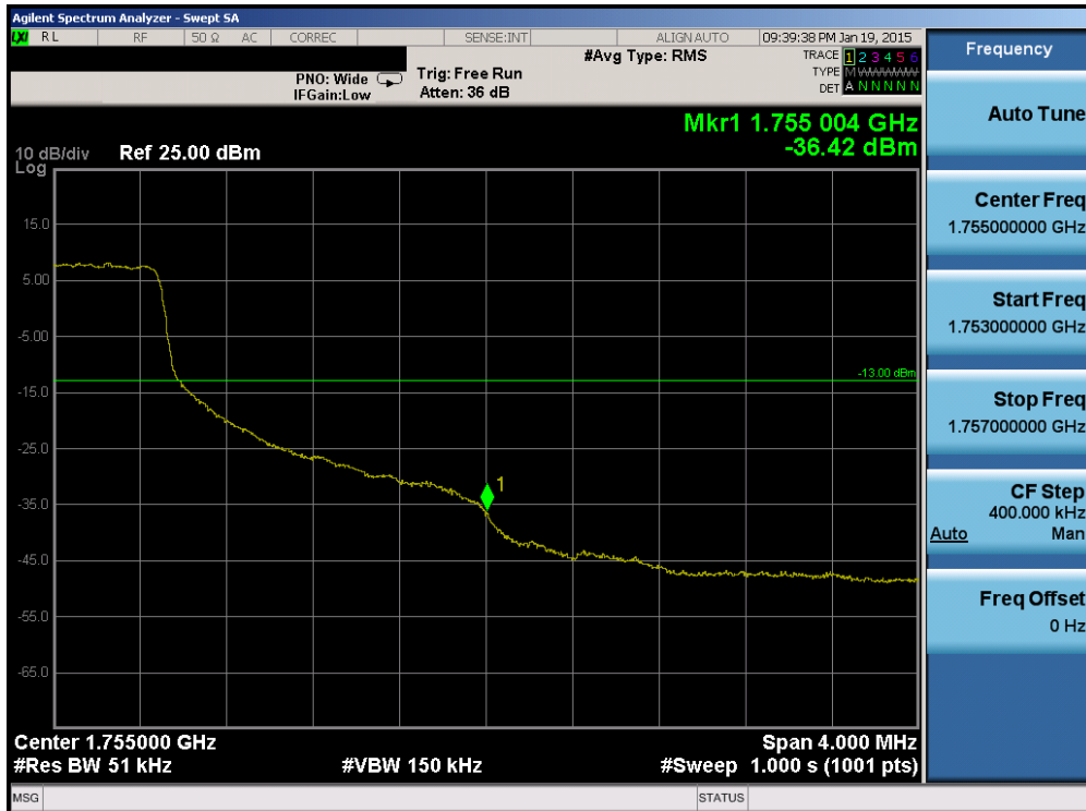
Plot 6-121. Upper Band Edge Plot (Band 4 – 5.0MHz QPSK – RB Size 25)
