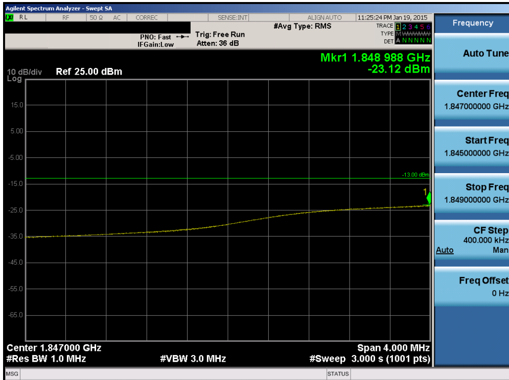
Plot 6-151. Lower Extended Band Edge Plot (Band 2 – 15.0MHz QPSK – RB Size 75)
