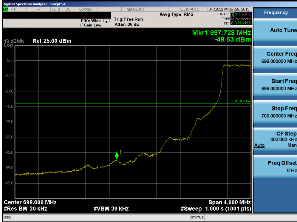
Plot 6-80. Lower Band Edge Plot (Band 12 – 1.4MHz QPSK – RB Size 6)
