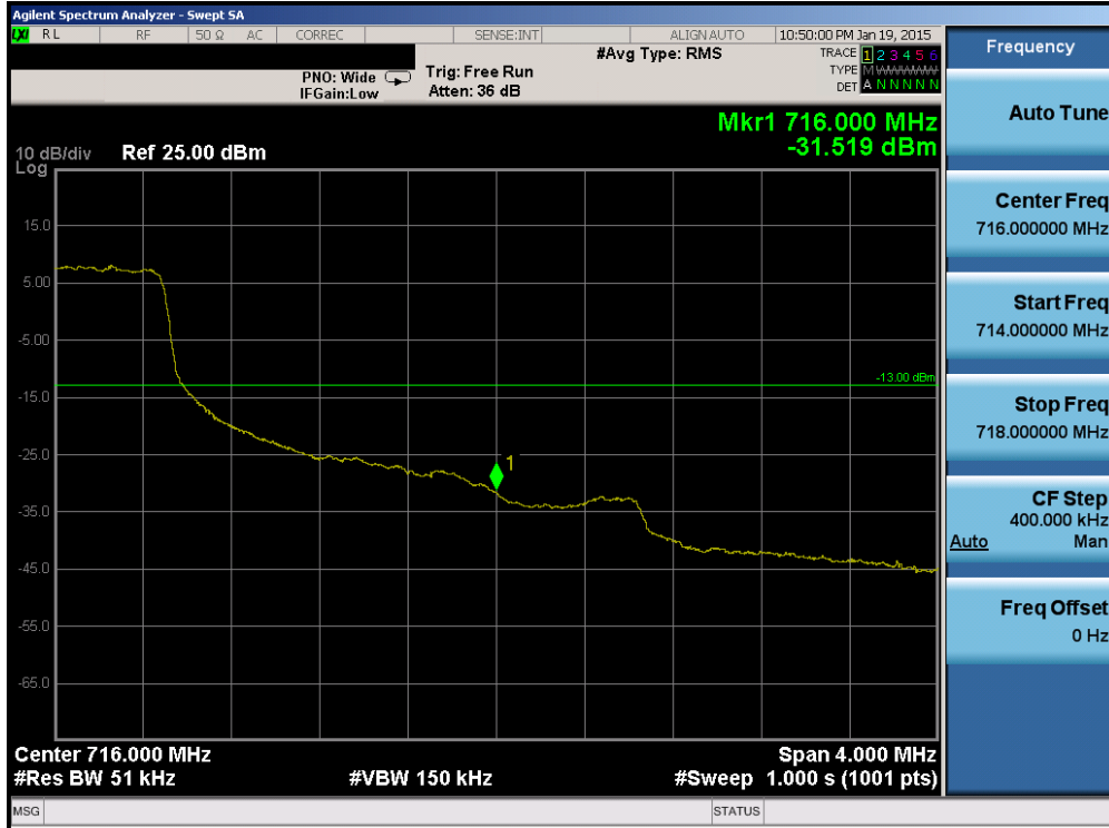
Plot 6-90. Upper Band Edge Plot (Band 12 – 5.0MHz QPSK – RB Size 25)
