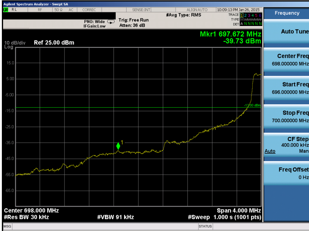
Plot 6-84. Lower Band Edge Plot (Band 12 – 3.0MHz QPSK – RB Size 15)
