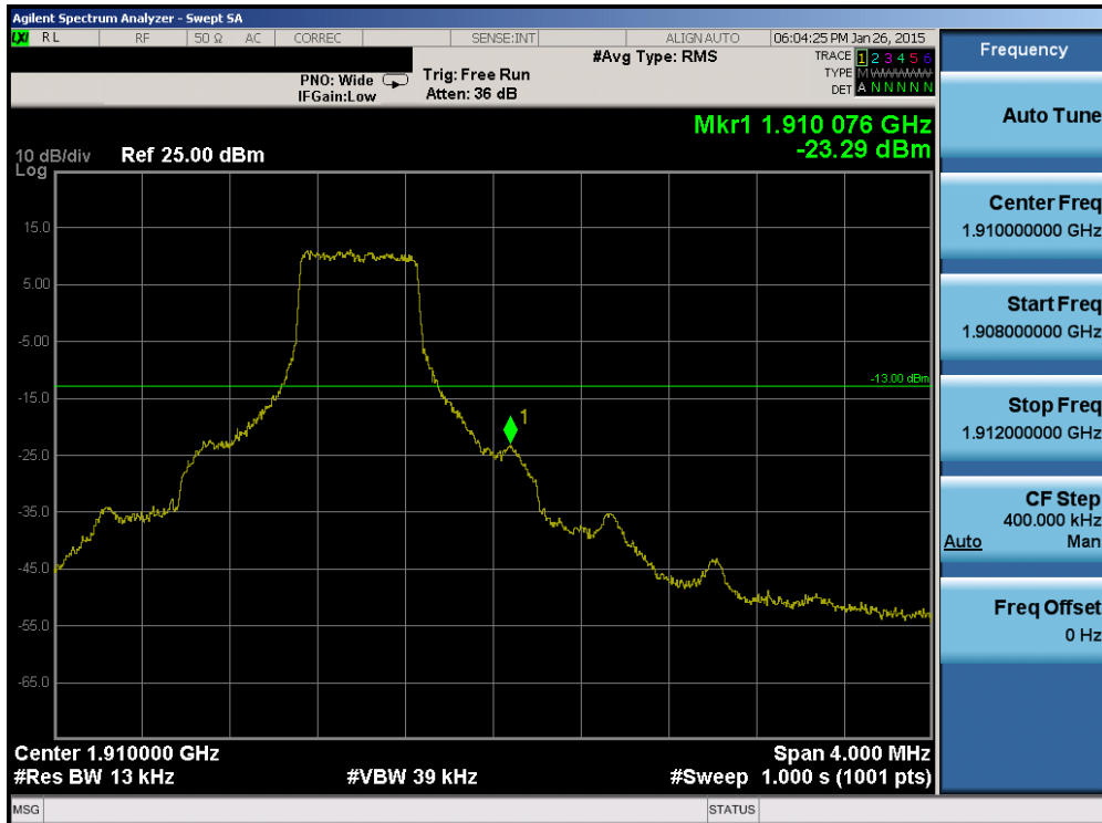
Plot 6-137. Upper Band Edge Plot (Band 2 – 1.4MHz QPSK – RB Size 6)
