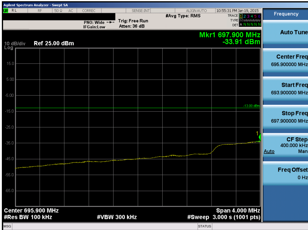
Plot 6-93. Lower Extended Band Edge Plot (Band 12 – 10.0MHz QPSK – RB Size 50)
