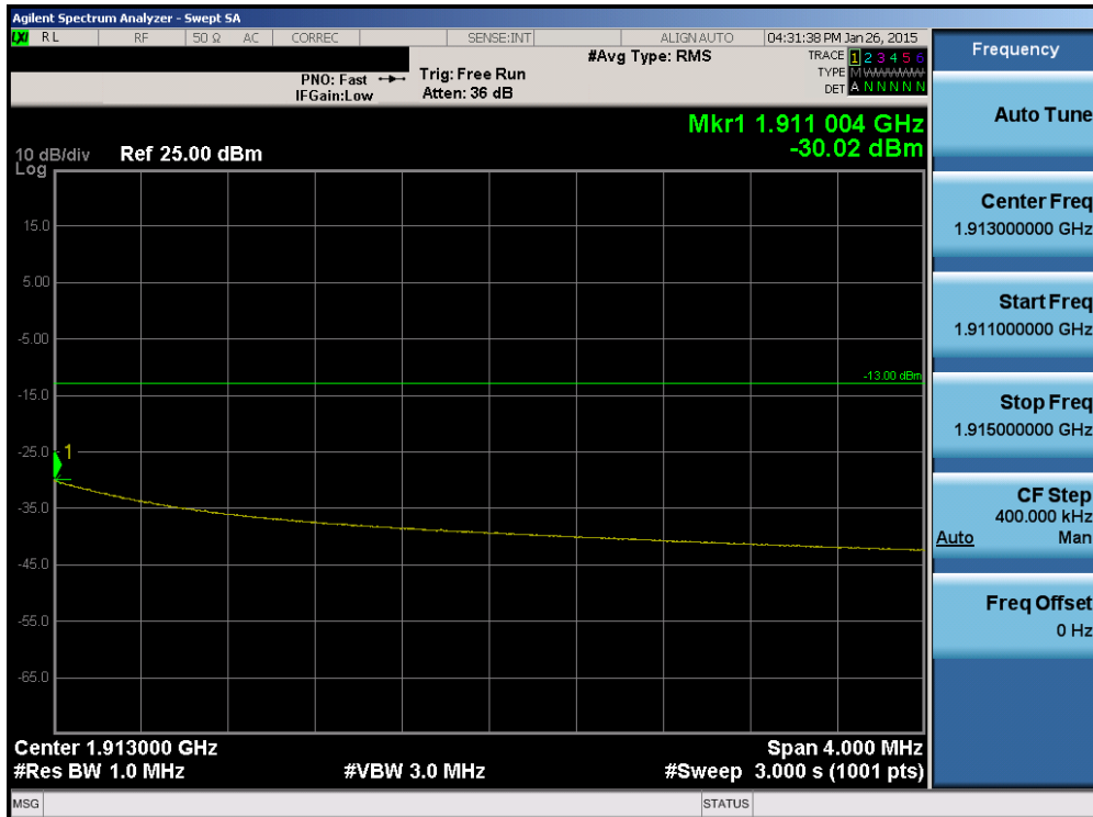
Plot 6-141. Upper Extended Band Edge Plot (Band 2 – 3.0MHz QPSK – RB Size 15)
