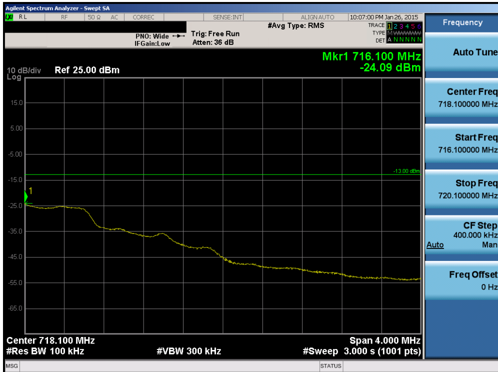
Plot 6-87. Upper Extended Band Edge Plot (Band 12 – 3.0MHz QPSK – RB Size 15)
