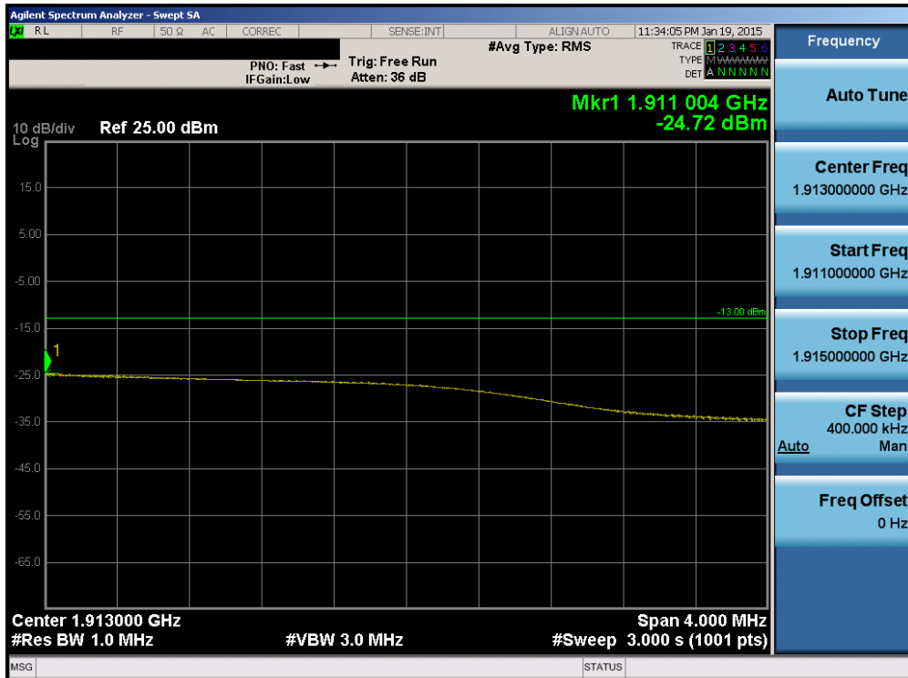
Plot 6-157. Upper Extended Band Edge Plot (Band 2 – 20.0MHz QPSK – RB Size 100)
